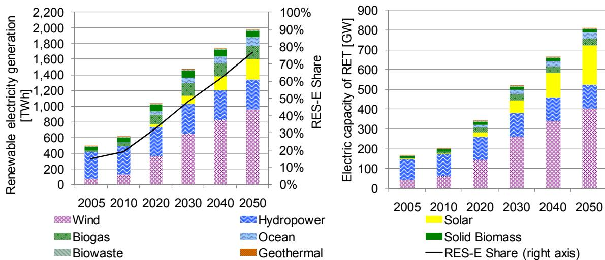
Figure 6-10 Renewable electricity generation, the share of renewables in gross electricity consumption and installed renewable capacity between 2005 and 2050 in the Policy\_FIT\_Static Scenario
