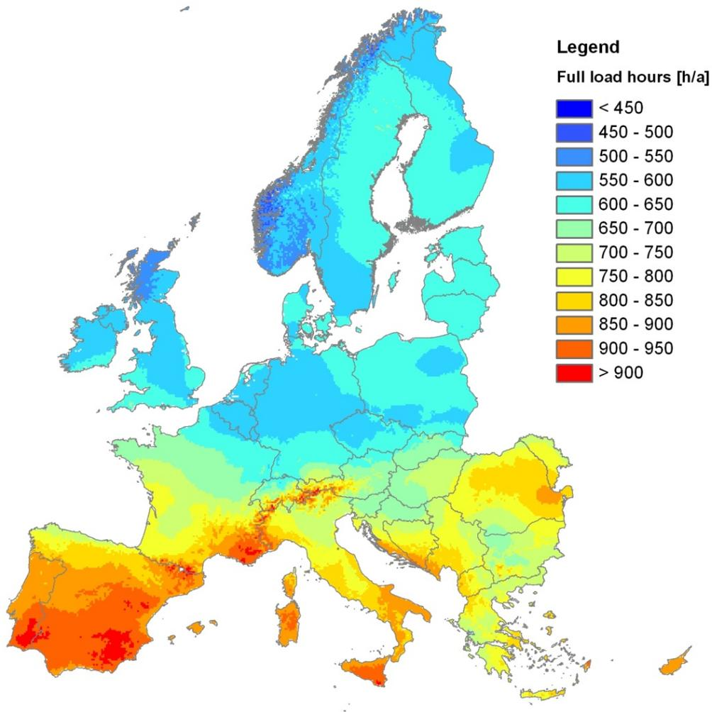
Figure 4-11 Annual full load hours of vertically inclined PV modules
