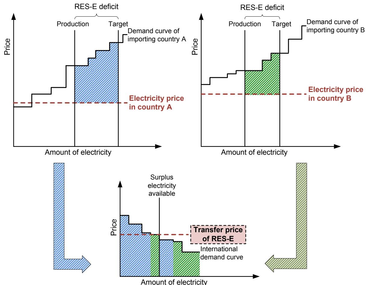
Figure 5-7 Schematic illustration of price determination mechanism in a buyer's market.
