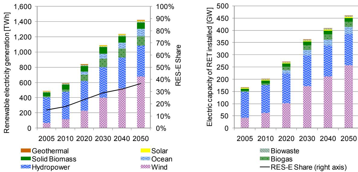
Figure 6-1 Renewable electricity generation, the share of renewables in gross electricity consumption and installed renewable capacity between 2005 and 2050 in the Reference Scenario
