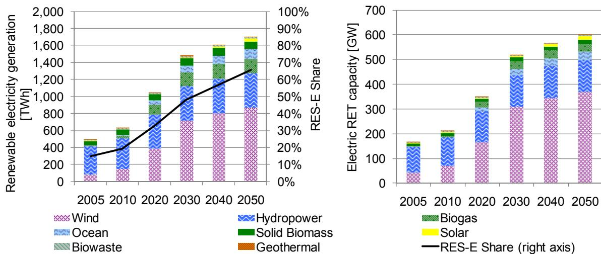
Figure 6-4 Renewable electricity generation, the share of renewables in gross electricity consumption and installed renewable capacity between 2005 and 2050 in the Policy\_Quota Scenario
