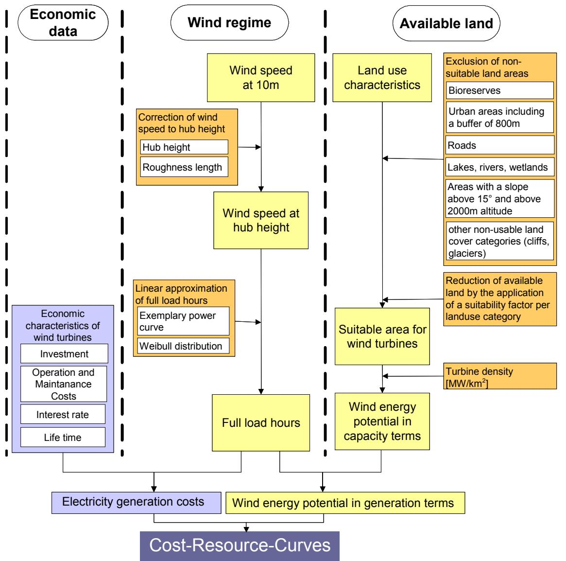
Figure 4-3 Scheme of applied approach for the determination of the cost-resource curves for onshore wind electricity
