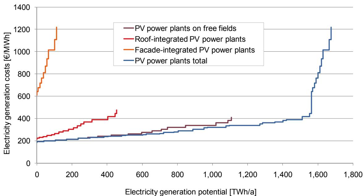
Figure 4-12 Derived cost-resource curves for solar PV technologies in the EU27 in 2009
