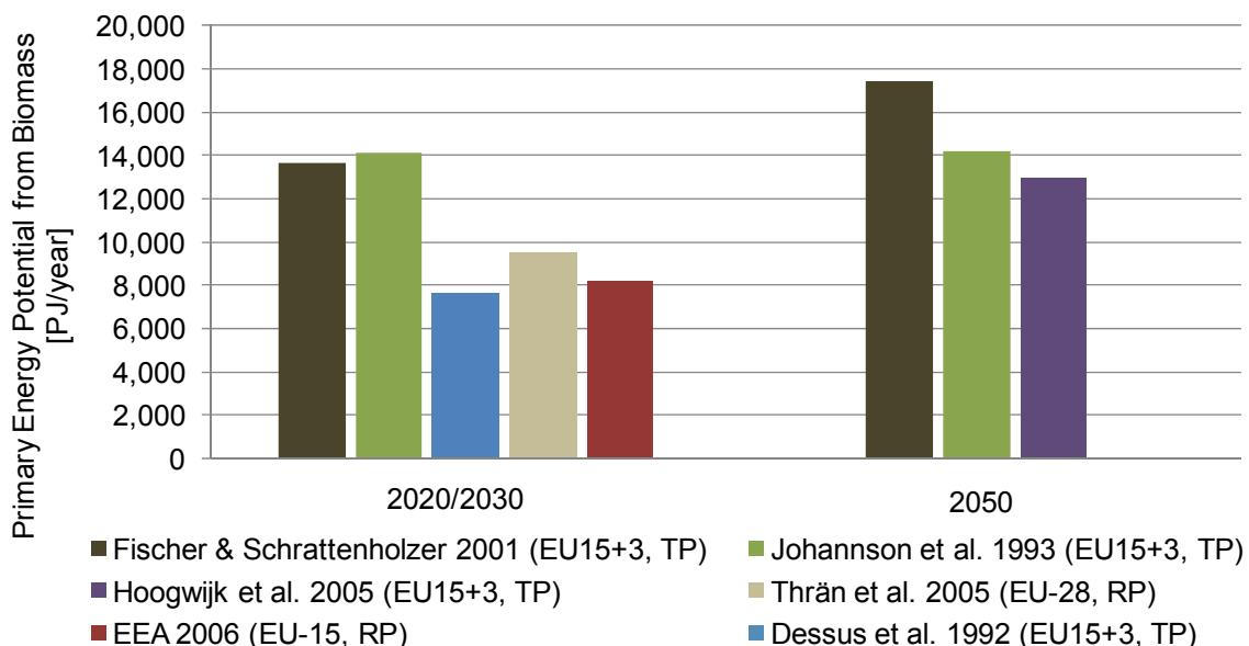
Figure 4-14 Comparison of the biomass primary energy potential in Europe. EU15+3 includes Norway, Switzerland and Turkey, TP means ‘Technical Potential’ and RP stands for ‘Realisable Potential’
