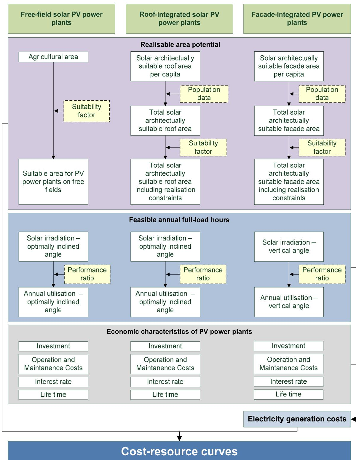
Figure 4-9 Scheme of applied approach for the determination of the cost-resource curves for electricity generation from solar PV power plants
