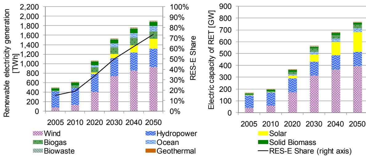
Figure 6-7 Renewable electricity generation, the share of renewables in gross electricity consumption and installed renewable capacity between 2005 and 2050 in the Policy\_FIT\_Dynamic Scenario
