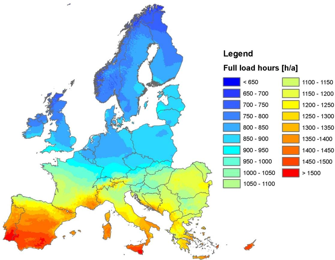
Figure 4-10 Annual full load hours of optimally inclined PV modules
