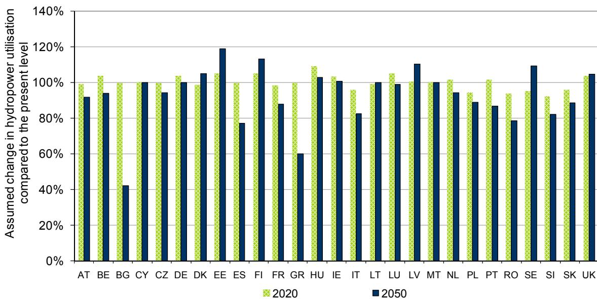
Figure 5-8 Assumed change in hydropower utilisation compared to the base year 2005
