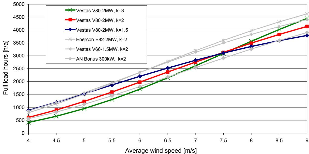
Figure 4-4 Approximation of the relation between full load hours and average wind speeds based on power curves of existing wind turbines
