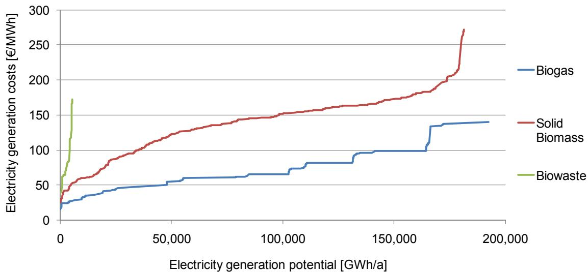
Figure 4-16 Derived cost-resource curves for biomass conversion technologies in the EU27 for 2009
