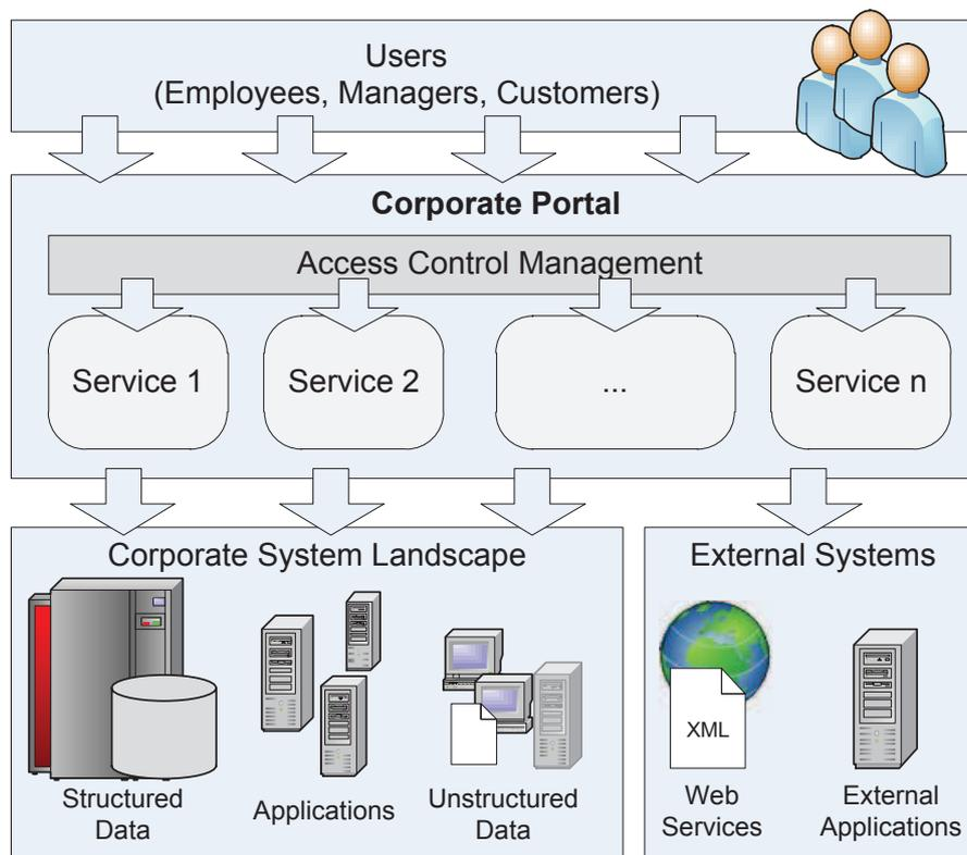
**Figure 1.3.:** Corporate portal architecture with interfaces to various sources and access control component.
