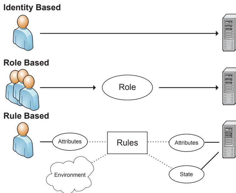
Figure 1.4.: Access control model types.
