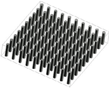
Figure 2.6: Sketch of a 1-3 piezoelectric fibre composite material. Fibre spacing, fibre diameters, and their variations are defined by the applied technology [Sch08].
