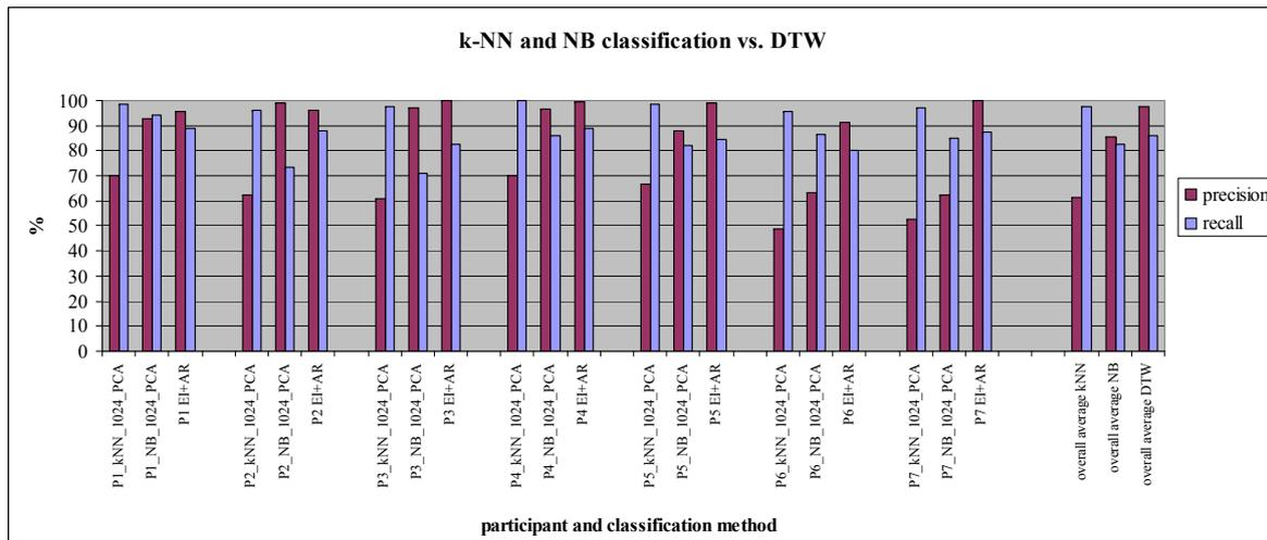
**Figure 6.15:** Comparison of the classification performance of online DTW with sliding window classification methods. Sliding window classification has been performed with a Naive Bayes (NB) classifier and a k-nearest neighbor classifier (kNN). Results are averaged over all classes.
