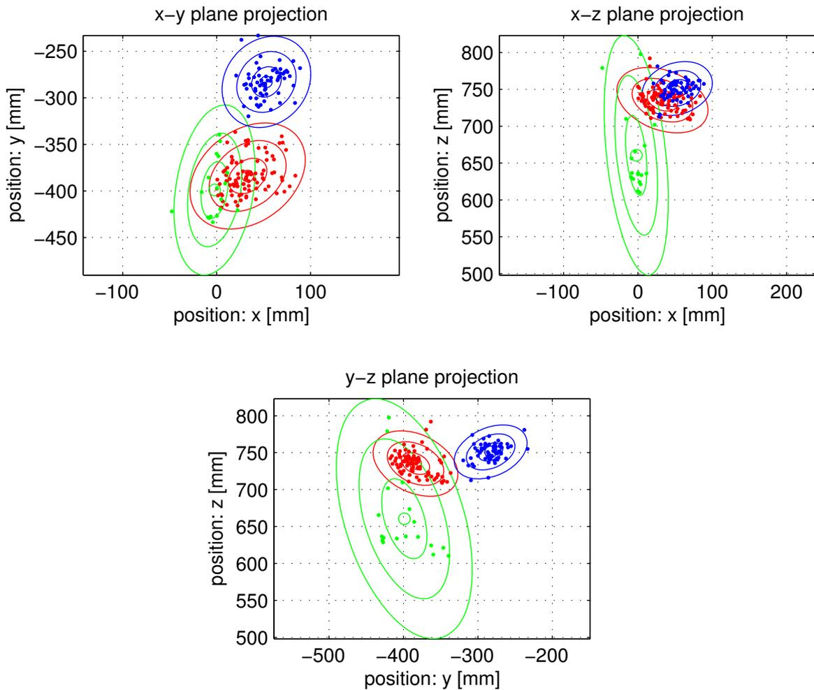
**Figure 4.5:** 2-dimensional projections of the position measurements of figure 4.4 onto the  $x-y$ ,  $x-z$  and  $y-z$  planes. The  $1\sigma$ ,  $2\sigma$ ,  $3\sigma$  ellipses enclose possible confidence areas.
