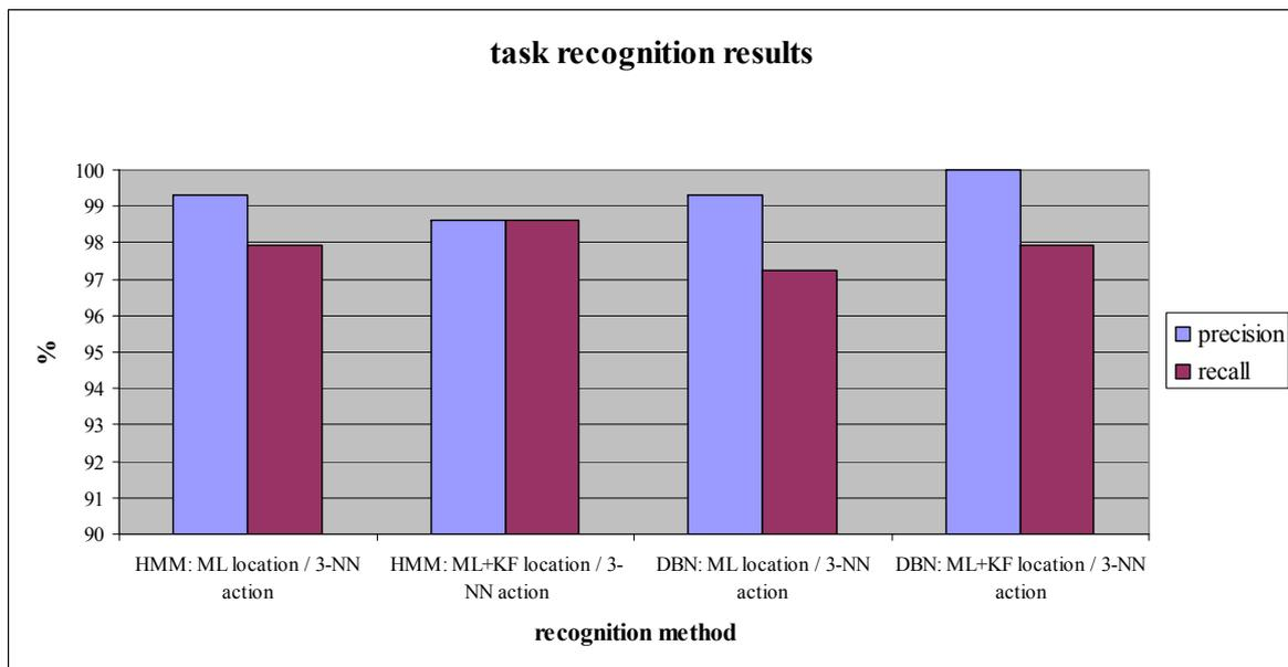
**Figure 5.9:** Comparison of online task recognition results based on sequences containing all tasks. All tests are based on the detections from maximum likelihood location classification (with and without KF) and 3-NN action classification. For the HMM experiments location and action classification results have been fused by majority voting.
