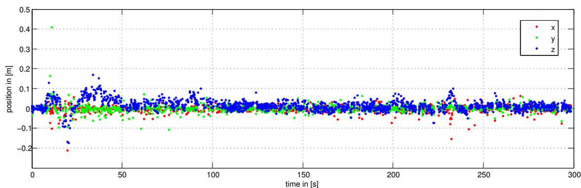
**Figure 3.13:** EKF result for a real data test sequence: Position deviation of estimations with the 15-state model to VT system measurements at the end of each outage.
