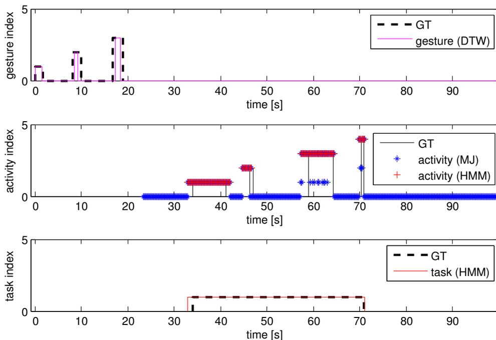
**Figure 7.6:** Recognition results of the PC assembly and gesture recognition experiment part 1. The results have been recorded during the execution of gestures 1–3 and task number 1.
