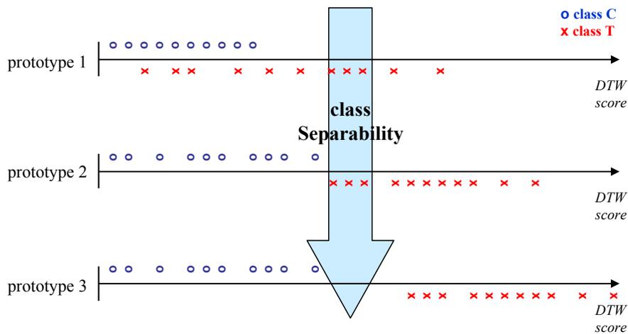
**Figure 6.3:** Distance distributions of DTW score values. The distance distributions of the prototypes to templates of classes *C* and *T* differ depending on the prototype. Prototype 3 achieves the best separation between the distributions.
