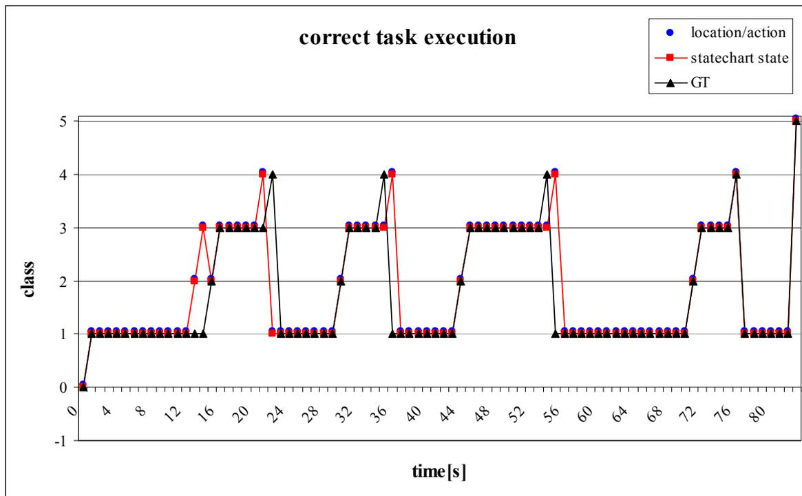
**Figure 7.4:** Recognition results of a correctly executed spot welding task. The plot shows detected actions and locations such as the resulting statechart states (0 = gun in storage, 1 = gun moving, 2 = gun at spot position, 3 = gun stable at spot position, 4 = welding of spot, 5 = returned to storage, -1 = task error). The GT refers to the statechart state and has been recorded manually.
