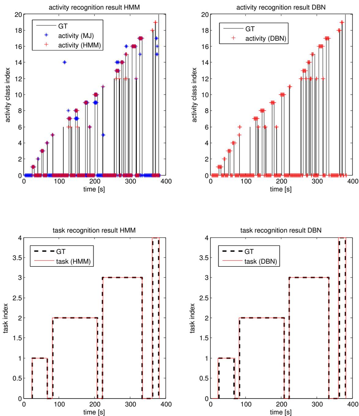
**Figure 5.8:** Result example for activity (top) and task (bottom) recognition with the HMM (left) and the DBN (right). The processed sequence contains all tasks of the PC scenario.
