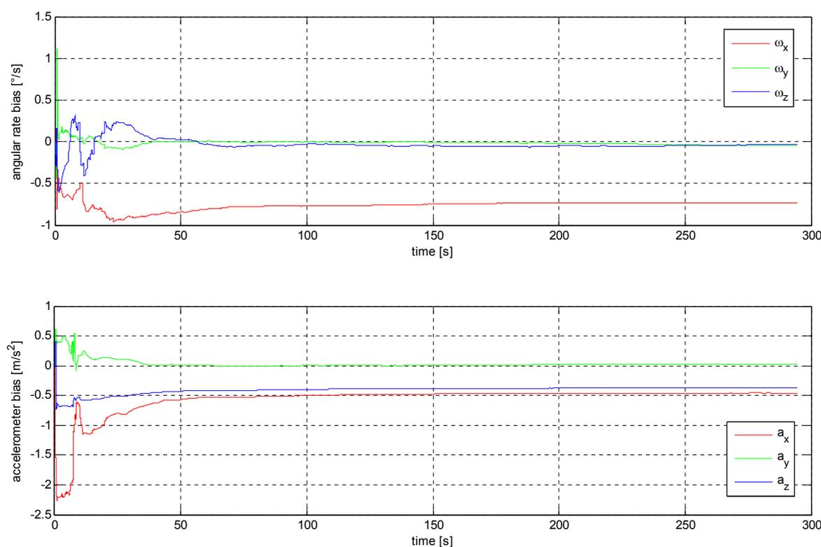
**Figure 3.15:** Bias estimations of the 15-state EKF model for a sequence of the real dataset. After an initialization time of about a minute, the filter provides a stable result for bias estimations.
