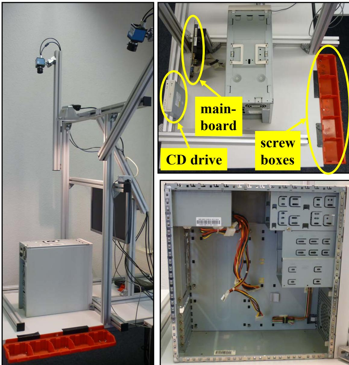
**Figure 4.6:** PC scenario: Left: Laboratory workplace environment overview. Right (top): PC case position and storage places of the mainboard, the CD drive and the screws. Right (bottom): Empty PC case
