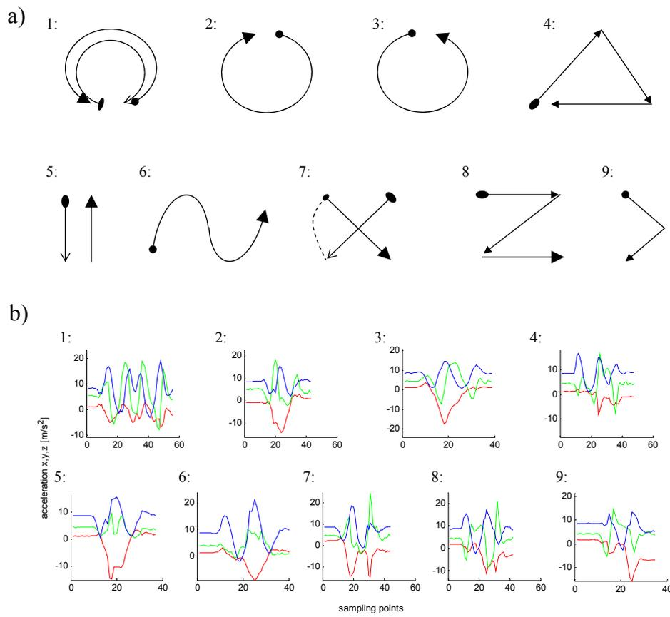
**Figure 6.7:** Gestures utilized in DTW tests: a) Gesture descriptions (arm movements). b) Accelerometer signals of the respective gestures.
