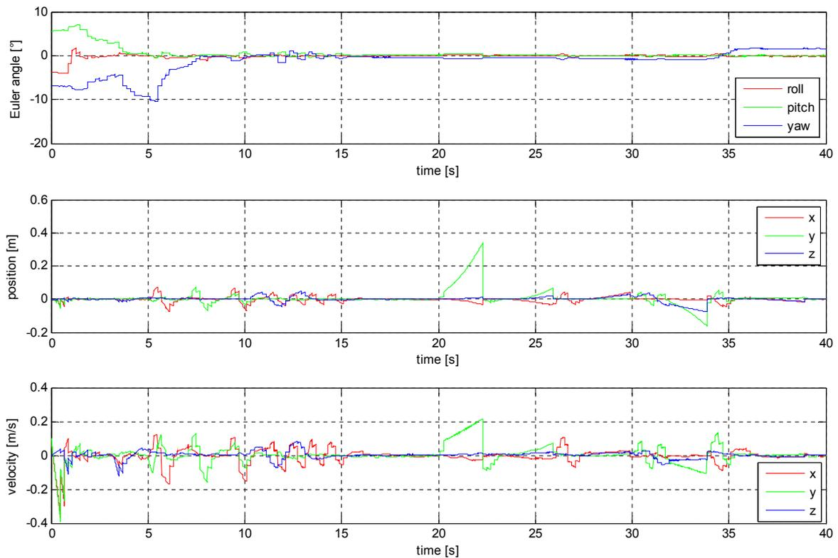
**Figure 3.9:** Estimation errors of the 15-state EKF model after application to a sequence of simulated data with outages and a synchronization error between IMU and VT data of 100ms: Attitude, position and velocity.
