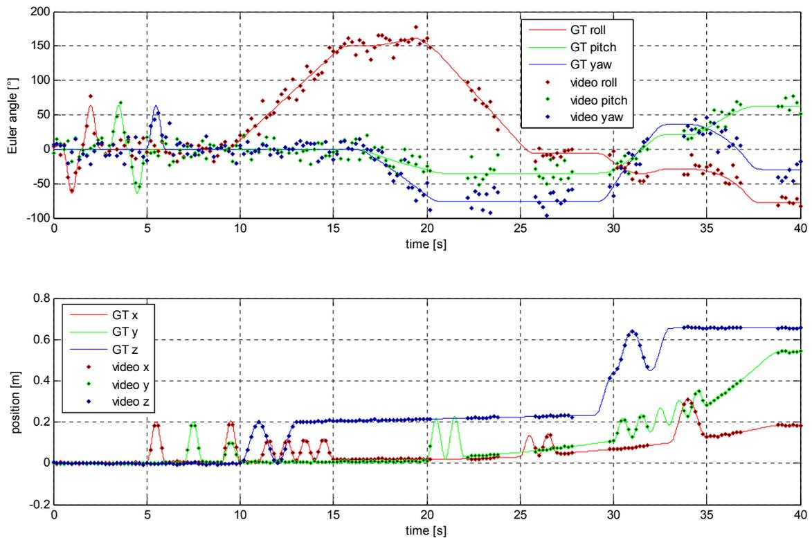
**Figure 3.5:** VT measurements (attitudes and positions) of a simulated test run with outages. Ground truth data is represented by lines and sampling points of simulated VT measurements by dots.
