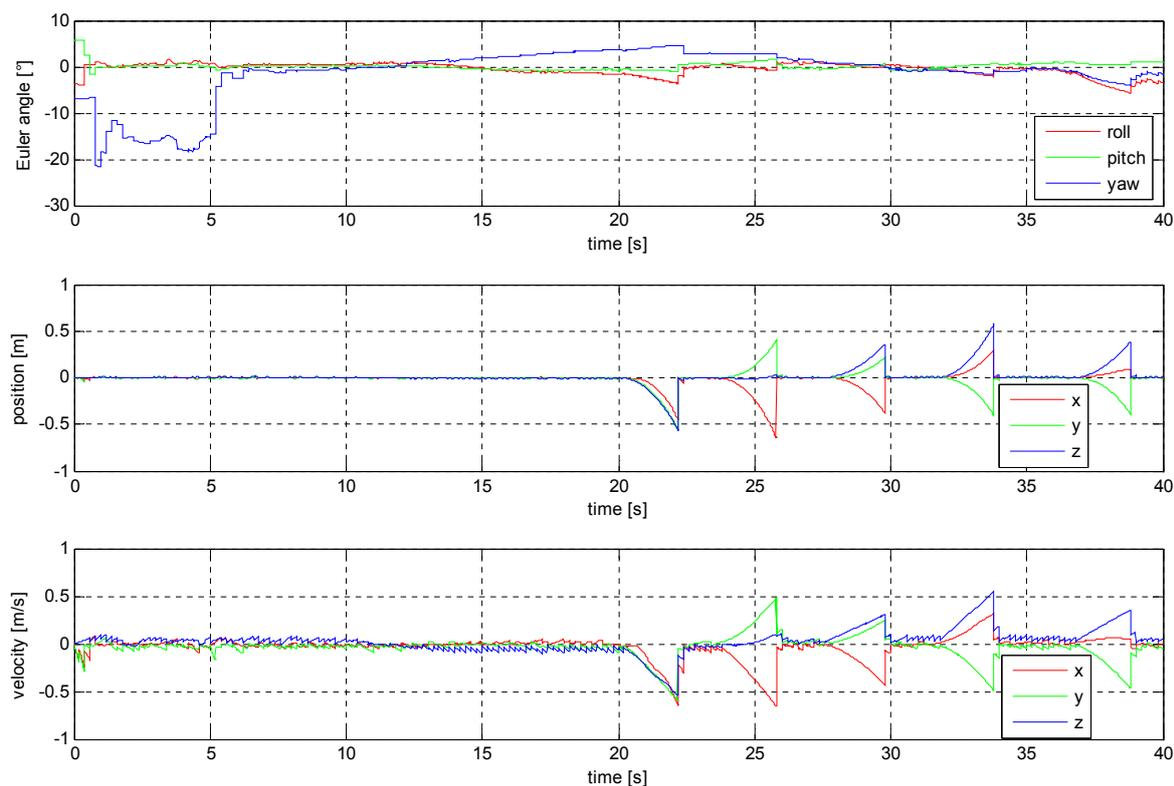
**Figure 3.6:** Estimation errors of the 9-state EKF model after application to a sequence of simulated data with outages.
