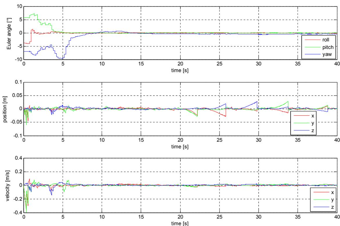
**Figure 3.7:** Estimation errors of the 15-state EKF model after application to a sequence of simulated data with outages: Attitude, position and velocity.
