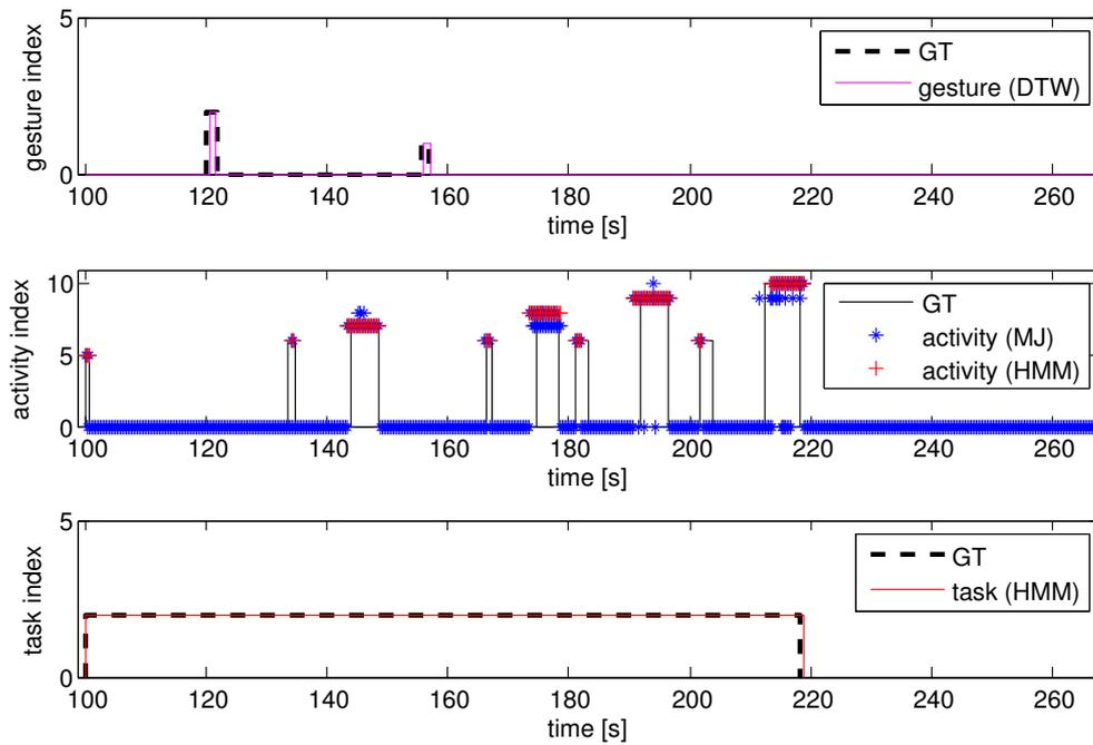
**Figure 7.7:** Recognition results of the PC assembly and gesture recognition experiment part 2. The results have been recorded during the execution of gestures 2 and 1 and task number 2.
