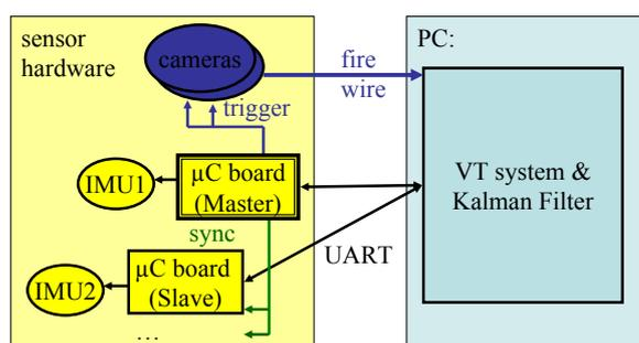
**Figure 3.2:** Scheme for hardware synchronization of IMUs and cameras. Synchronization is done by means of microcontroller ( $\mu\text{C}$ ) connector boards. Camera images are triggered and  $\mu\text{C}$  clocks are synchronized by means of a master controller.
