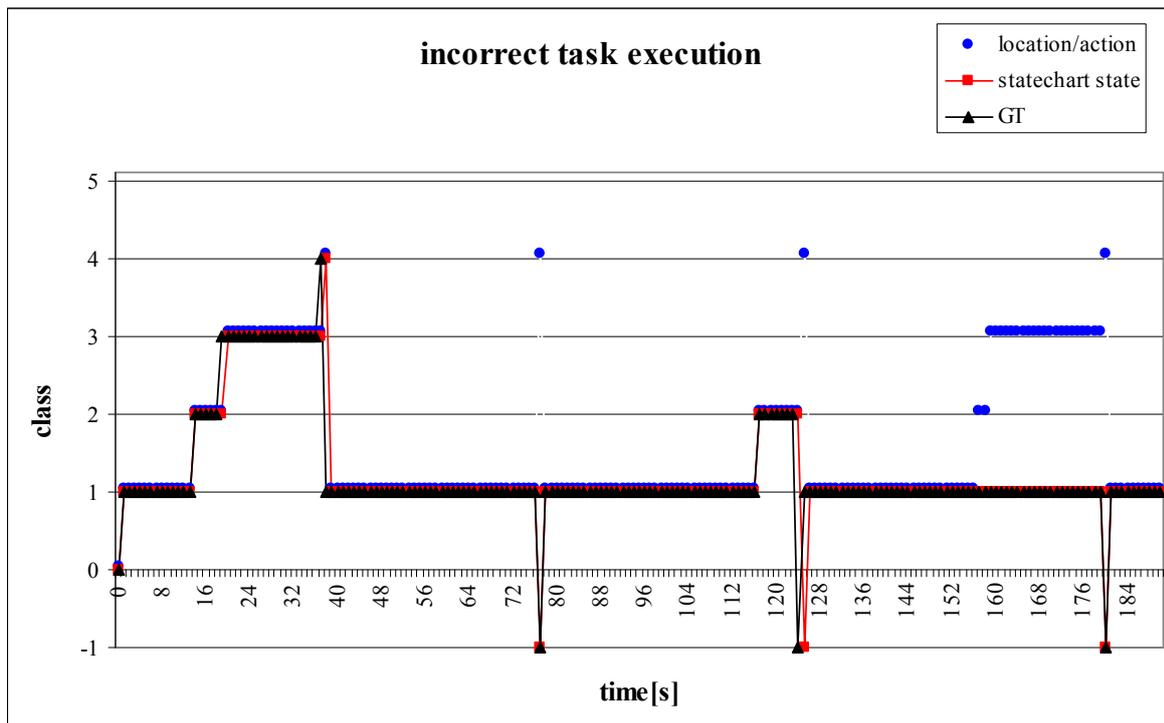
**Figure 7.5:** Recognition results of an incorrectly executed spot welding task. For the plot the same class indices have been used as in figure 7.4.
