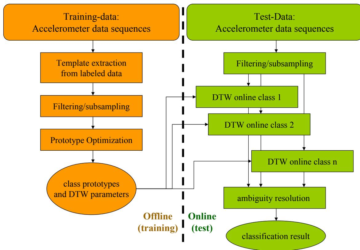
**Figure 6.6:** Scheme of the gesture recognition process. Class prototypes are extracted offline from training data in the training phase. Gesture recognition is applied in the online test phase to sequences of input data and is based on distance calculations to the class prototypes.
