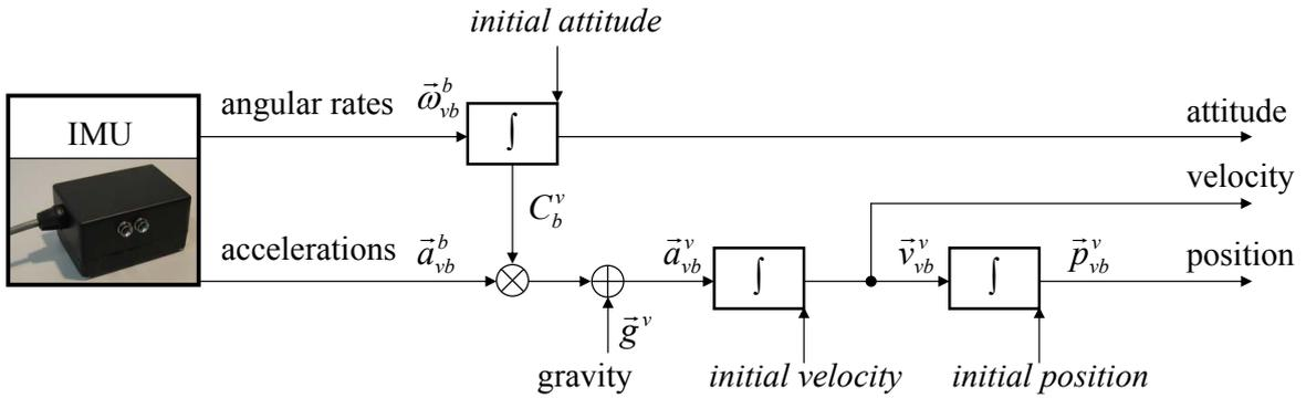
**Figure 3.4:** Block diagram of the strapdown model.
