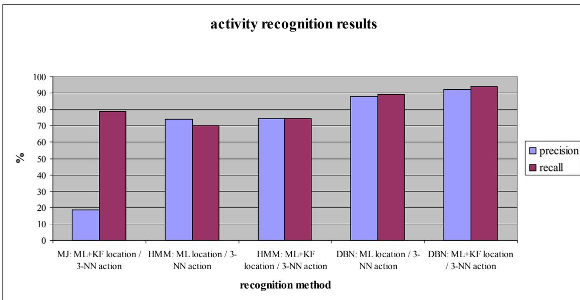
**Figure 5.7:** Comparison of activity recognition results. All tests are based on the detections from maximum likelihood location classification (with and without KF) and 3-NN action classification. For the HMM experiments location and action classification results have been fused by majority voting.
