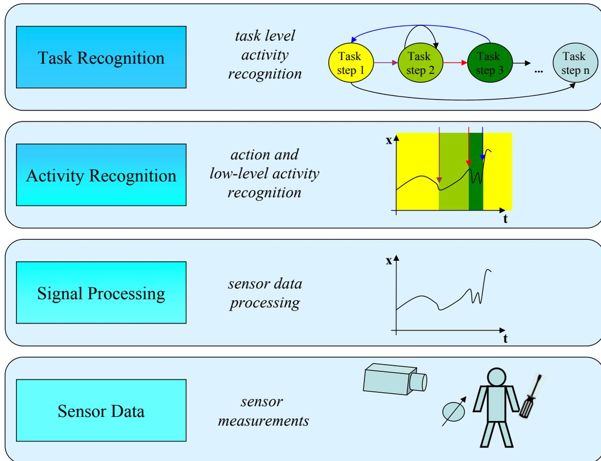
**Figure 2.1:** Hierarchical model describing the worker activity recognition process.
