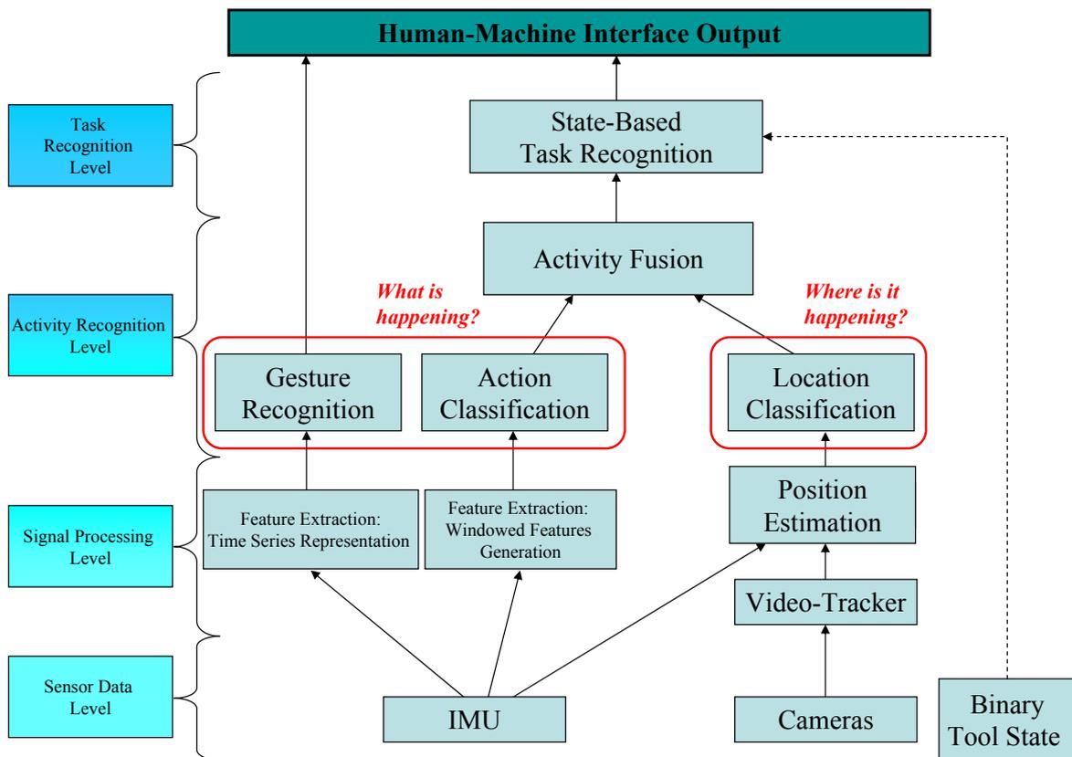
**Figure 2.2:** Overview about the main components of the human-machine interface.
