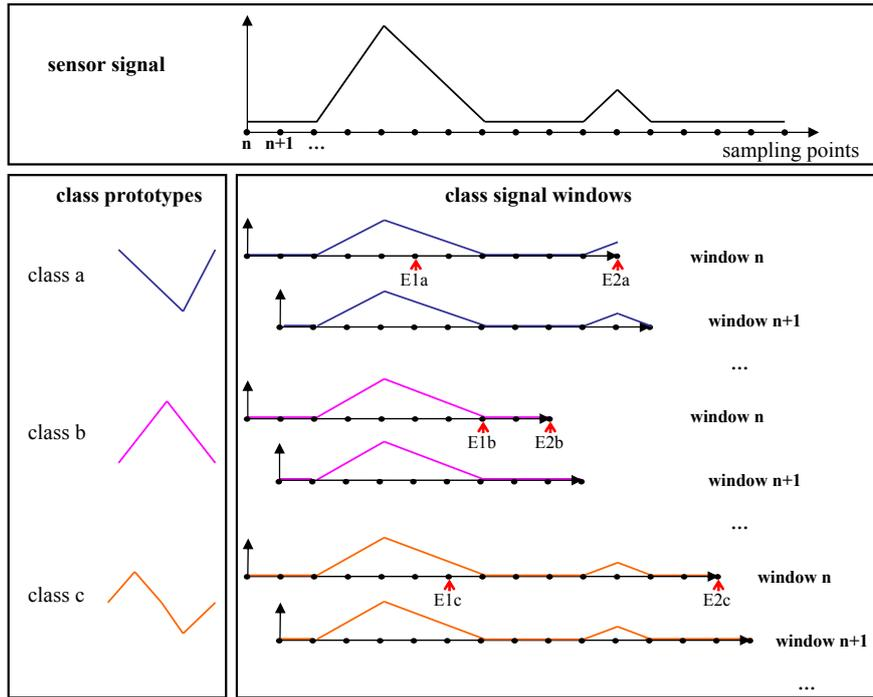
**Figure 6.2:** Online gesture recognition with multiple time series prototypes. Templates are extracted in parallel from an input data stream for distance calculations to each class prototype. Depending on the prototype, sliding windows with prototype depending lengths ( $E2$ ) are utilized.
