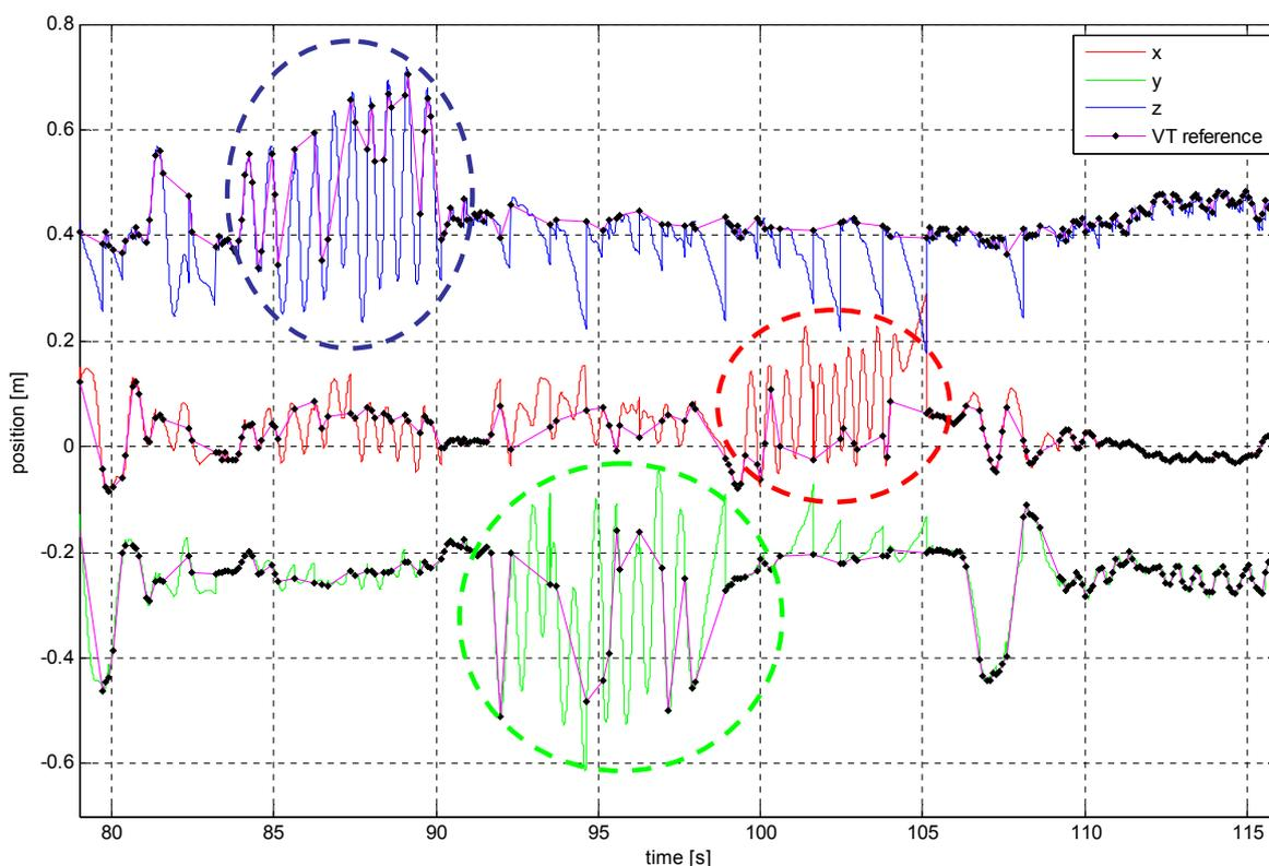
**Figure 3.12:** Example for lacking VT system position measurements, which are retrieved by the 9-state EKF model. Relevant areas are marked with dashed circles.
