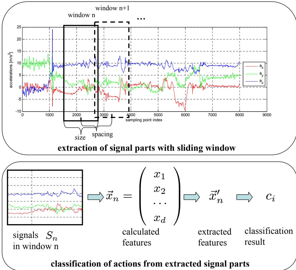
**Figure 4.1:** Classification of actions from sensor signals based on a sliding window. Top: Segmentation of recorded sensor data by means of a sliding window. Bottom: Classification of extracted segments.
