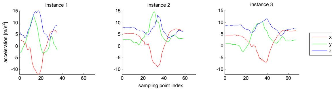
**Figure 6.1:** Gesture signals recorded with a triaxial accelerometer: The three instances of the gesture resemble each other in shape, but show spatial and temporal variabilities.
