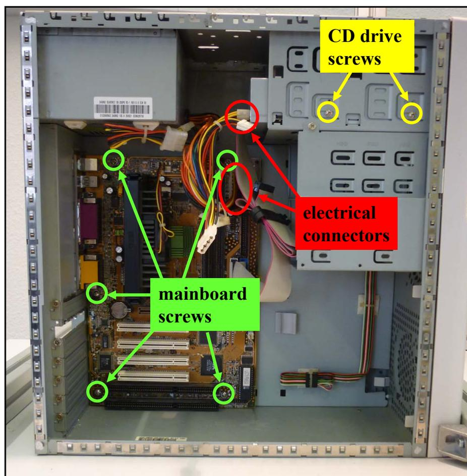
**Figure 4.7:** PC scenario: PC case with assembled components and locations of mainboard screws (screw 1-5), CD drive screws (screw 1+2 only, screw 3+4 are on the other side) and electrical connections (CD data connector is behind the CD power connector).
