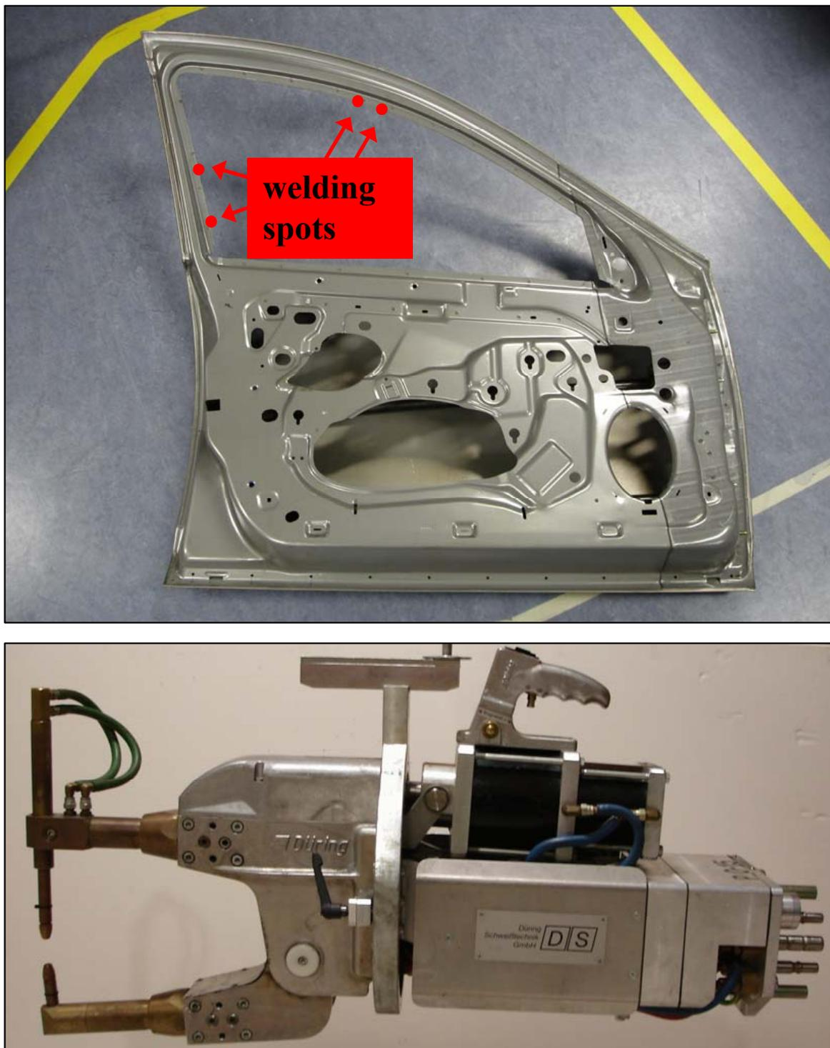
**Figure 7.1:** Car door (top) and hand welding gun (bottom).
