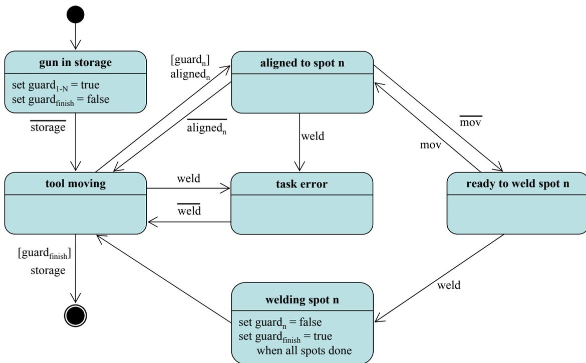
**Figure 7.3:** Statechart model of the spot welding task. Transitions between task states are modeled as actions and locations (storage = storage switch, weld = welding gun trigger, aligned<sub>n</sub> = below position threshold of spot *n*, mov = above motion threshold).
