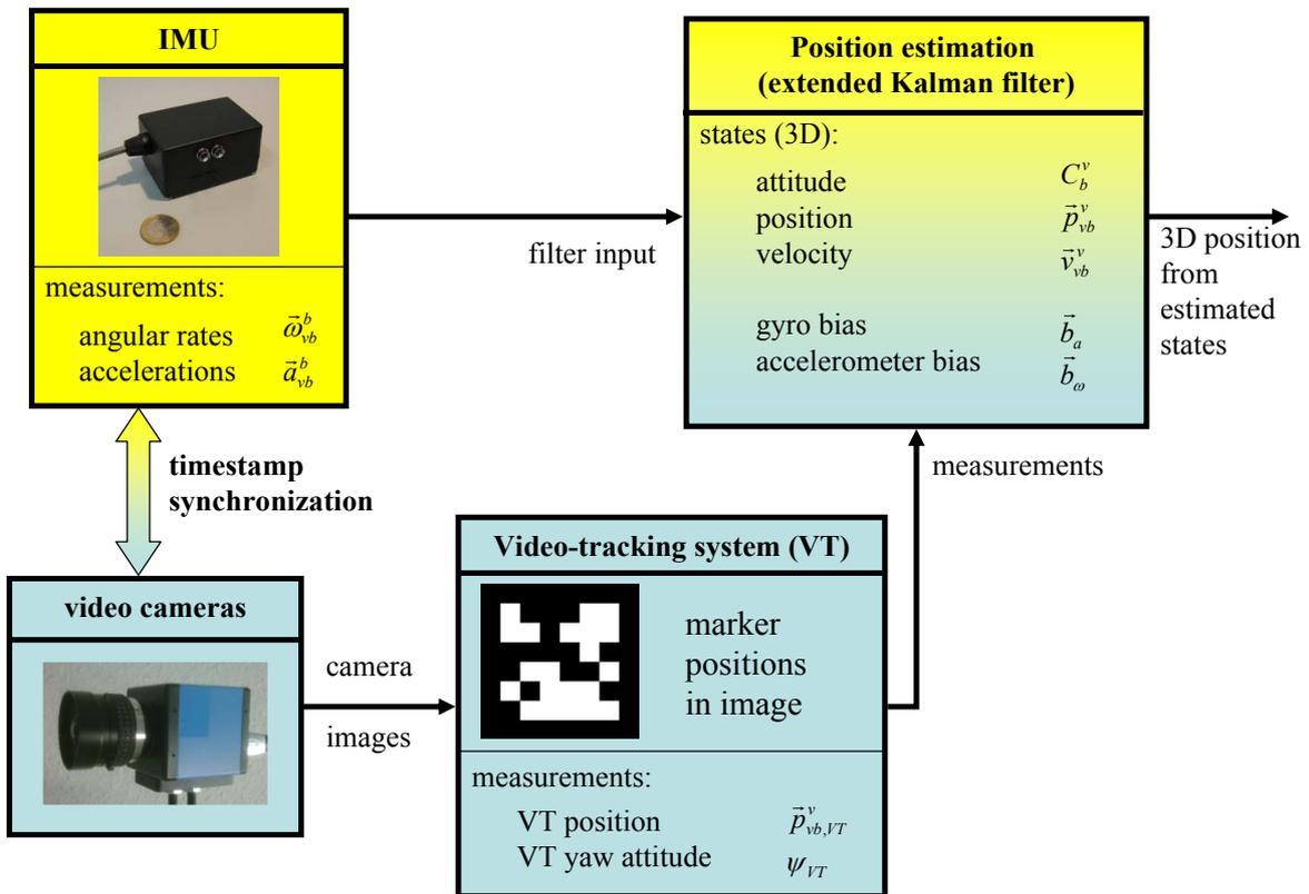
**Figure 3.1:** Components of the position estimation approach: IMU, video camera, VT system and position estimation with an extended Kalman filter.
