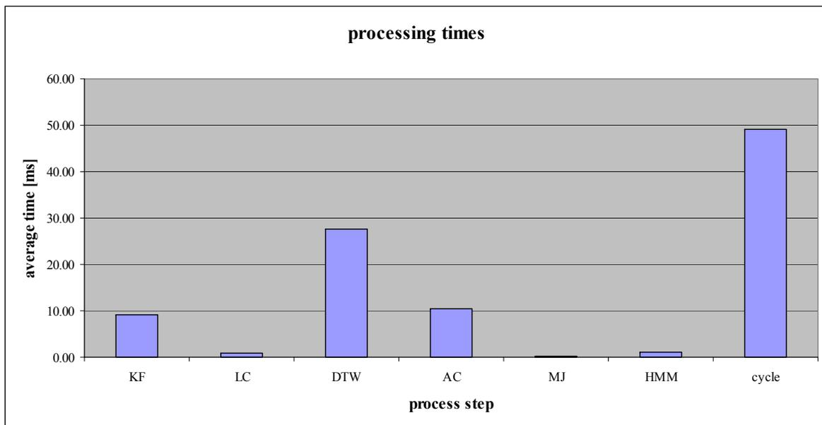
**Figure 7.10:** Processing time comparison of the components of the PC assembly demonstrator for input data measured during 1s in reality (KF = Kalman filter position classification, LC = location classification, DTW = online DTW gesture recognition, AC = action classification, MJ = activity recognition by majority voting, HMM = online HMM, cycle = complete processing cycle).
