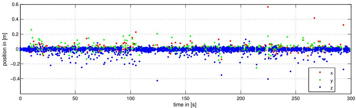
**Figure 3.11:** EKF result for a real data test sequence: Position deviation of estimations with the 9-state model to VT system measurements at the end of each outage.
