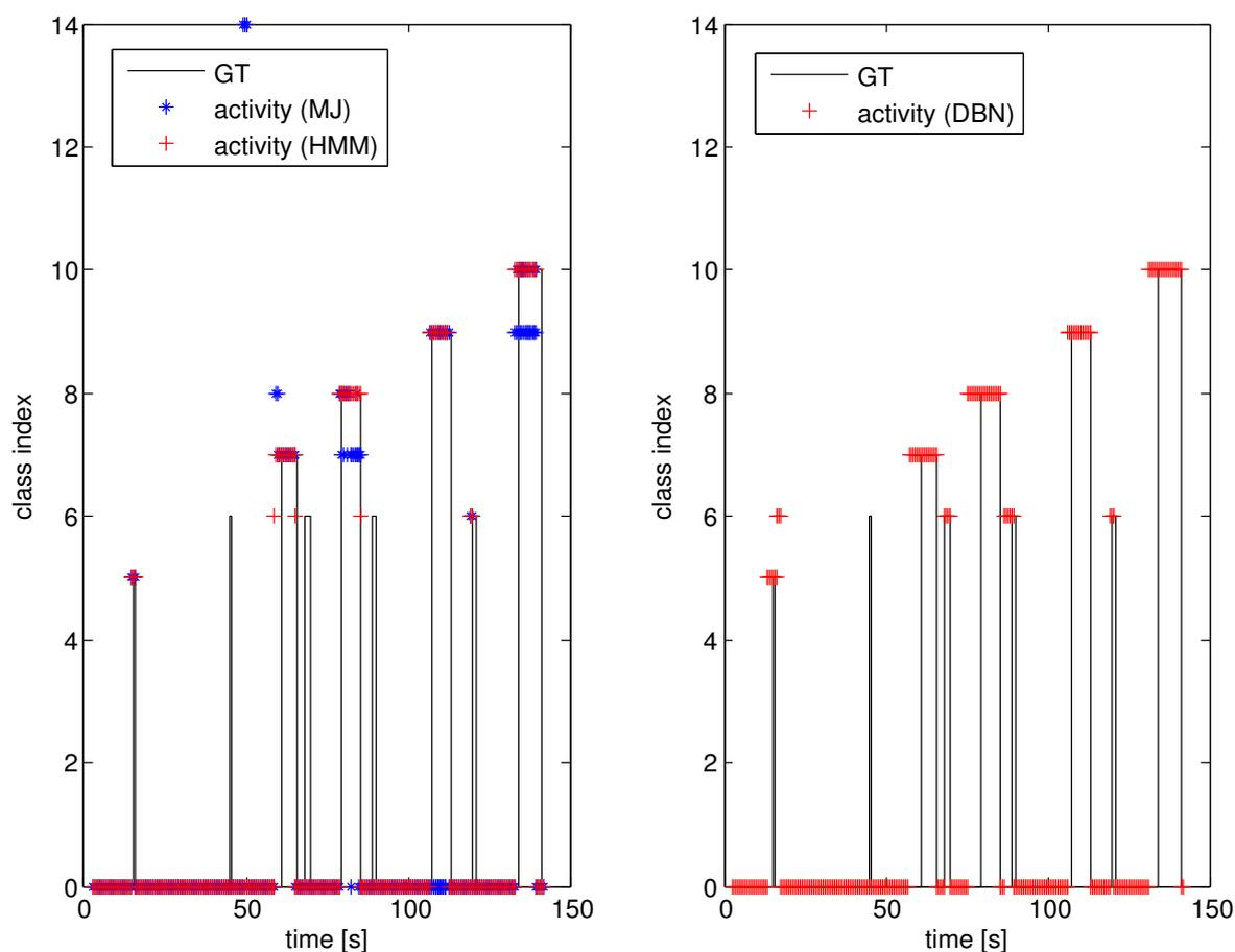
**Figure 5.6:** Result example for activity recognition with the HMM (left) and the DBN (right). Additionally, the majority voting result (MJ) is shown in the left plot as a basis for comparison. The test sequence, which has been used in this example, is of task class number 2.
