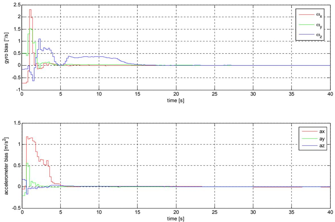
**Figure 3.8:** Estimation errors of the 15-state EKF model after application to a sequence of simulated data with outages: Gyro and accelerometer biases.
