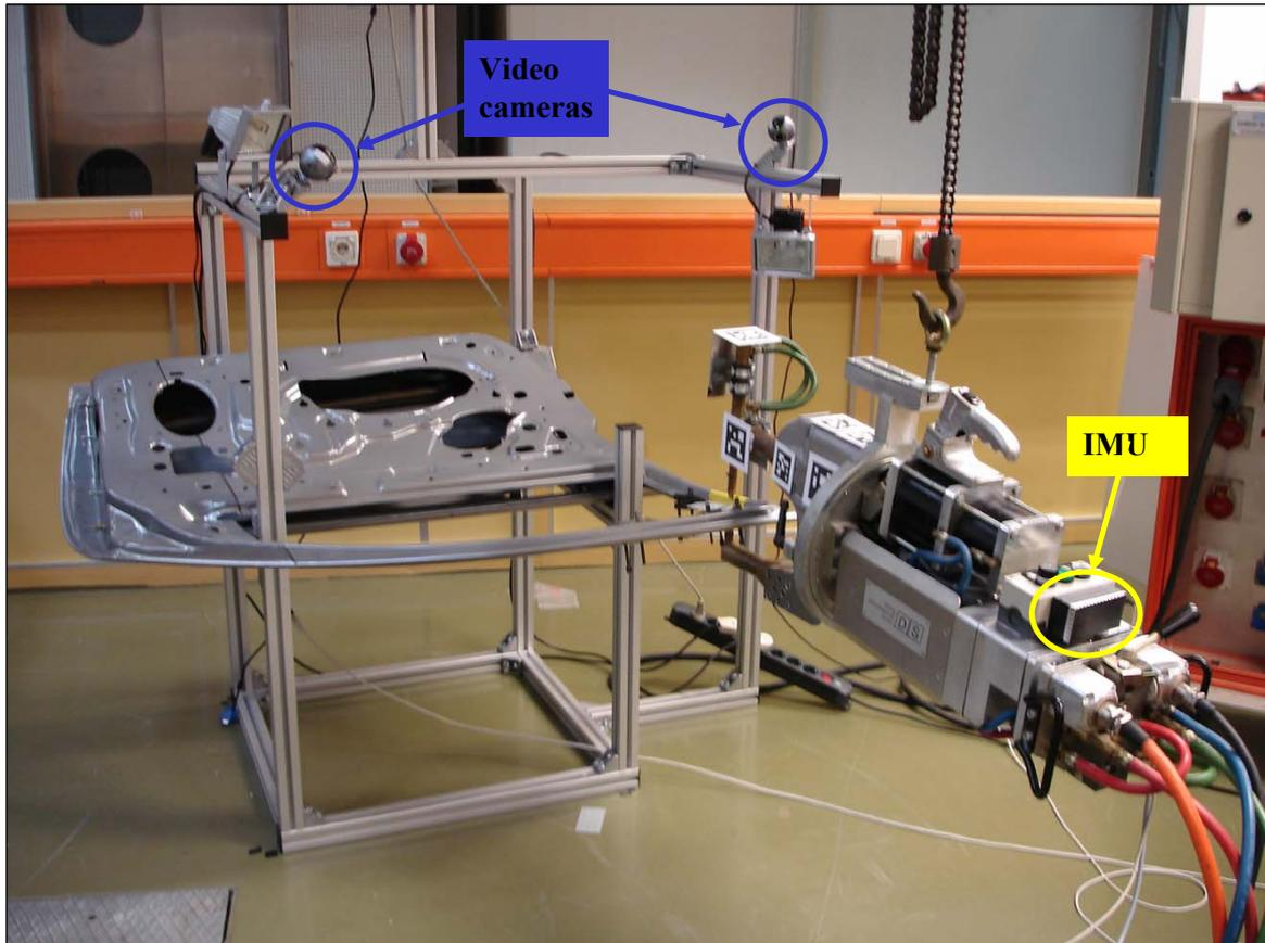
**Figure 7.2:** Experimental setup of the spot welding demonstrator with welding gun and car door. The locations of the video cameras and the IMU are indicated.
