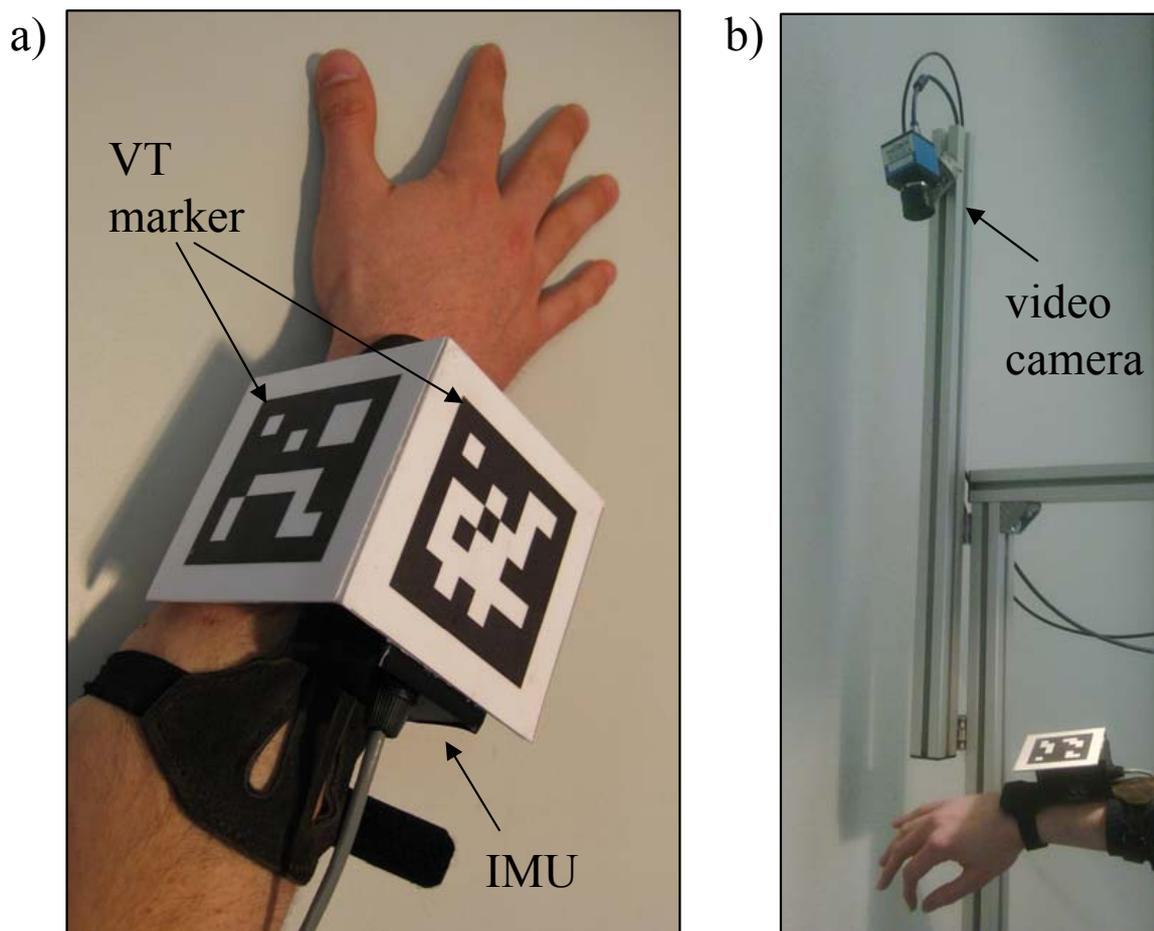
**Figure 3.10:** Setup for real data tests with the position estimation system: a) Sensor bracelet with IMU and VT markers. b) Camera position for recording hand movements.
