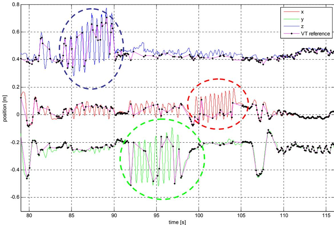
**Figure 3.14:** Example for lacking VT system position measurements, which are retrieved by the 15-state EKF model. Relevant areas are marked with dashed circles.
