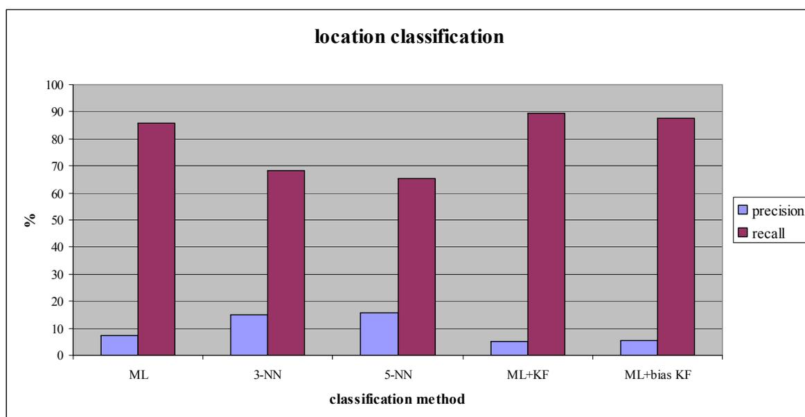
**Figure 4.10:** Location classification results of the maximum likelihood (ML) and the k-NN classifier (for k=3 and 5) in the PC scenario (recognition rates are averaged over all classes). Additionally, results of ML location classification applied to Kalman filtered data is shown for the 9-state (KF) and the 15-state (bias KF) EKF models.
