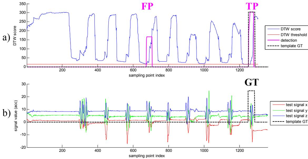
**Figure 6.8:** Online DTW applied to a gesture sequence (utilizing a prototype of class number 9): a) Online DTW score value, GT (black dashed line) and detections (one true positive overlapping with the GT and one false detection). b) Accelerometer signals (in  $m/s^2$ ) with GT.
