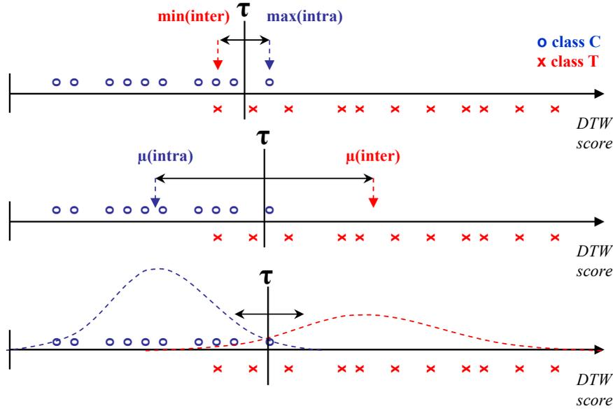
**Figure 6.4:** Different target function models applied to a distribution of DTW score values produced by a prototype of class C (from top to bottom): Minimal interclass to maximal intraclass distance, center point distance and distribution-based distances (Kullback-Leibler divergence and error function integral model).
