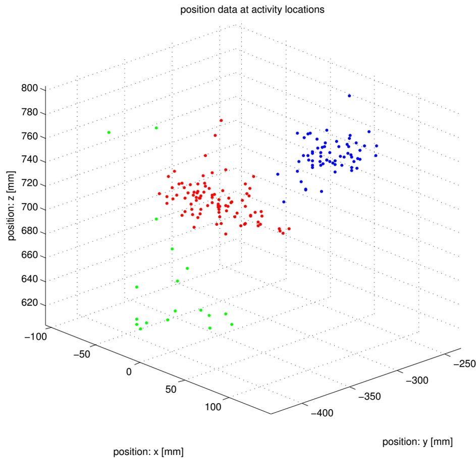
**Figure 4.4:** Hand position measurements recorded during the execution of three different activities of a manual assembly task. The position measurements appear as point clouds belonging to different location classes, which are indicated by the colors red, green and blue.
