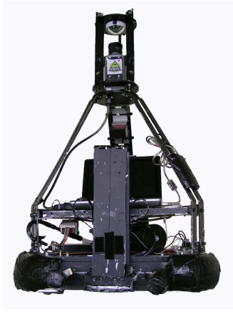
Figure 2: Robot of the team Brainstormers Tribots in the year 2007. From top to bottom the picture shows the omnidirectional camera, an additional perspective camera, the control laptop, the kicking device, and the chassis.
