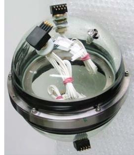
(c) Pressure hull made of glass resistant to 10,000 m water depth.
