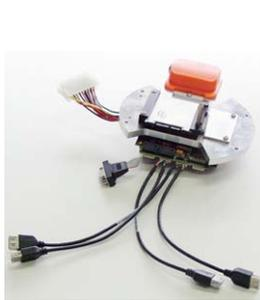
(b) Top view: inertial measurement unit and SSD data storage.
