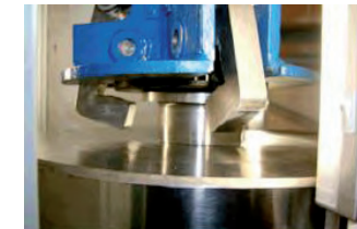
Figure 4: Opening of the grab in the borehole
