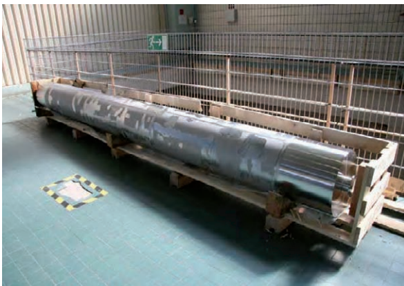
HLW Triple Pack (3 HLW dummies in steel envelope)
