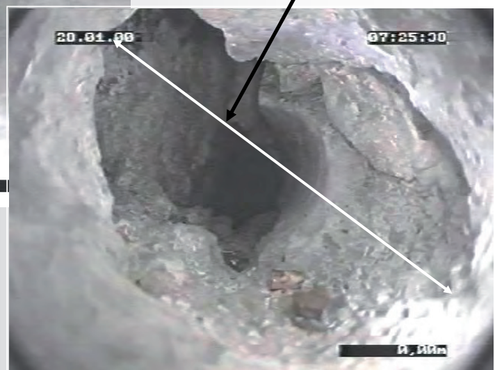
Open fractures and break-outs in pillar 3/4, depth 658 m, video inspection from January 2000
