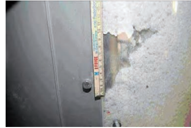
remaining small triangular space (BSK 3 leaning against borehole wall)
