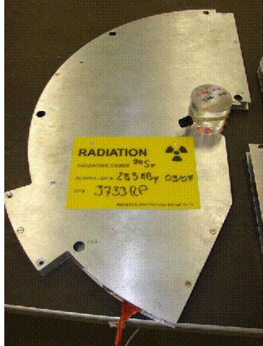
Figure 6.1: Setup used to test all diamond channels of the final system. To generate a signal a  $^{90}\text{Sr}$  source was put on top of the diamond packages.
