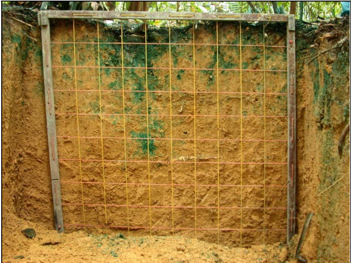
FIG. 2: DYED PROFILE IN PRIMARY FOREST. COUNTING FRAME WITH A SIZE OF 100 X 100 CM. MANY TERMITE-MADE STRUCTURES WERE FOUND IN THIS PROFILE
