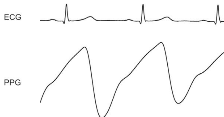
Figure 3-3: The pulsatile (AC) component of the PPG signal and corresponding electrocardiogram (ECG) [All07].
