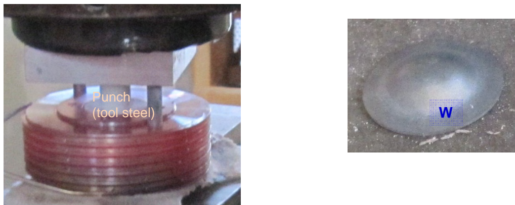
Fig. 2: First W deep draw attempt with a new developed tool (left), thimble cap from 1 mm W sheet (right).
