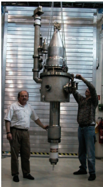
Fig. 1: Coaxial 2.2 MW 170 GHz short pulse pre-prototype gyrotron at KIT (left) and the industrial long pulse prototype, installed at the CRPP test stand (right). The blue sphere is the CNR 2 MW RF load (see fig. 4).
