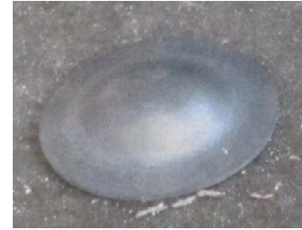
First W deep draw attempt with a new developed tool (left), thimble cap from 1 mm W sheet (right)
