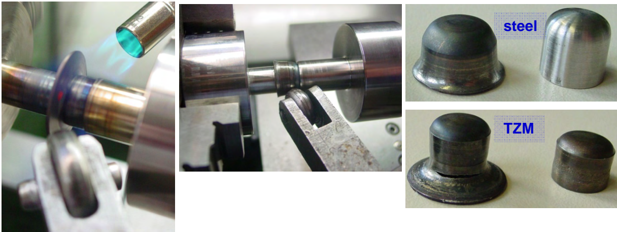
Fig. 1: Roll pressing attempt using butane gas heating (left), thimble cap from 1 mm sheet of steel and TZM (right).
