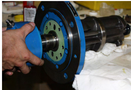
Fig. 4: Oil-pump for compressor V2 of the 2 kW-refrigerator.
