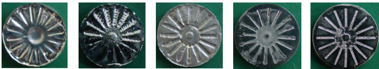
Fig. 3: Effect of pulsed currents. From left to right increasing pulse frequency 0 Hz; 10 Hz; 100 Hz; 500 Hz; 1000 Hz.
