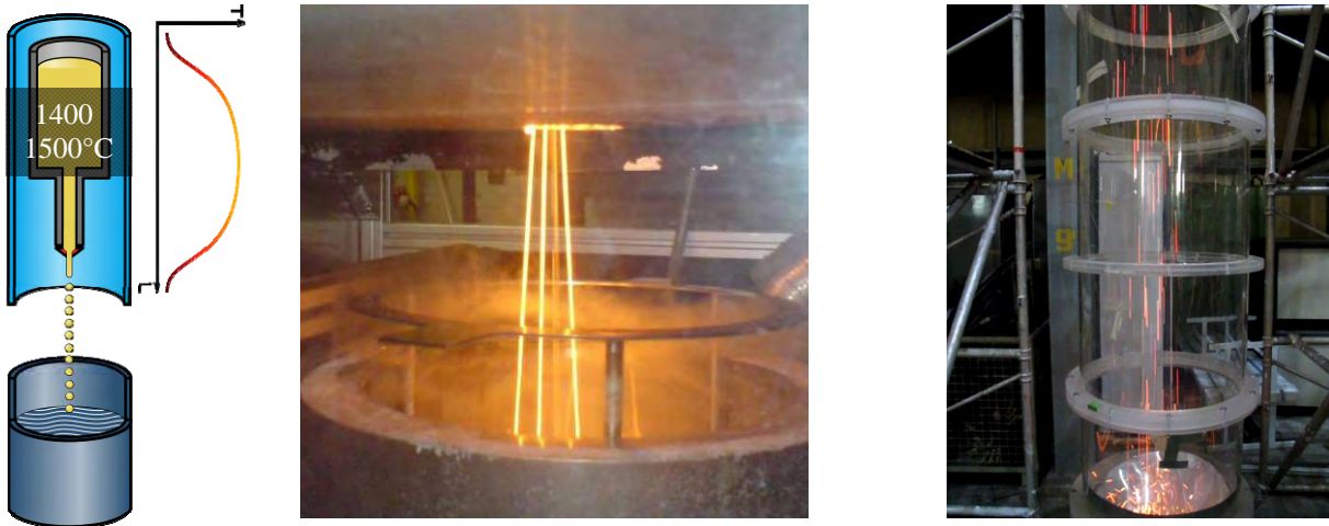
Fig. 5: Experimental setup – test facility (drawing), triple nozzle experiment, and test with a drop height of 14 m.
