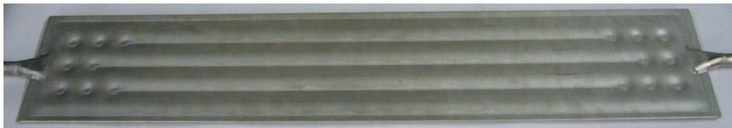
Fig. 4: Picture of one 1:1 scaled hydroformed cryopanel (1m long x 0.2 m wide).
