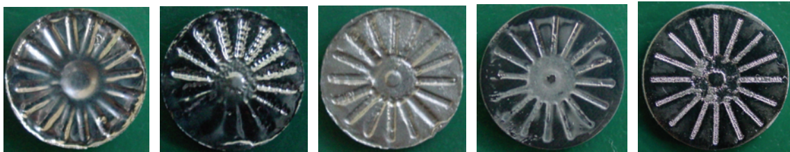
Effect of pulsed currents. From left to right increasing pulse frequency 0 Hz; 10 Hz; 100 Hz; 500 Hz; 1000 Hz
