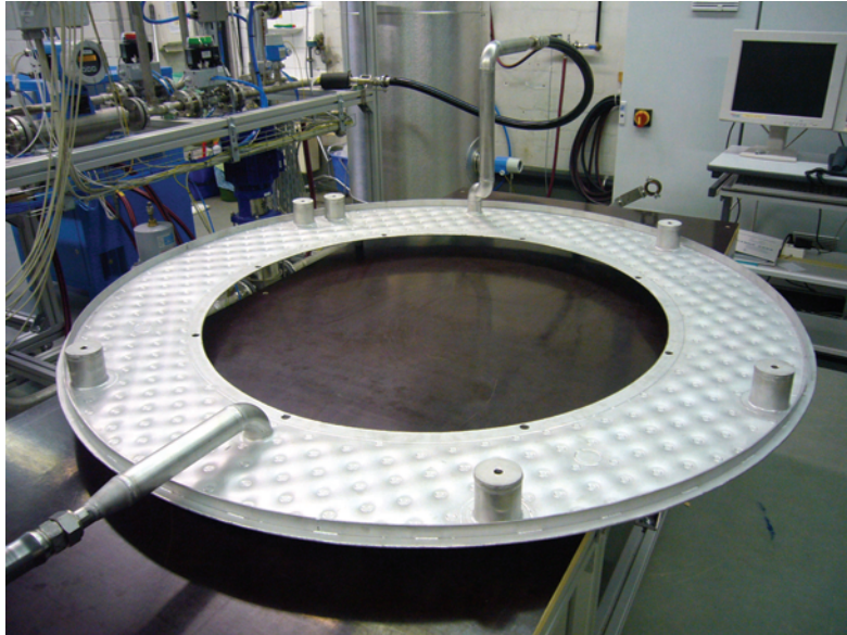
Fig. 3: Picture of the 1:1 scale hydroformed PPC front shield (external diameter of 1510 mm).
