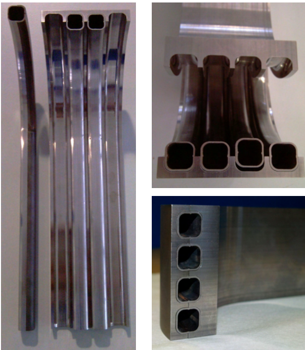
Fig. 3: Assembling the single parts (bended pipes and plates).
