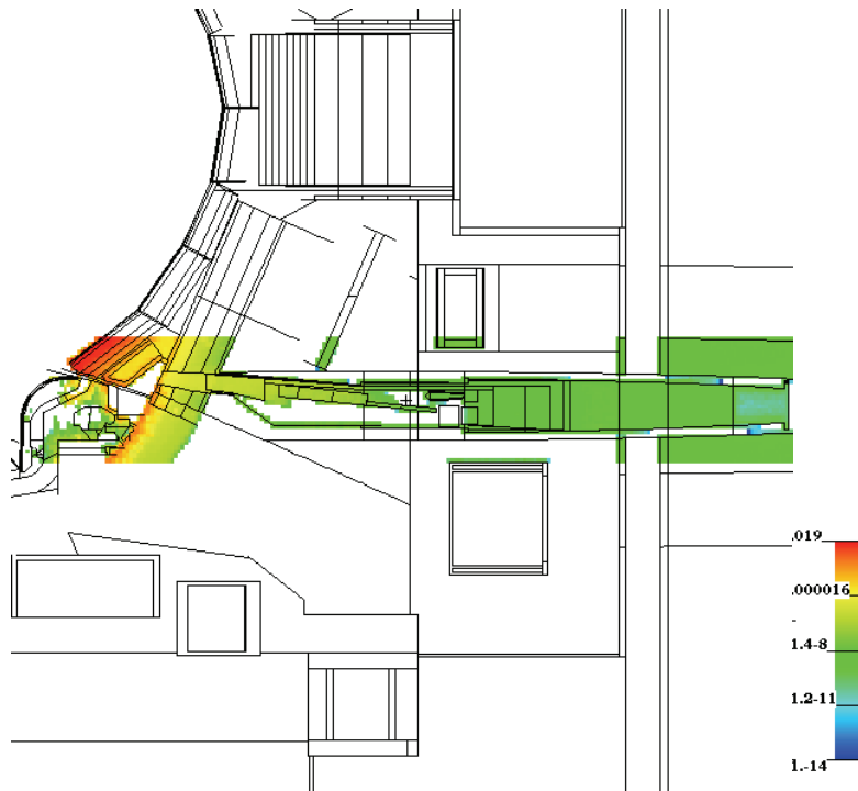
Fig. 2: Map of decay-photon heating distribution after 20 yr operation at cooling time 0 s [W/cm 3 ].
