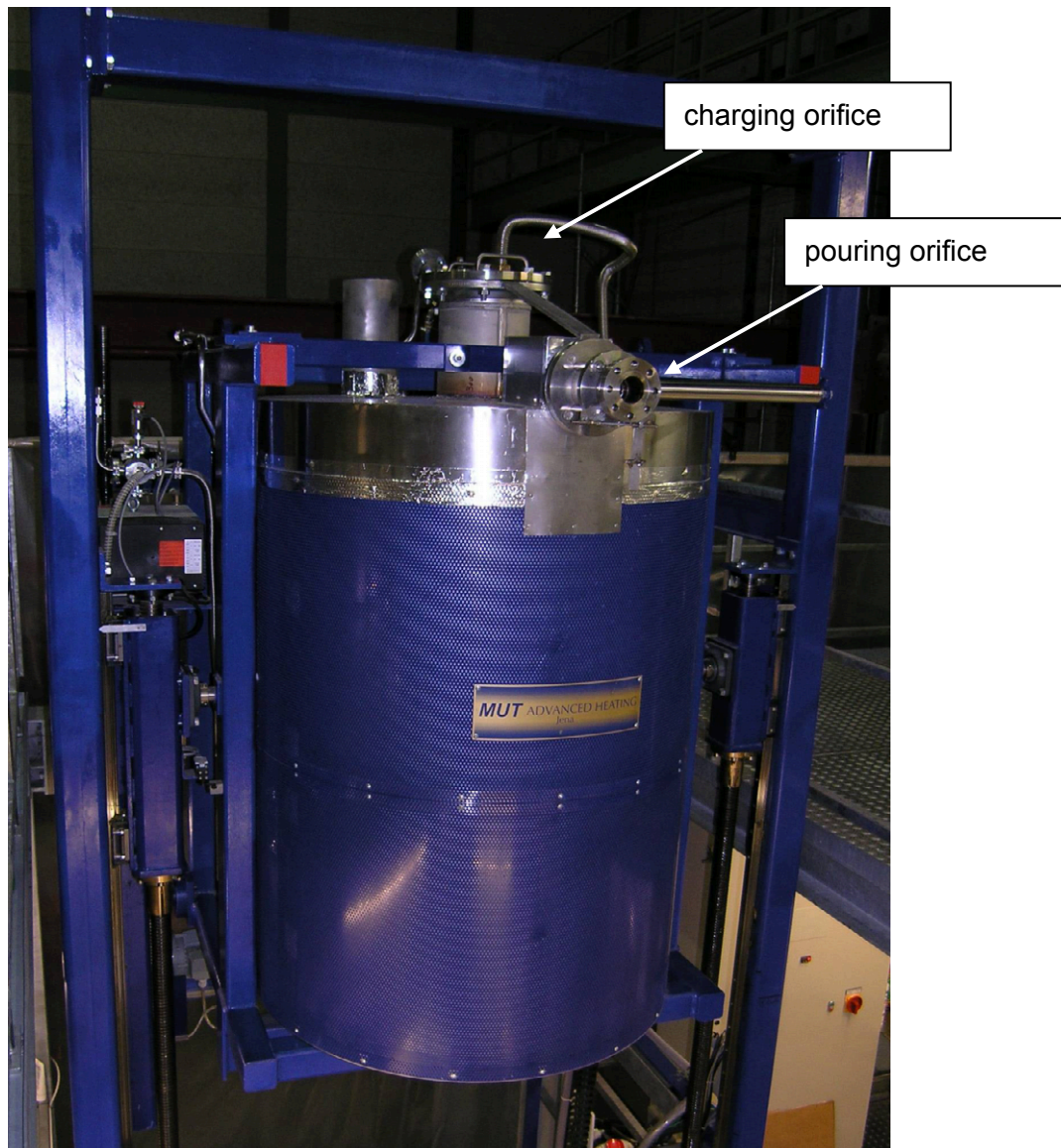
Figure 4: Picture of the heating furnace for the melting of simulant materials
