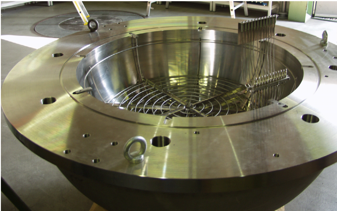
Figure 1: Picture of the LIVE test vessel with volumetric heating system
