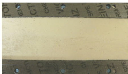
Fig. 6.4-2: View of the surface of the 5 \mu\text{m} Ag plated membrane placed in the reactor
