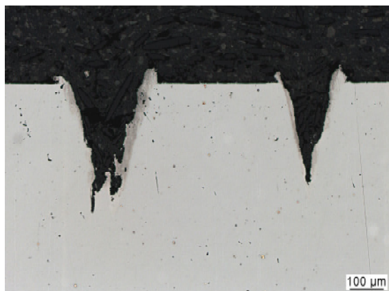
Fig 14-2: View of a sample engraved with optimized laser parameter: V-shape and desired dimensions have been produced
