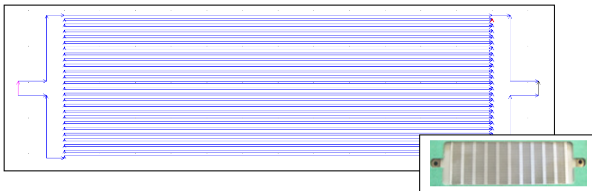
Fig. 8.4-1: Design of the central area of the hydroxylation reactor (drawn at scale 1) using COMSOL Multiphysics
