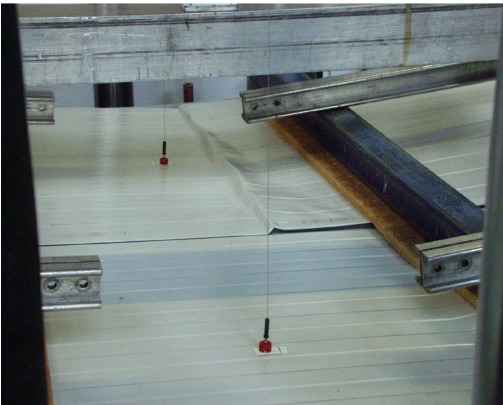
Fig. 17: Wrinkling failure of the panel at load p_3 = 14,1 kN
