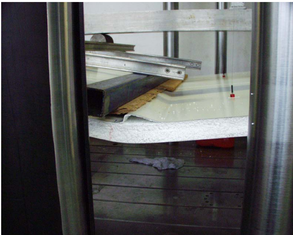
Fig. 7: Wrinkling failure of the panel at load p_3 = 20,1 \text{ kN}
