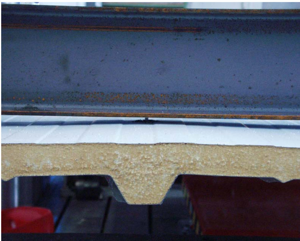
Fig. 15: Gap between face layer and beam
