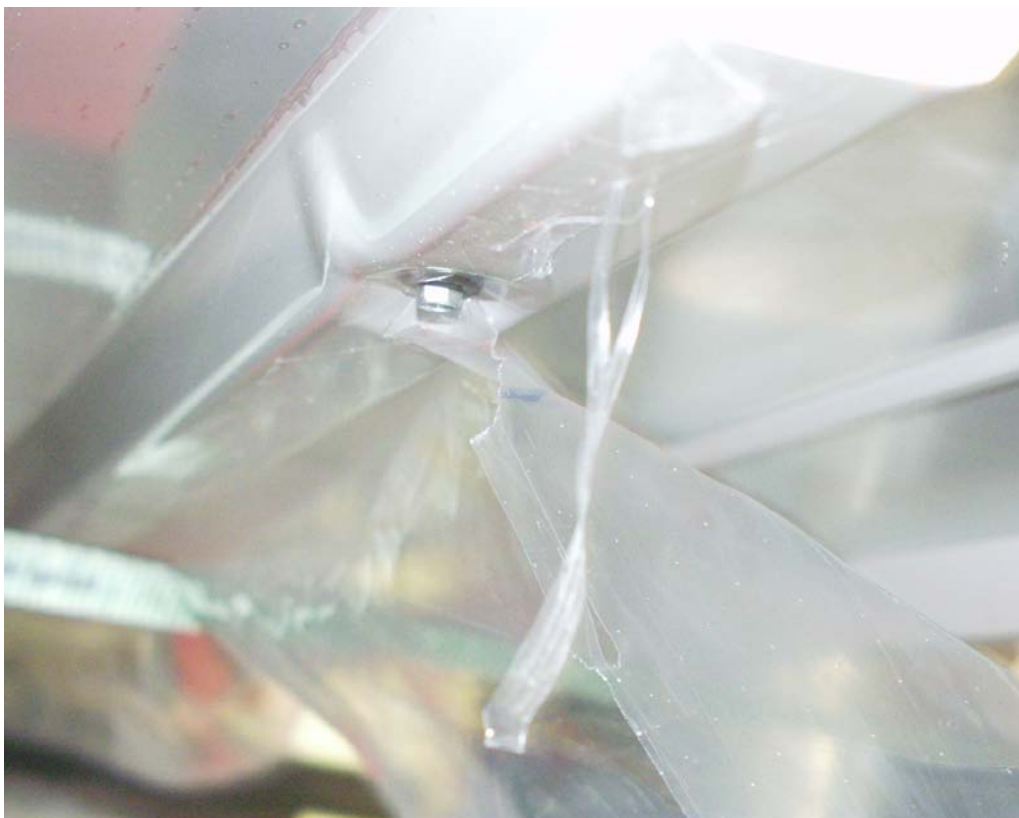
Fig. 18: Indentation of the fastener and web crippling
