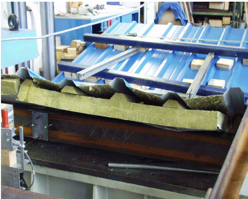
Fig. 14: shear failure of the panel at load p_3 = 15,0 kN
