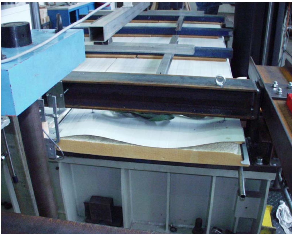
Fig. 12: Pull-through failure of the fasteners at load p_2 = 13,0 kN
