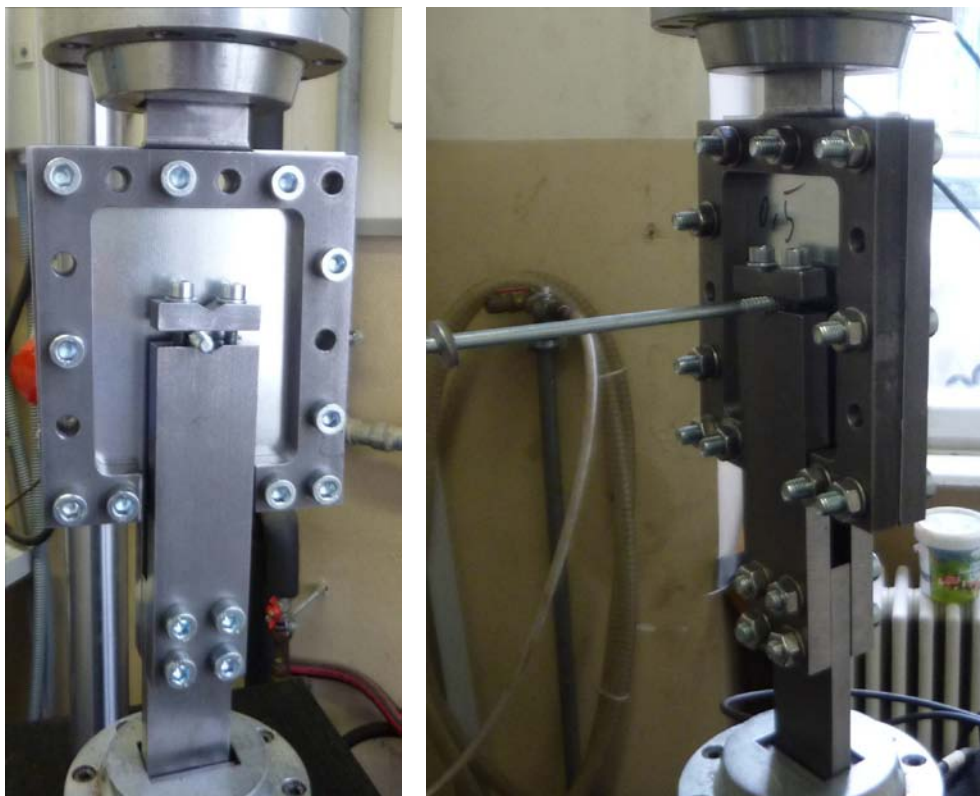
Fig. 6: Test set-up for hole elongation tests
