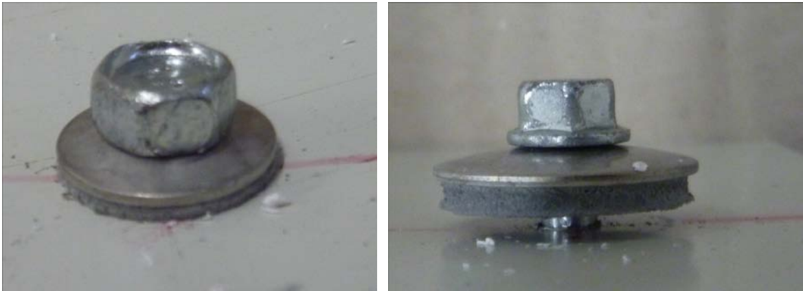
Fig. 9: Specimens with and without clamping of the head
