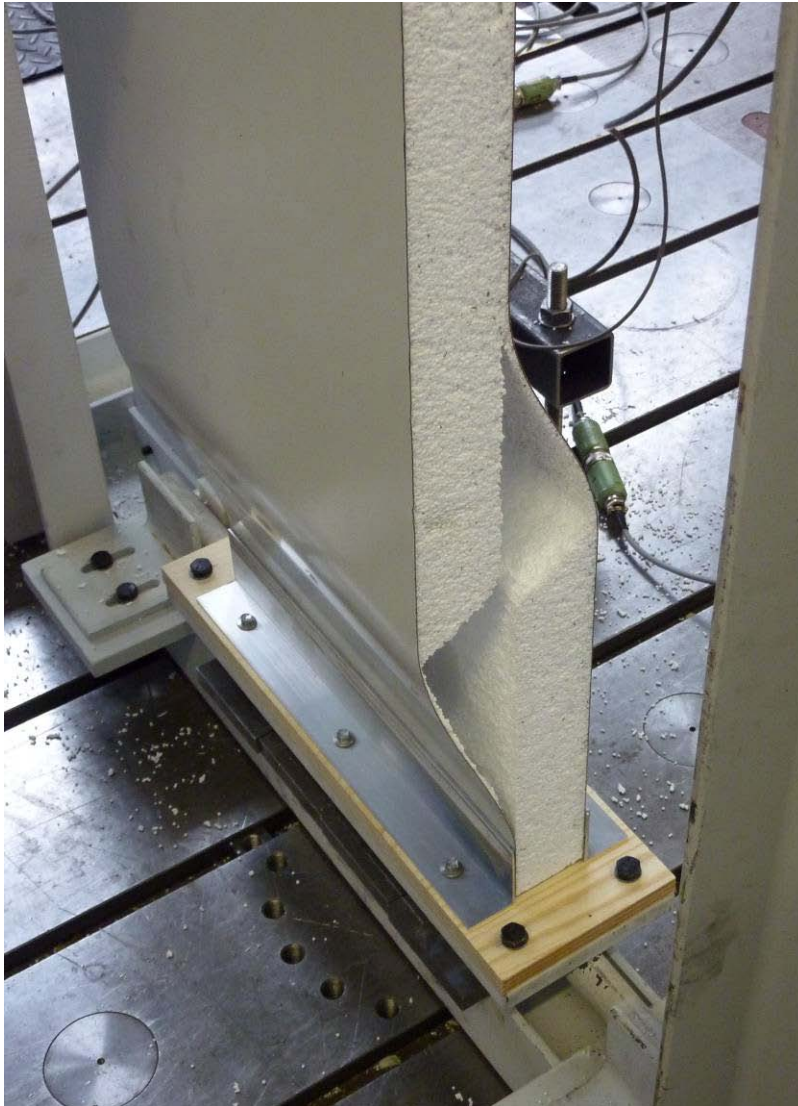
Fig. 12: Failure mode of test no. 04
