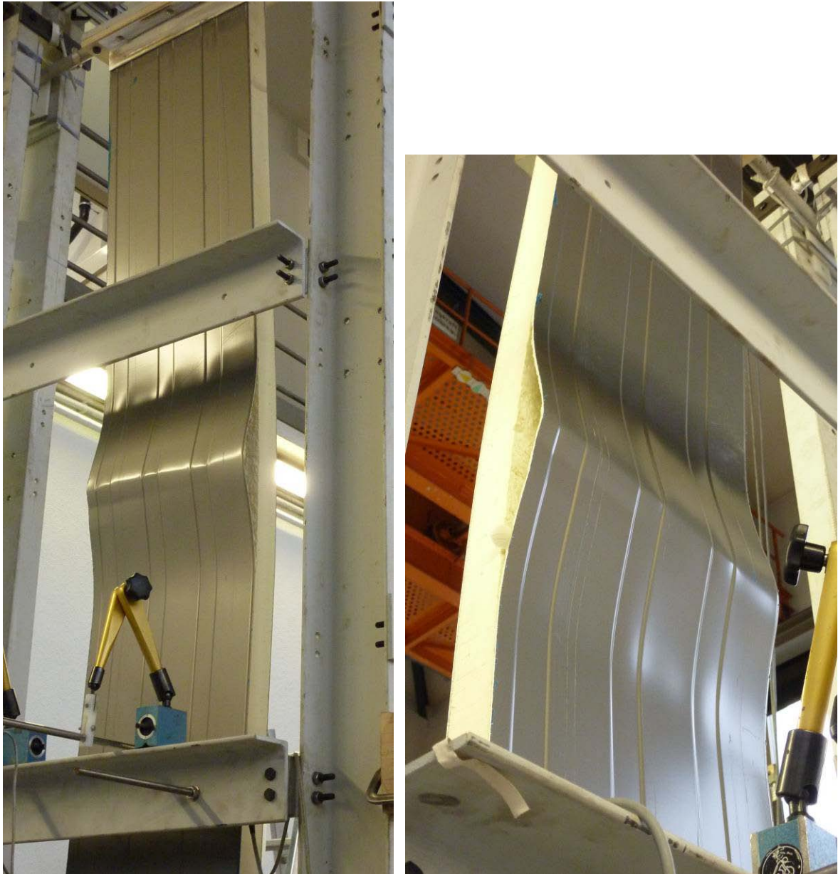
Fig. 20: Failure mode of test no. 09
