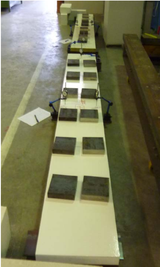
Fig. 13: Test set up of creep tests
