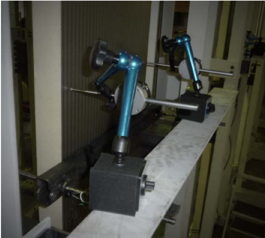
Fig. 9: Measurement of deflection and support at mid-span
