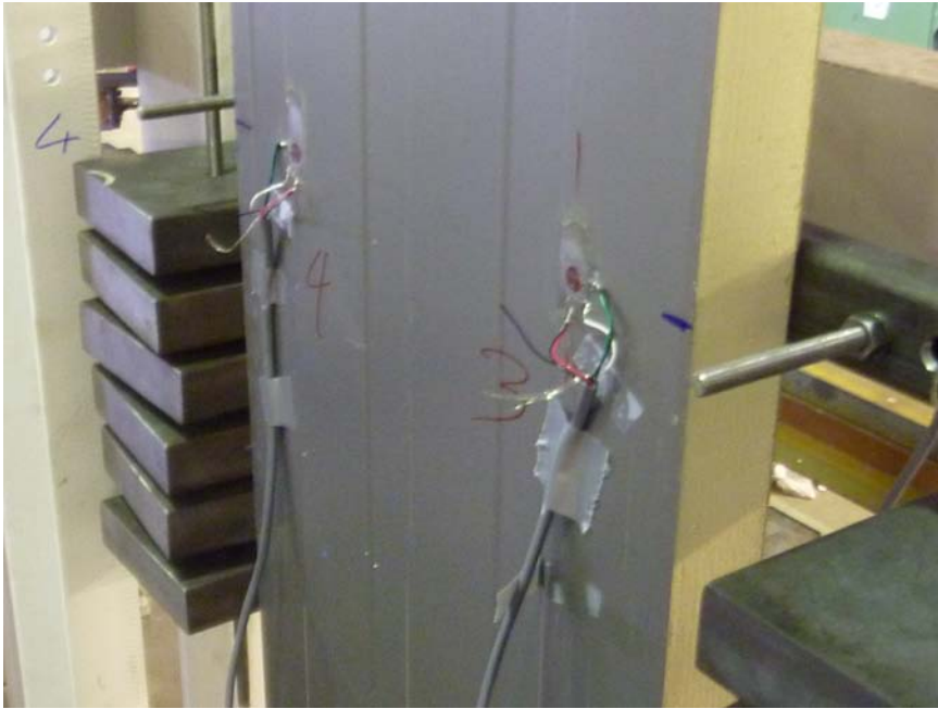
Fig. 11: Strain gauges at the face of the panel
