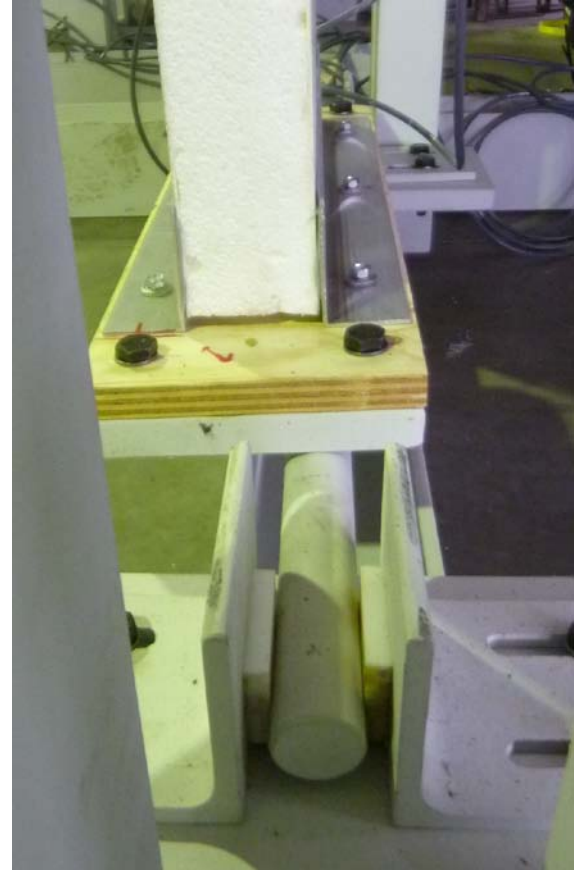
Fig. 8: Eccentric application of axial force
