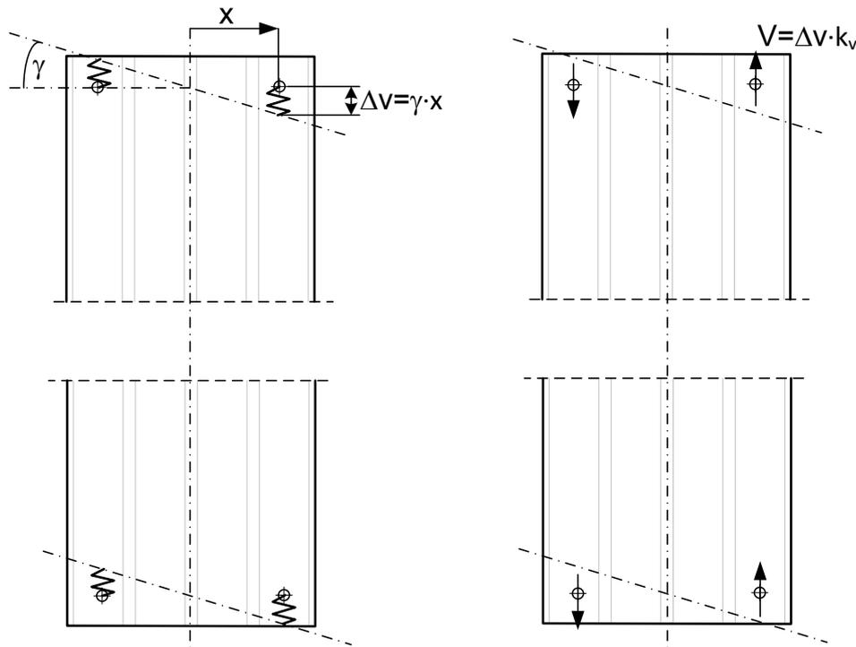
**Fig. 6.3: Displacement and forces of fastenings**
