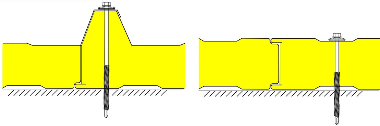
**Fig. 2.1: Connections of sandwich panels to a substructure**
