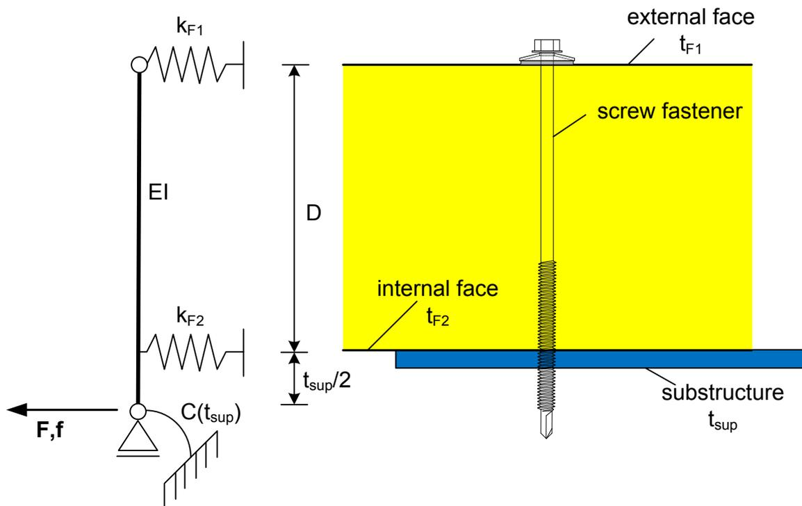
Fig. 3.1: Mechanical model of a fastening
