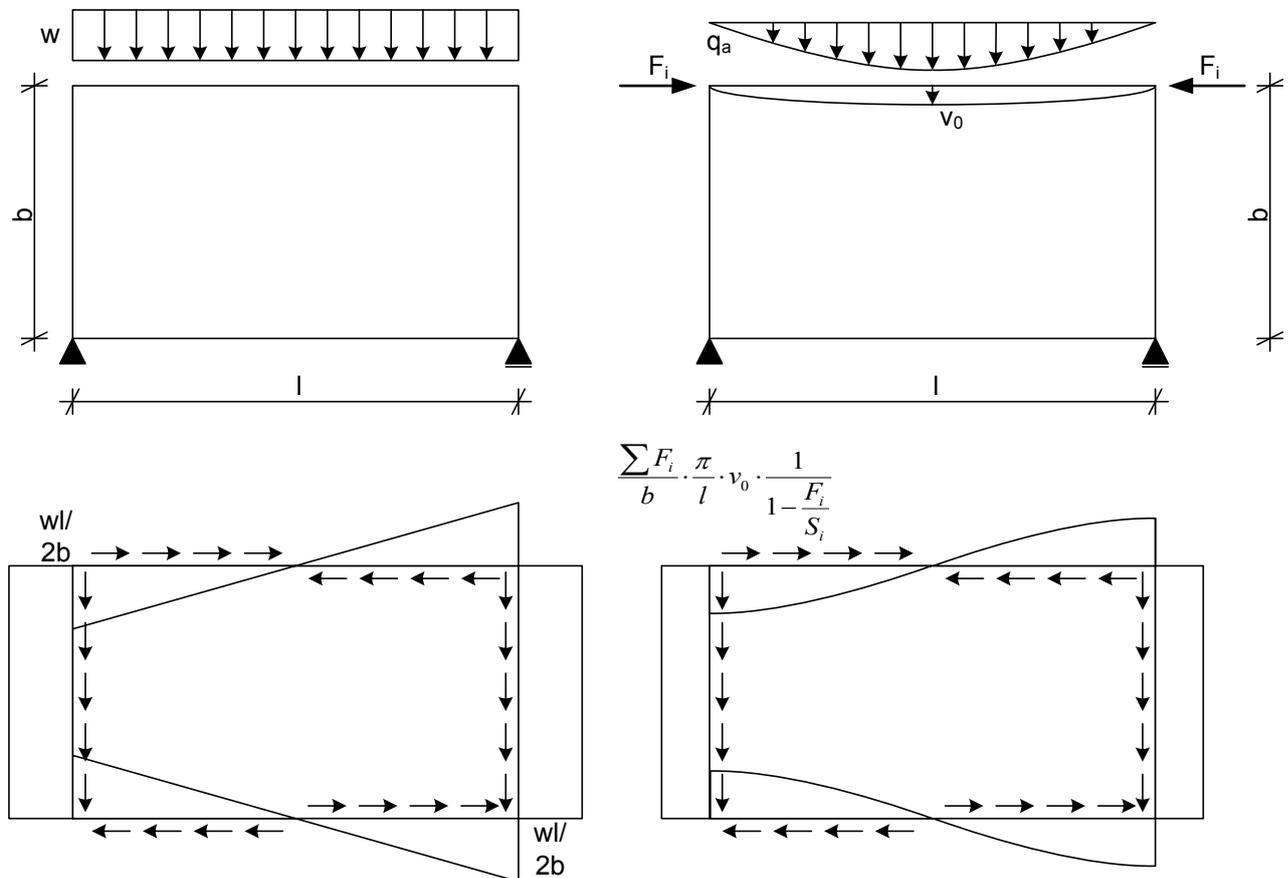
Fig. 8.8: Shear forces of diaphragms
