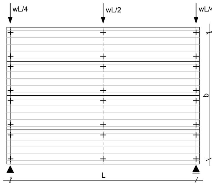
**Fig. 7.2: Application of loads by supporting beams**
