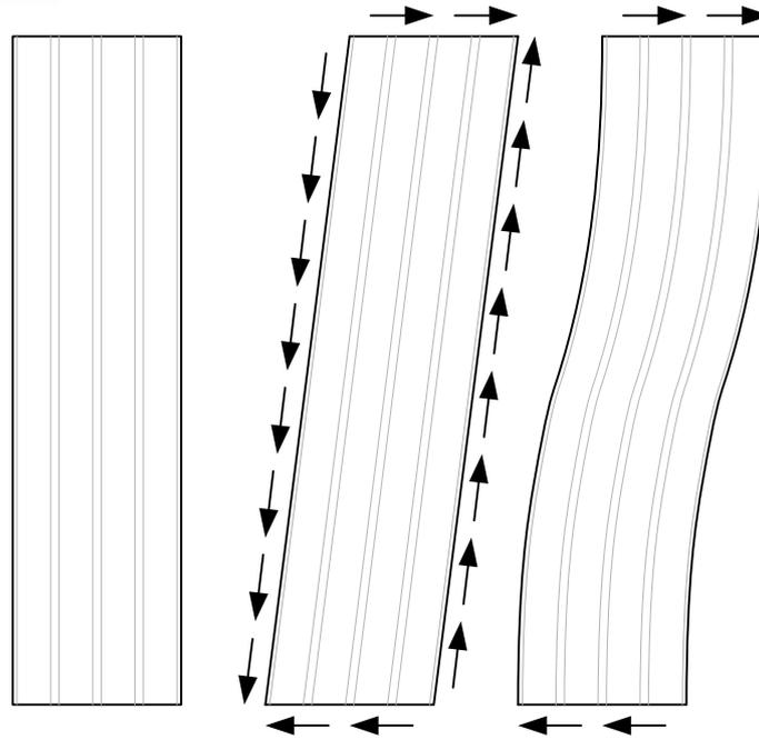
**Fig. 2.3: Load bearing systems: shear diaphragm and Vierendeel girder**
