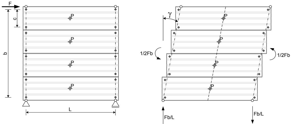
Fig. 6.1: Shear diaphragm with unidirectional spanning sandwich panels
