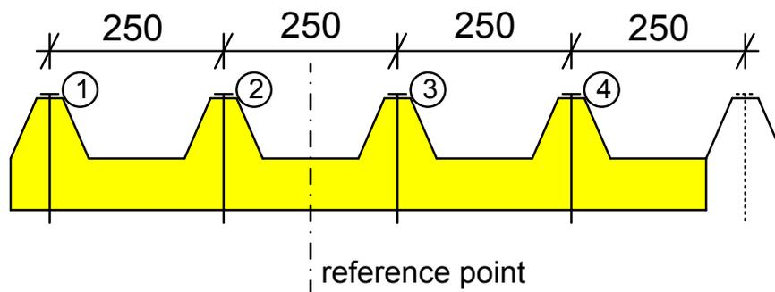
The diaphragm, which is used to transfer the horizontal load  $w$ , is given in the following figure.
