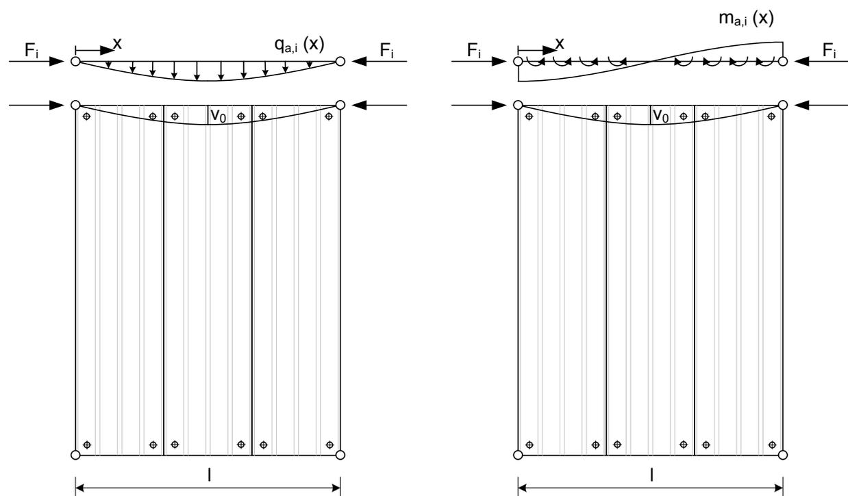
Fig. 7.4: Load resulting from stabilization of a single component
