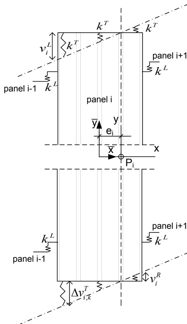
**Fig. 6.5: Model for determination of reference points**
