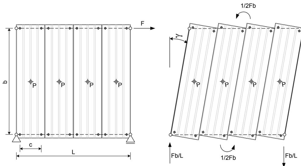
Fig. 6.2: Shear diaphragm with unidirectional spanning sandwich panels – continuation
