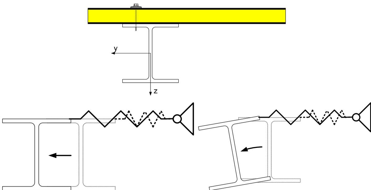
Fig. 5.1: Stabilization of beams by lateral restraint
