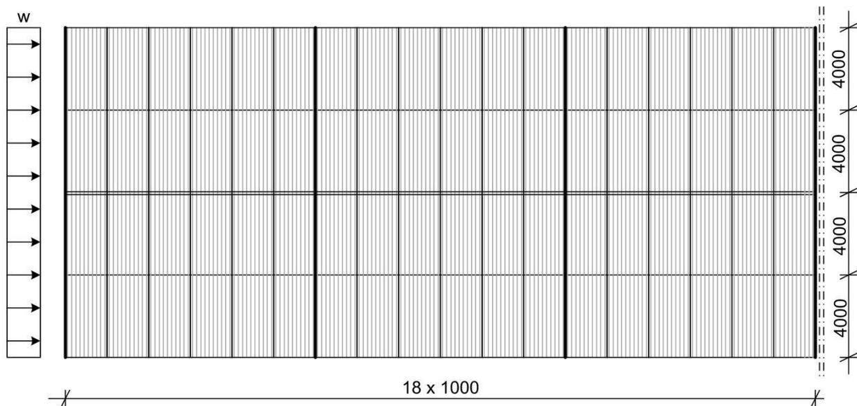
The panels are connected to the purlins as given in the figure below. There are not any connections at the longitudinal joints of the panels (or these connections are neglected).
