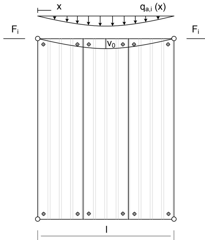
Fig. 8.6: Load resulting from stabilization of a beam
