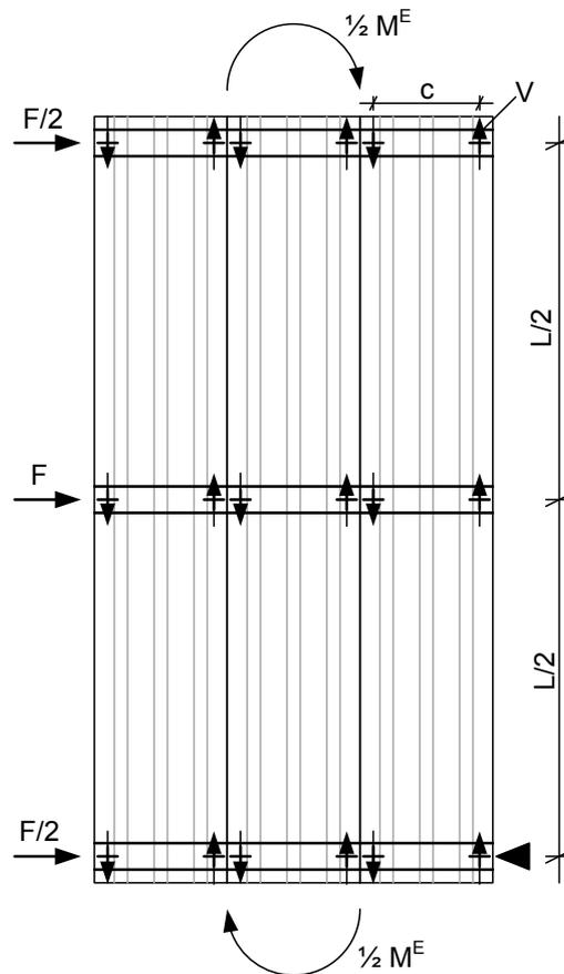
**Fig. 8.2: Shear diaphragm used to transfer horizontal loads**
