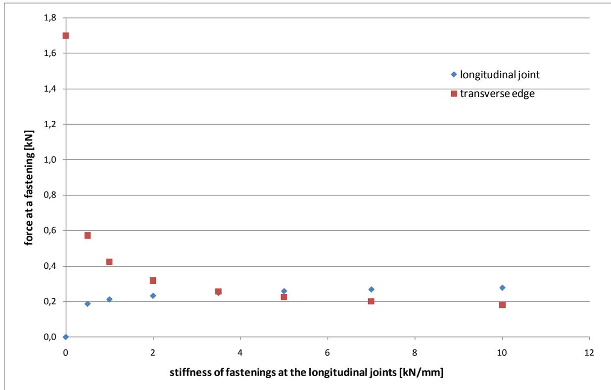
Concerning the forces of the fastenings there is a wide difference between diaphragms with and diaphragms without connections at the longitudinal joints. Even if the fastenings at the longitudinal joints have only a very low (not realistic) stiffness, the forces of the fastenings at the transverse edge decrease significantly. A further variation of the stiffness results in a comparatively slight modification of the forces of the fastenings.
