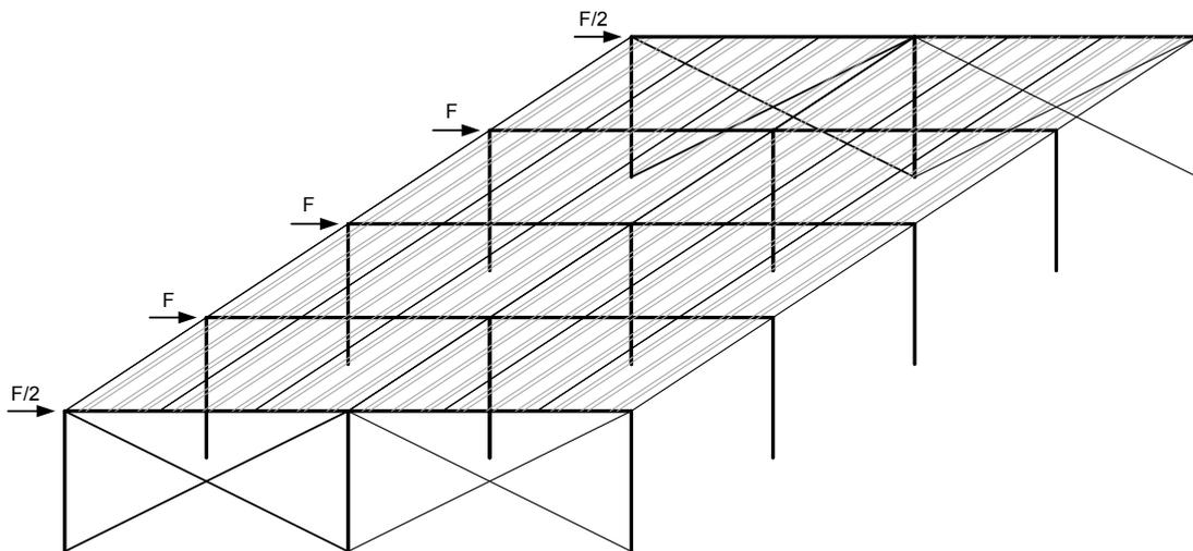
**Fig. 8.1: Transfer of horizontal loads**
