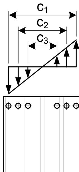
Fig. 8.4: Consideration of additional fasteners
