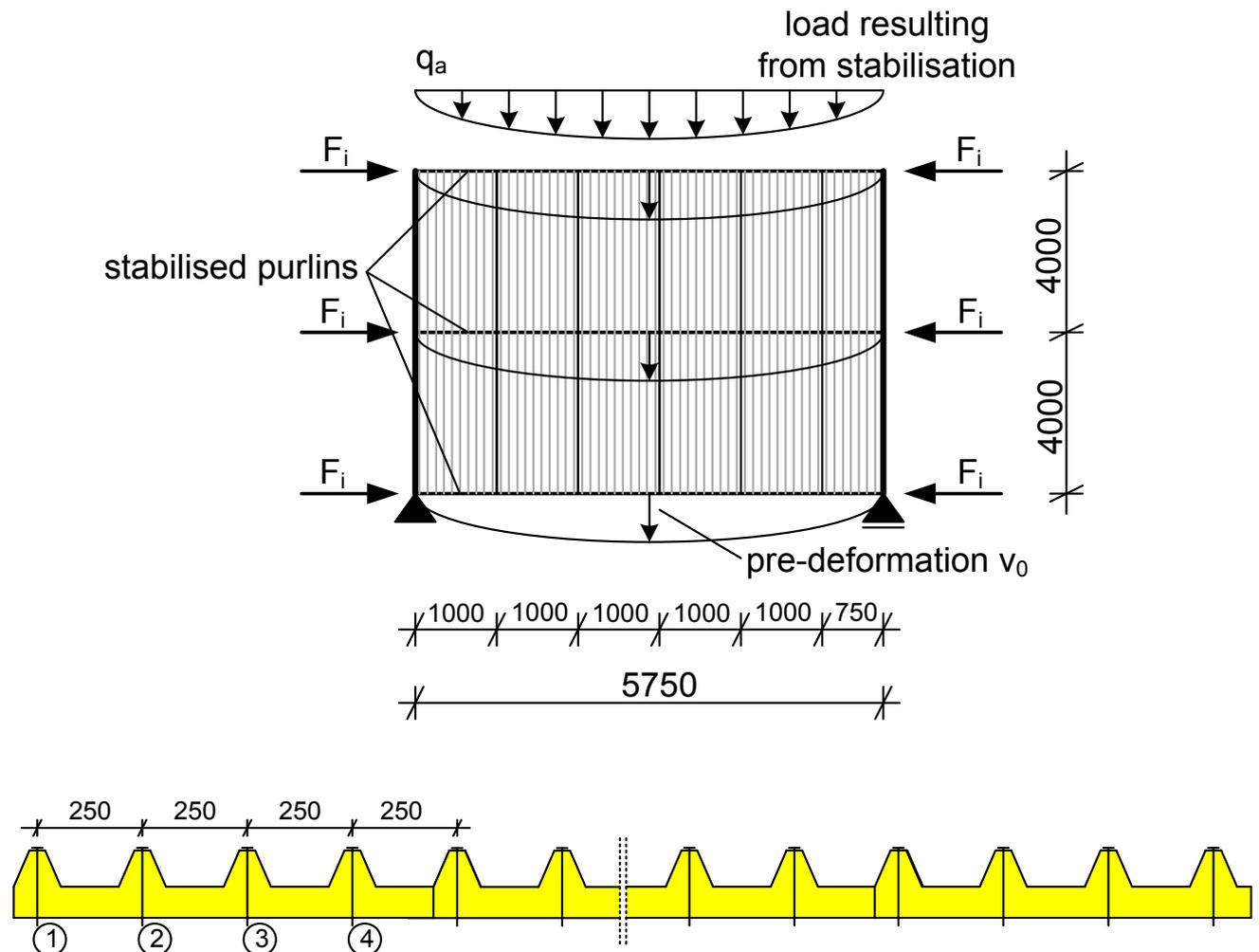
The fastenings at the transverse and at the longitudinal edges have the stiffness
