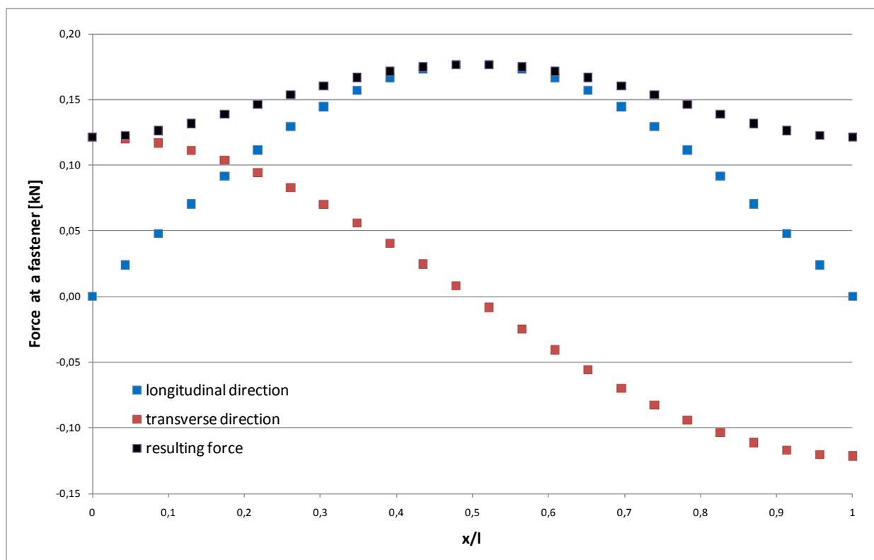
A further simplification is to calculate all forces with the width  $e = 250 \text{ mm}$ . For the fasteners at the corners of the diaphragm ( $x = 0$  and  $x = l$ ) the exact width is  $e/2$ . These fasteners are also loaded by the shear forces acting on the longitudinal edges. Also for this force the exact width is only  $e/2$ . These forces have to be added. But it is on the safe side to determine both forces with the width  $e$  and to design the fastening for the major of both forces.
