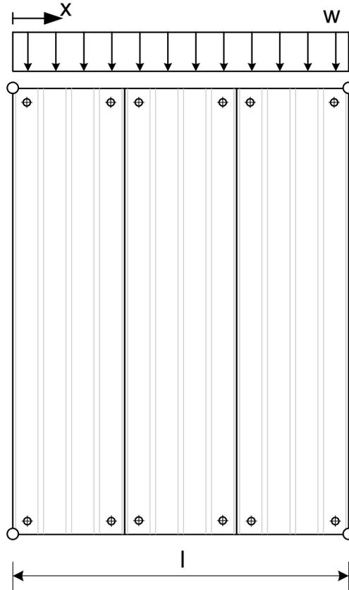
Fig. 8.5: Wind load acting in longitudinal direction of the panel
