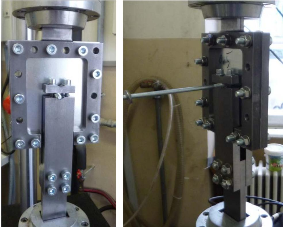
**Fig. 4.9: Test set-up of hole elongation tests**
