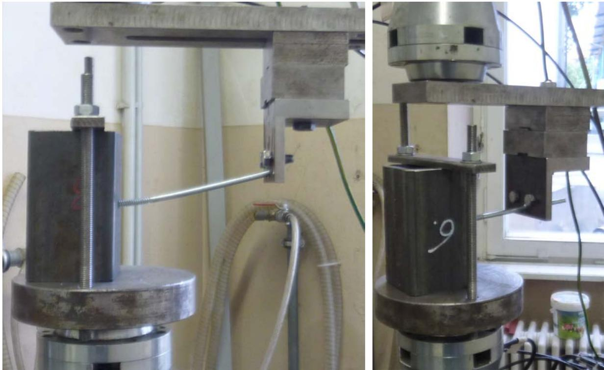
**Fig. 4.2: Test set-up of bending tests**
