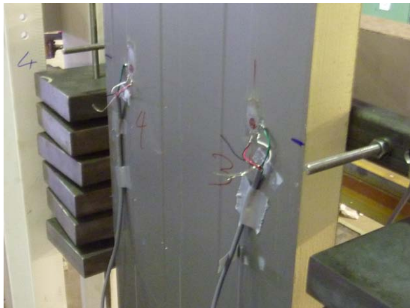
Fig. 7.8: Strain gauges at the face sheet subjected to tension
