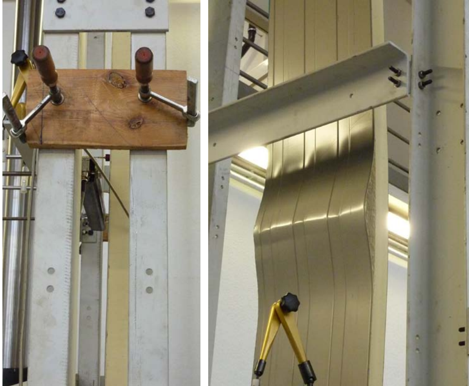
Fig. 4.7: Increasing of deflection and wrinkling at mid-span
