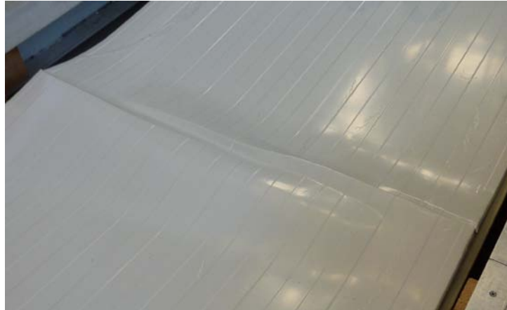
Fig. 2.2: Wrinkling of the compressed face sheet
