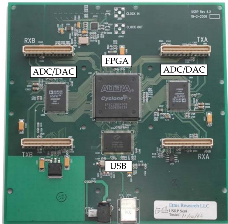
Figure 3.3: The USRP motherboard [54]
