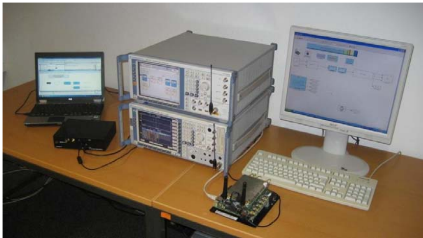
Figure 4.36: Measurement setup for the TETRA waveform testing
