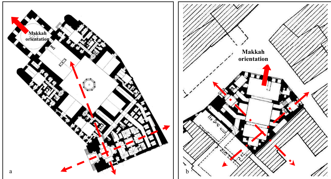
Figure 3-20: Deformed shape fits to two geometrical order (orientation order and orthogonal order) a- Madrasa of Sultan Hassan, b- Mosque of Amir Azbak al-Yusufi.
