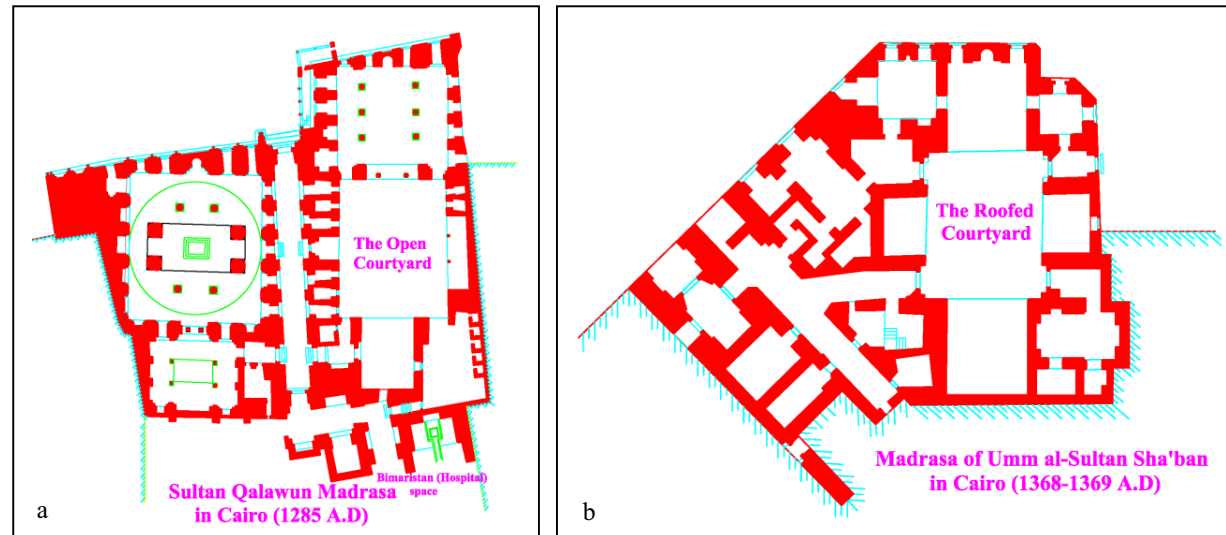
Figure 3-28: The two main prototypes of madrasa layout shapes a- Madrasa of Sultan Qalawun), b- Madrasa of Umm al-Sultan Sha'ban
