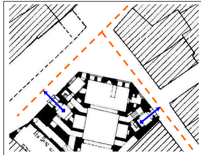
Figure 3-6: The street axis and the entrance axis and the perpendicular relation between them in the Mosque of Emir Azbak al-Yusufi.
