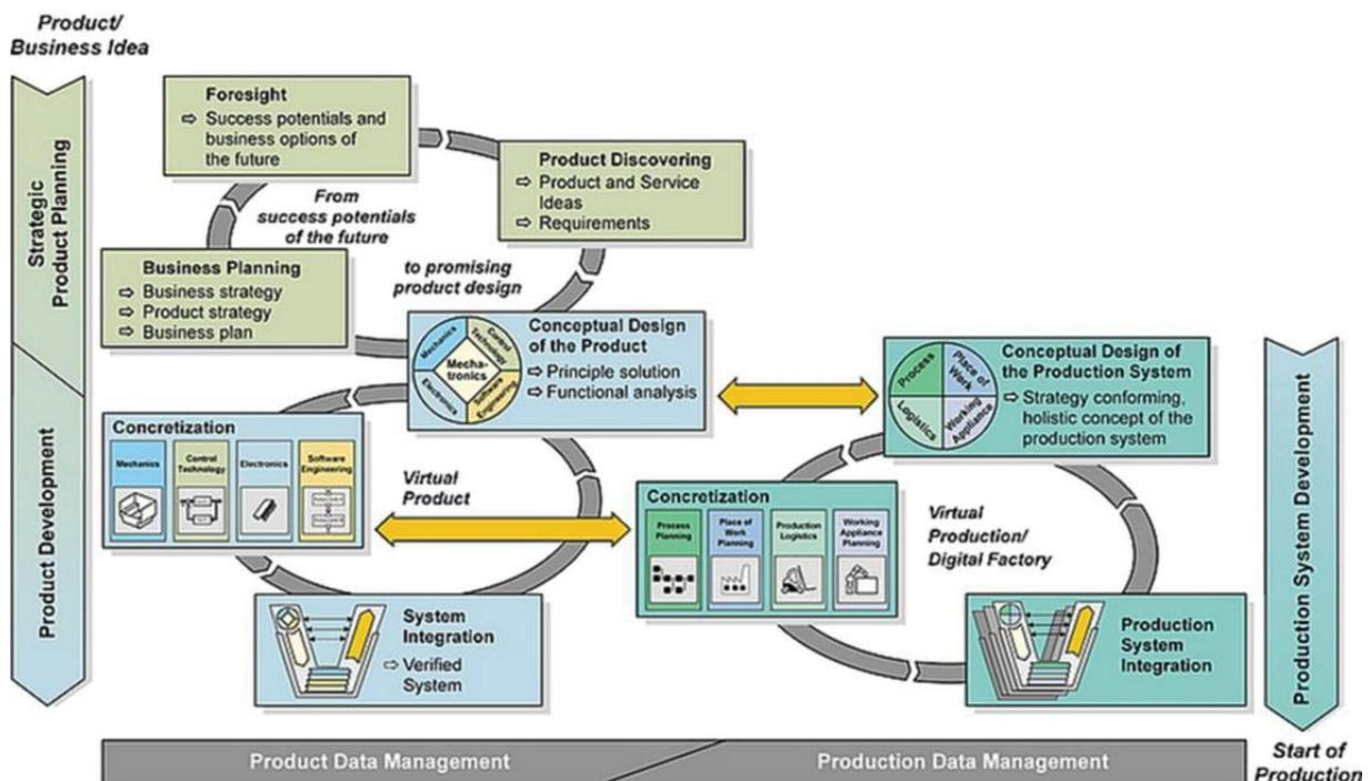
Figure 3-19: The three-cycle model<sup>326</sup>
