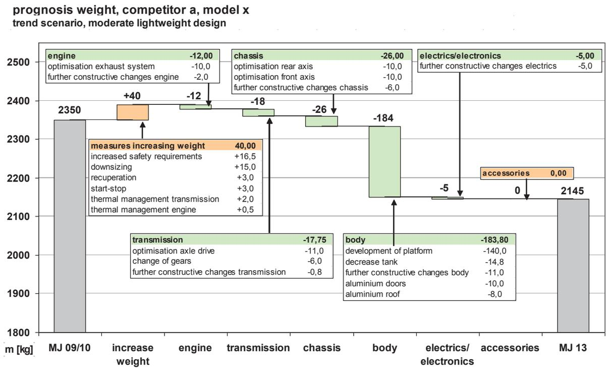
Figure 8-5: Prediction of future competitor car based on technological constraints
