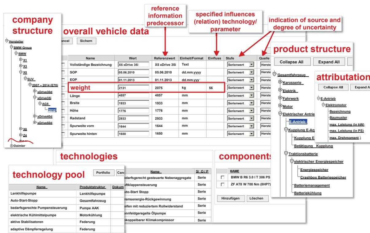
Figure 8-6: Data structures in the database<sup>425</sup>
