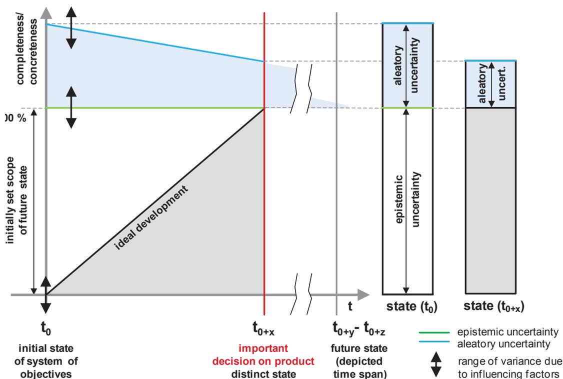
Figure 6-8: Overview of the initial scope for *concretisation* and *completion* of the system
