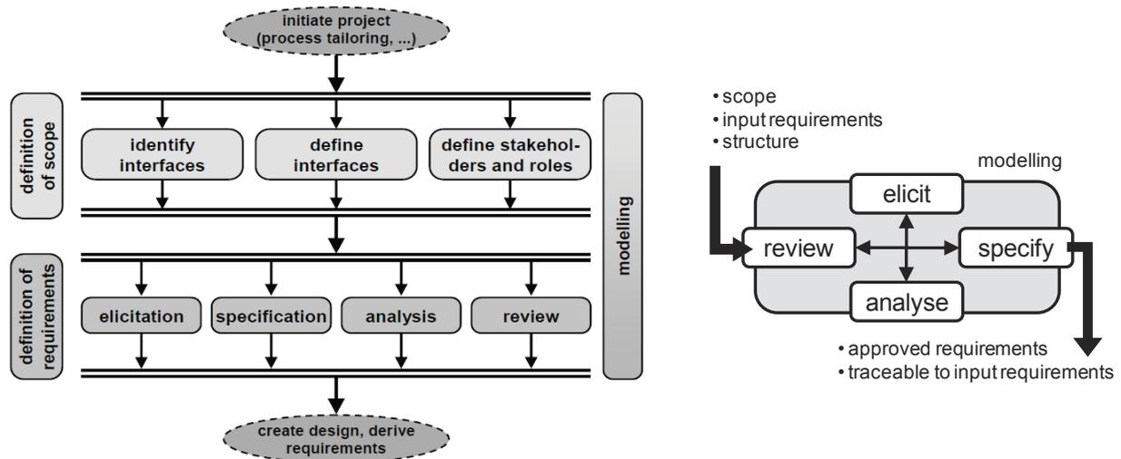
Figure 3-17: Process of requirements engineering<sup>317</sup>
