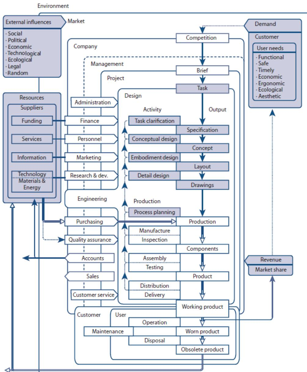
Figure 3-20: Engineering design process in project context<sup>329</sup>
