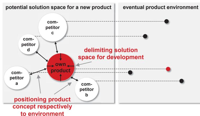
Figure 6-2: The two main functions of systems of objectives for product engineering
