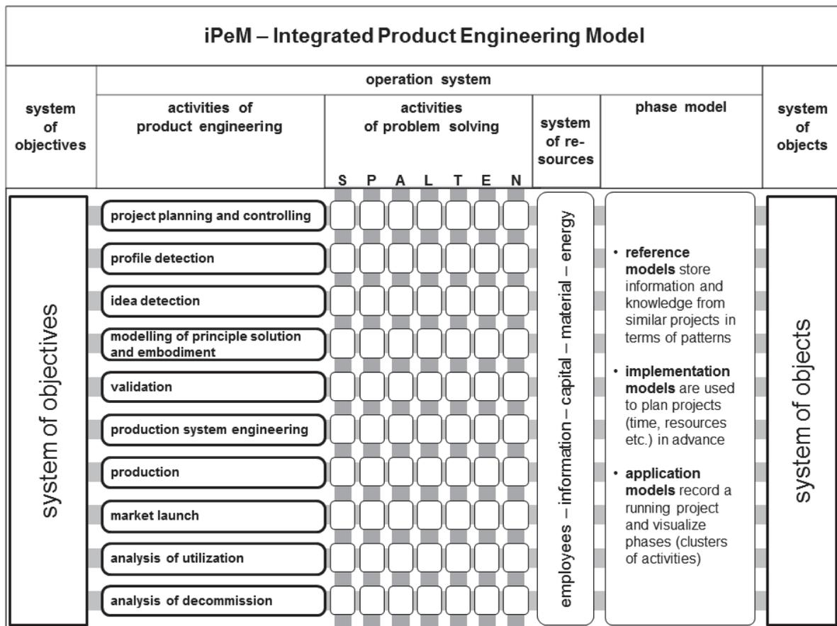
Figure 3-22: The Integrated Product Engineering Model (iPeM)<sup>332</sup>
