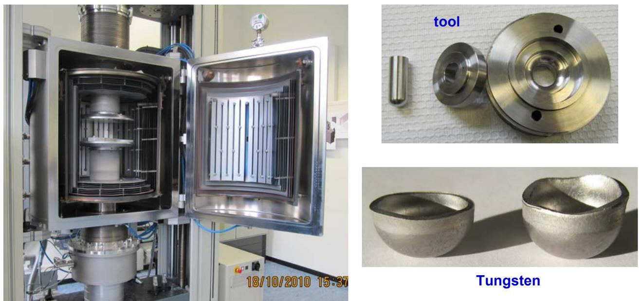
**Figure 4.3-3:** Successful deep-drawing tests with 1 mm W-sheet. Left: Vacuum furnace (courtesy V. Toth/KIT); Top right: newly developed tool made of tool steel; Bottom right: two deep-drawn W thimble-like caps ( $\text{Ø}15 \times 1$ ) of about 8 and 11 mm height, respectively.
