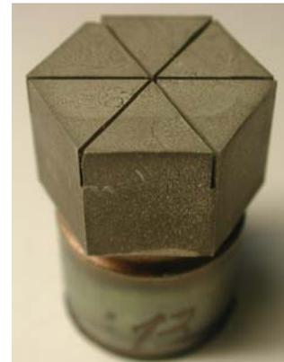
**Figure 3.9-15:** Second HHF test series, mock-up #13 (HEMJ, castellated).
