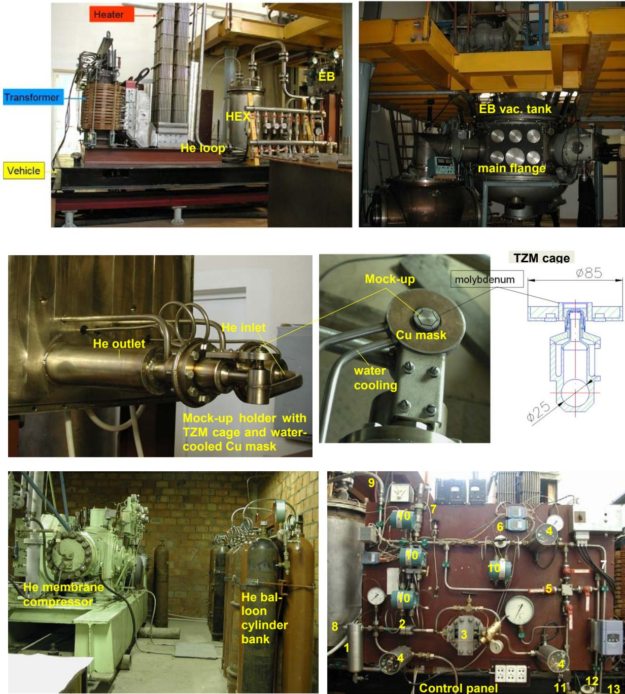
**Figure 3.9-2:** Built-in components of the helium loop and the TSEFEY vacuum tank.
