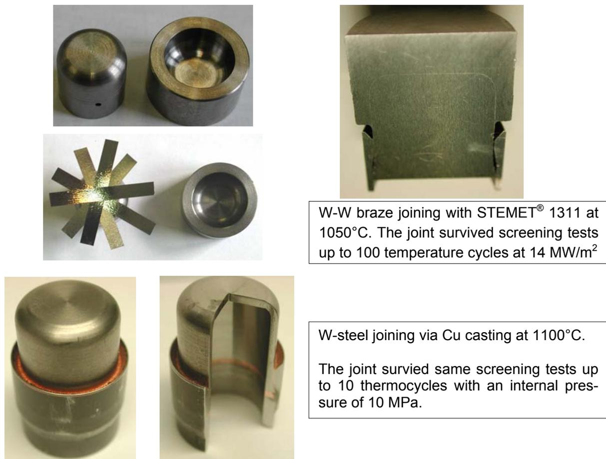
**Figure 3.9-5:** First successful attempts in joining of W parts with curvature (top) using a Ni-based filler metal STEMET<sup>®</sup> 1311 and W-steel parts with copper filler (bottom). Courtesy of Efremov.
