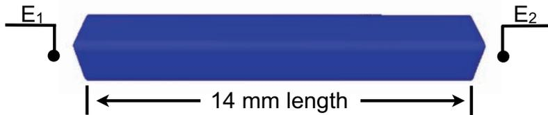
**Fig. 4.8.** The in-silico model of the parallelepiped (blue color) was 14 mm long and placed in a bath-medium with electrodes at either side to extract the extracellular potentials. The potential difference between the electrodes determined the course of the transmural ECG.
