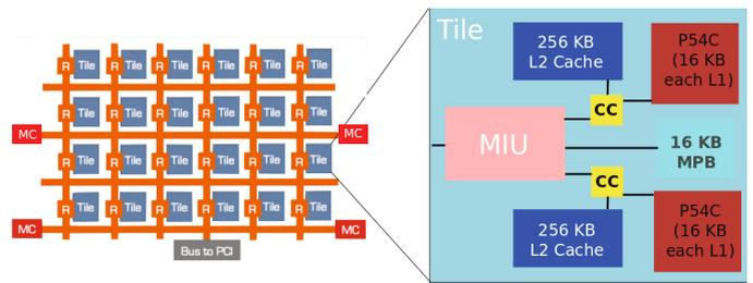
Fig. 1. Layout and tile architecture for the SCC
