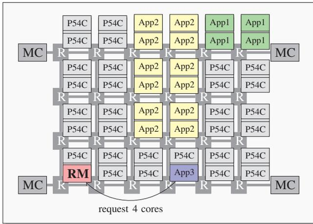
Fig. 2: Centralized resource management: Resource allocation/deallocation requests from applications are forwarded to and serviced by the Resource Manager (RM).
