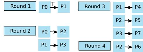
Fig. 5. Binary Tree broadcast running on 8 cores
