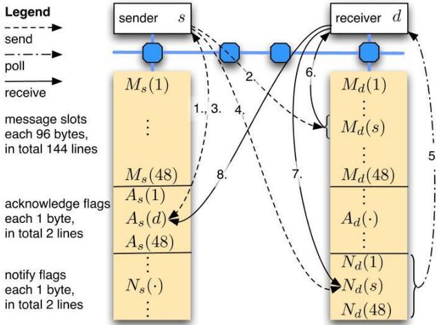
Fig. 5. Exchange of a one-way message over the SRAM.
