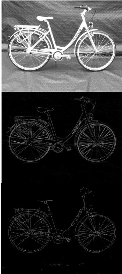
**Figure 1. a) input image, b) Sobel output, c) thinning output**
