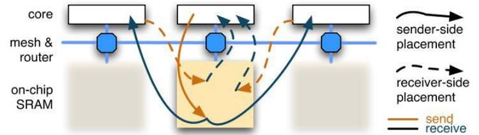
Fig. 4. Message placement on receiver vs. sender side.
