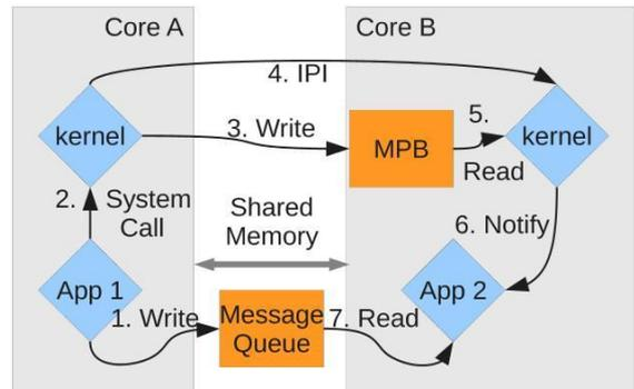
Fig. 1. Sending of a message between SCC cores
