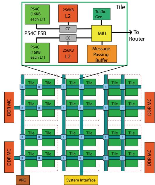
Fig. 2: SCC processor diagram
