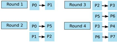
Fig. 7. Two Tree broadcast running on 8 cores
