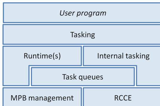
Fig. 1. A tasking environment for the SCC processor.
