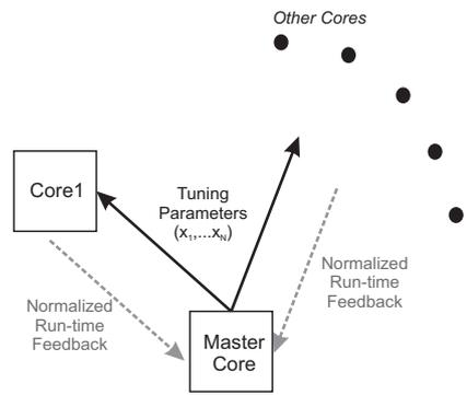
Fig. 1. Principles of homogeneous tuning on SCC cores.
