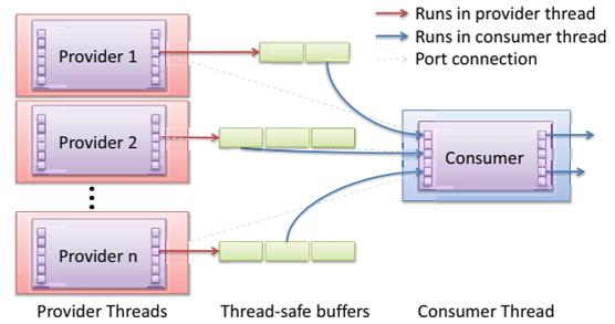
Fig. 3. Asynchronous data handover between two modules.
