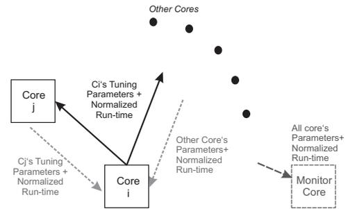
Fig. 2. Principles of heterogeneous tuning on SCC cores.
