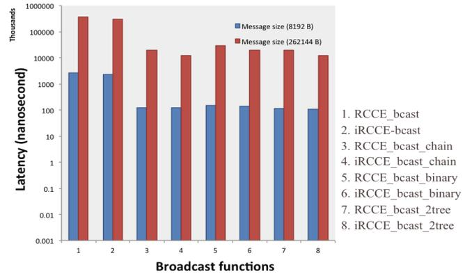
Fig. 12. Comparison RCCE broadcast algorithms performance on 48-cores
