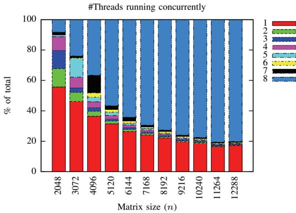
Fig. 2. Thread activity during the execution of the LU factorization with partial pivoting.
