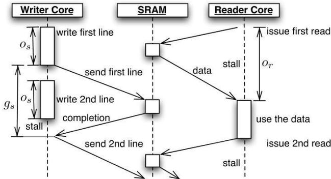
Fig. 2. Writing and reading over the mesh network.
