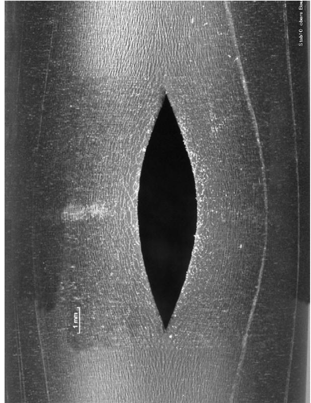
Rod #10 at 77°; p=45 bar,  $A_{burst}=13 \text{ mm}^2$
