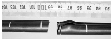
rod #5: rupture and crack at upper hydrogenated band
