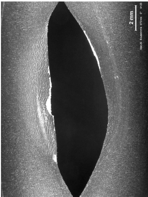
Rod #20 at 325°; p=50 bar,  $A_{burst}=53 \text{ mm}^2$
