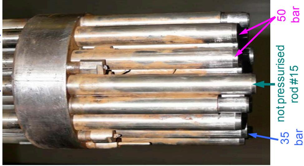
Fig. 46: QUENCH-L0; Consequences of ballooning.
