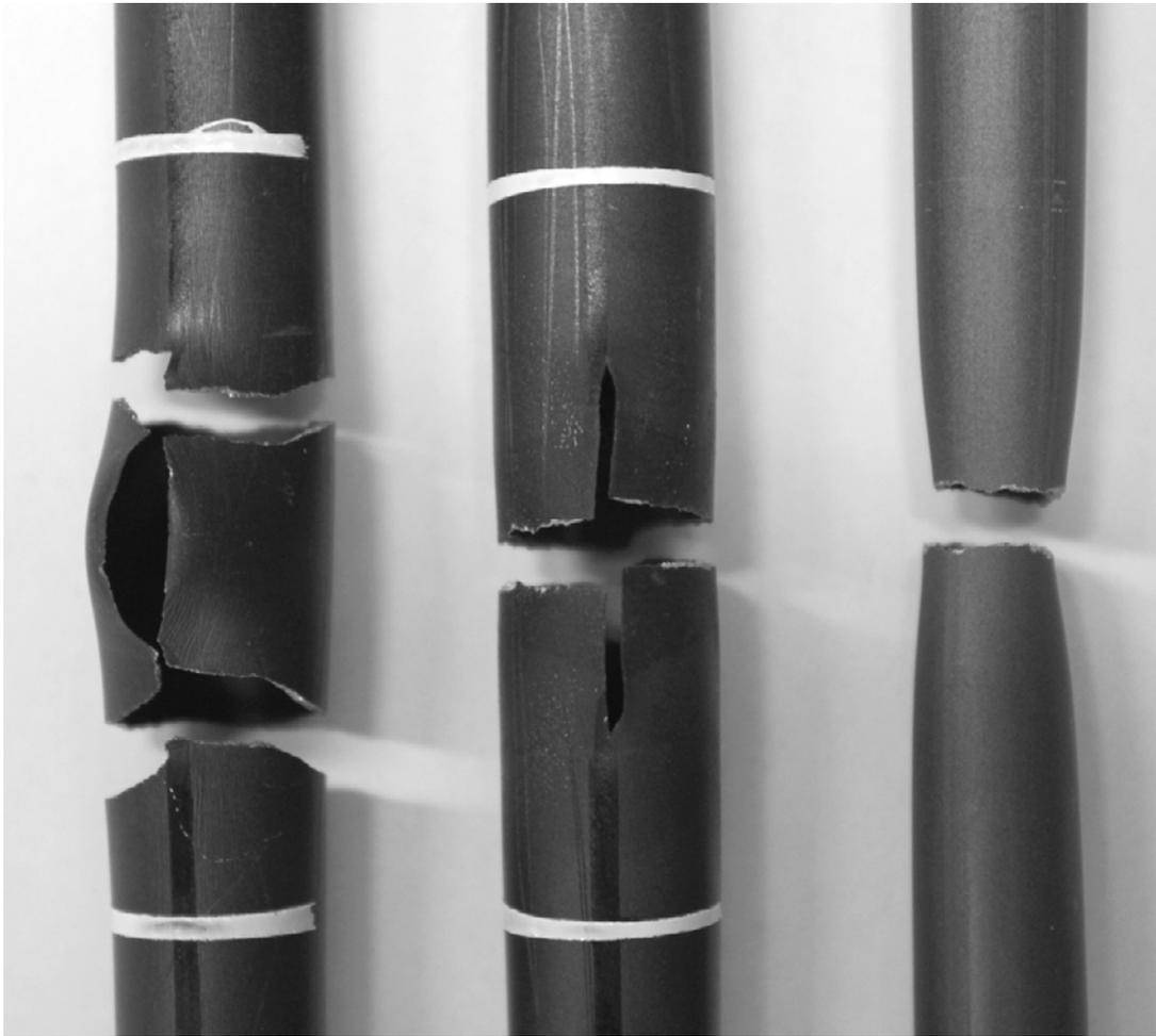
Two ruptures near to burst opening due to hydrogen embrittlement
