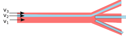
Fig. 2. Microfluidic switch controlled by the inflow speeds of the liquids.
