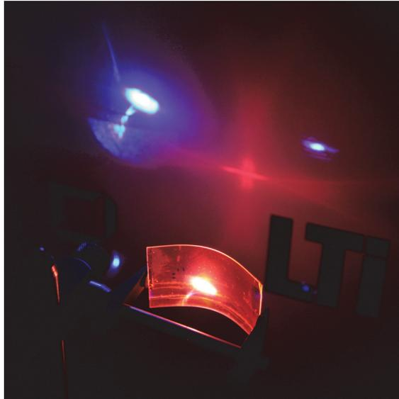
Figure 2.21: Photograph of an organic laser based on a two dimensional DFB resonator on a flexible polymer substrate and its output beam. The laser is on the foreground of the photograph. The beam can be seen as a red cross on the paper screen. The bright blue spots originate from scattered UV pump light which causes the paper to luminesce. (T. Woggon [65])
