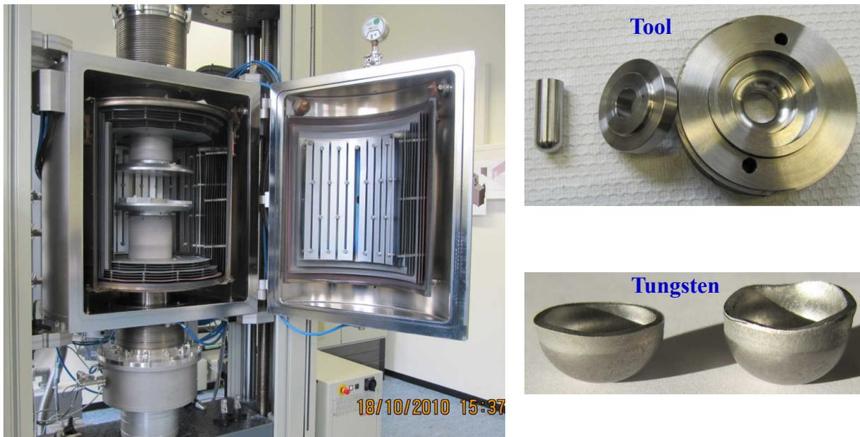
**Figure 4.3-3:** Successful deep-drawing tests with 1 mm W-sheet. Left: Vacuum furnace (courtesy V. Toth/KIT); Top right: newly developed tool made of tool steel; Bottom right: two deep-drawn W thimble-like caps ( $\text{\O}15 \times 1$ ) of about 8 and 11 mm height, respectively.
