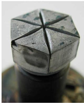
**Figure 3.9-29:** Third HHF test series, mock-up #32. Image after tests (10 cycles at  $q=10 \text{ MW/m}^2$ ).
