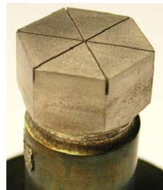
**Figure 3.9-17:** Second HHF test series, mock-up #18 (optimized HEMJ, castellated).
