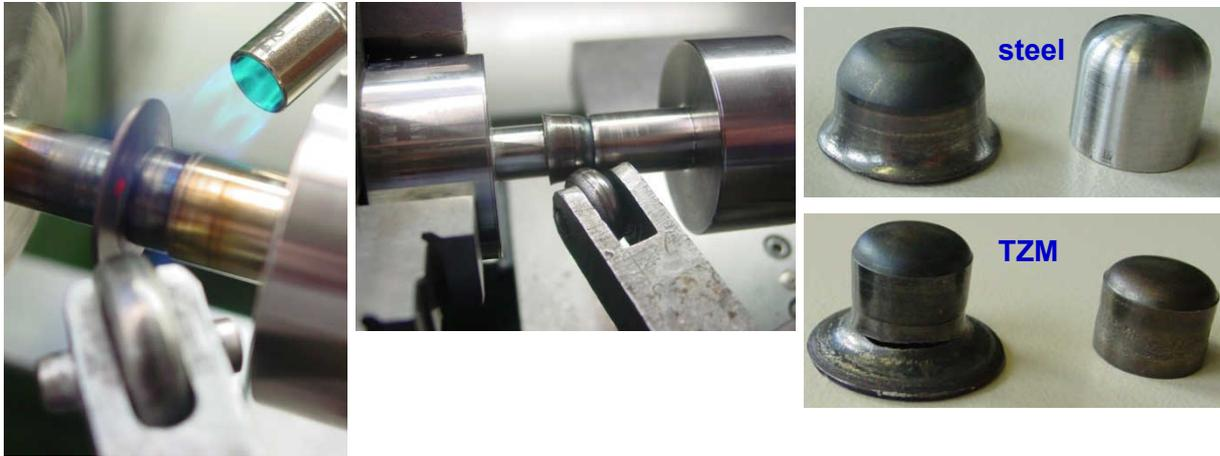
**Figure 4.3-2:** Roll pressing attempt using butane gas heating (left), thimble cap from 1 mm sheet of steel and TZM (right) [4.1-2]. Image courtesy of J. Reiser.
