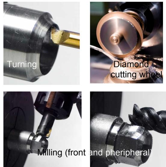
**Figure 4.1-2:** Machining methods for bulk tungsten tile.
