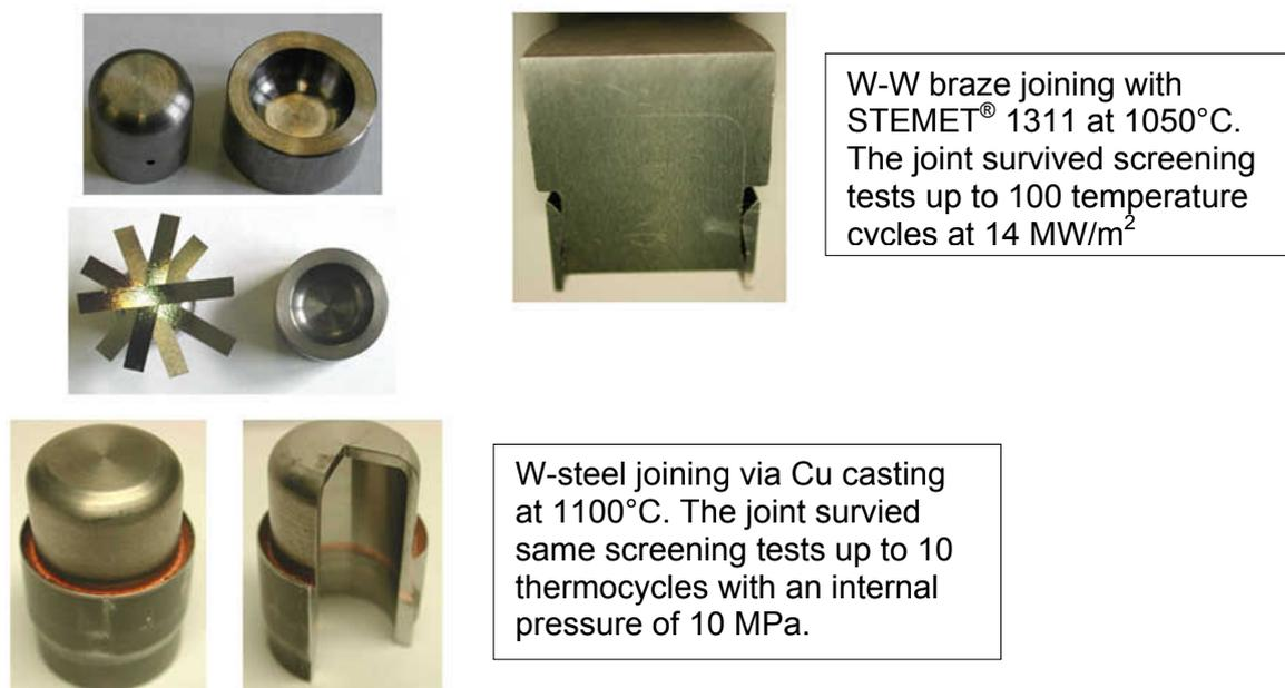
**Figure 3.9-5:** First successful attempts in joining of W parts with curvature (top) using a Ni-based filler metal STEMET<sup>®</sup> 1311 and W-steel parts with copper filler (bottom). Courtesy of Efremov.
