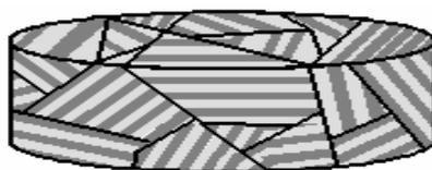
*Fig. 21 Schematic representation of a diblock copolymer sample with locally anisotropic ordered grains, which randomly orientate in the whole sample. The grain sizes are on the submicrometer scale.*
