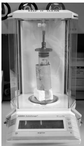
(b) Weighing syringe with sampled mother solution using a sample holder; Here the determination of mass of solution sampled is more accurate than using the mass difference of the beaker for dilution before and after sampling.
