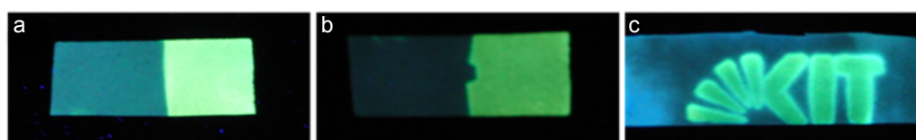
Figure 5.15: Photographs of pieces of cellulose under irradiation of light (366 nm) after the NITEC coupling, on their right-hand half in ethanol solutions containing maleimide functionalized PDMAEMA 3 (a), quaternized maleimide functionalized PDMAEMA 4 (b) and using a hand-made aluminum foil KIT mask in an ethanol solution containing maleimide functionalized pMMA 2 (c).
