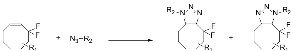
Figure 4.2: Overall reaction scheme of 1,3-cycloaddition incorporating ring-strained and fluorinated alkynes.
