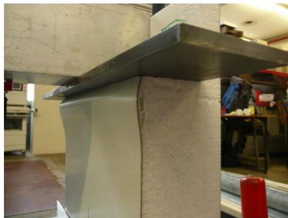
Fig. 4.1: Crippling at load application area
