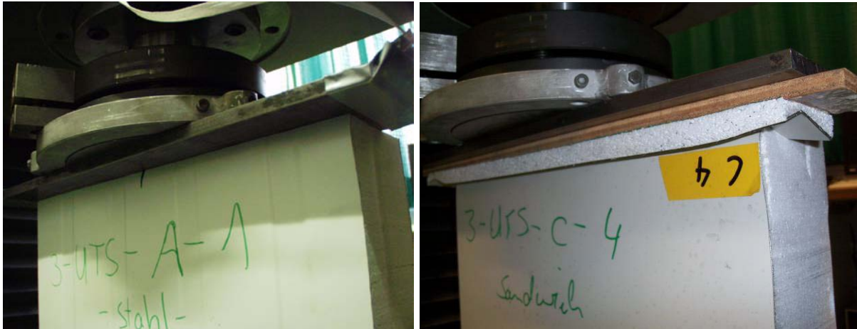
Fig. 3.5: Introduction of load by plate of steel and by sandwich panel
