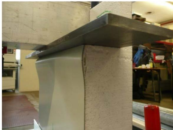
**Fig. 3.8: Crippling of the face at load application area**
