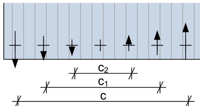
**Fig. 9.17: Longitudinal forces resulting from a moment**
