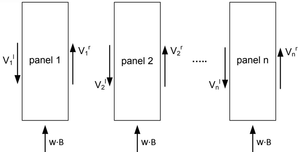
**Fig. 9.11: Forces acting in longitudinal direction of the panels**
