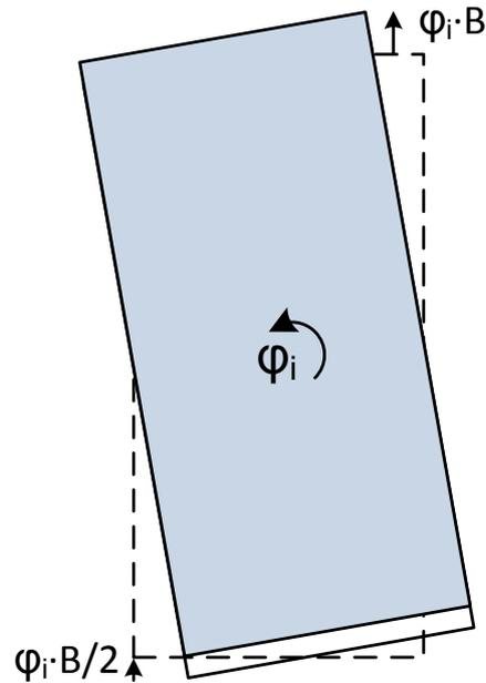
**Fig. 9.15: Displacements of panels resulting from rotation**
