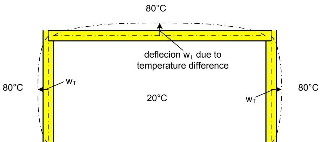
**Fig. 4.3: Temperature differences**
