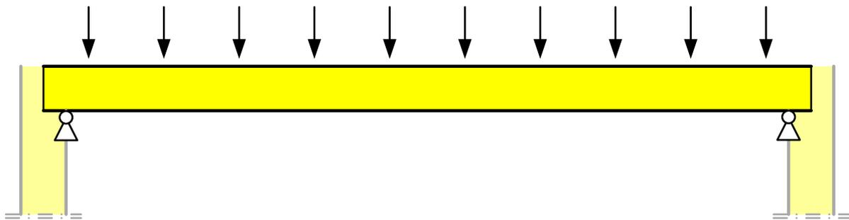
**Fig. 6.1:** Static system of roof panels
