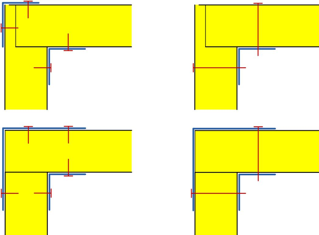
**Fig. 2.2: Possible versions of connections between wall and roof**
