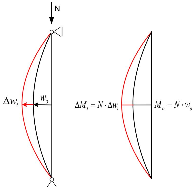
**Fig. 3.6: Creeping of axially loaded panels**
