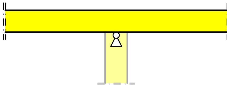
**Fig. 6.2:** Support of a roof panel by an interior wall
