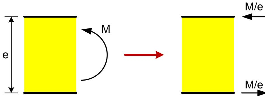
**Fig. 3.2:** Load bearing behaviour of panels subjected a bending moment
