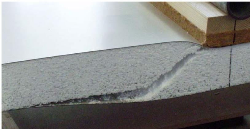
**Fig. 3.5:** Shear failure of the core
