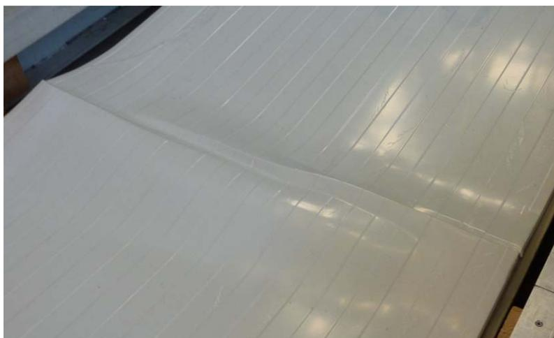
**Fig. 3.3:** Wrinkling of the compressed face sheet
