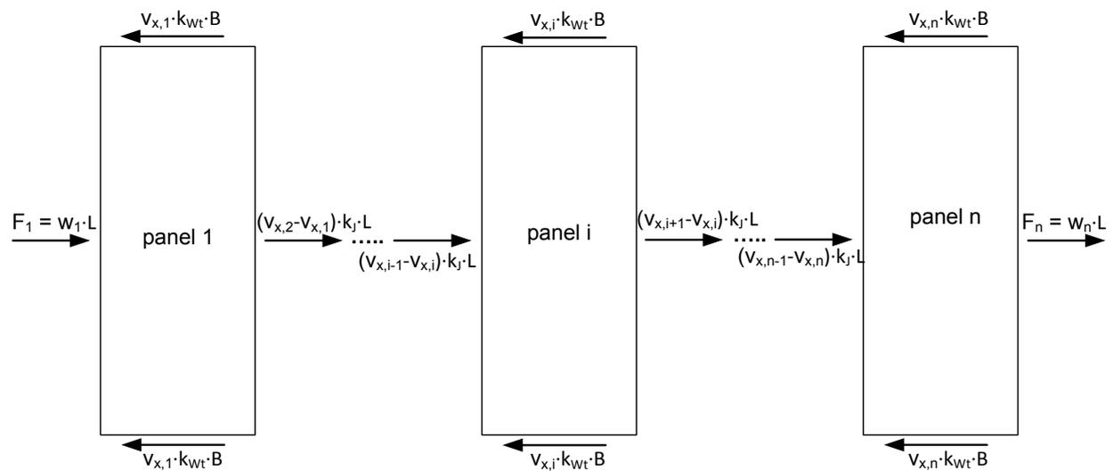
Fig. 9.10: Forces acting on the panels of a roof
