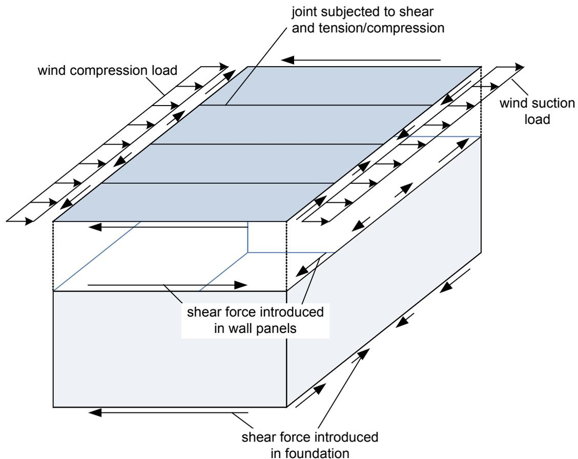
**Fig. 9.3: Transfer of loads through the roof**
