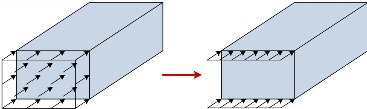
**Fig. 9.1: Introduction of horizontal loads into the roof**
