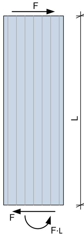
**Fig. 9.4: Transfer of in-plane shear loads through a wall panel**
