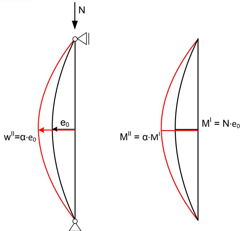
**Fig. 3.7:** 2<sup>nd</sup> order effects for a panel with initial deflection and axial load
