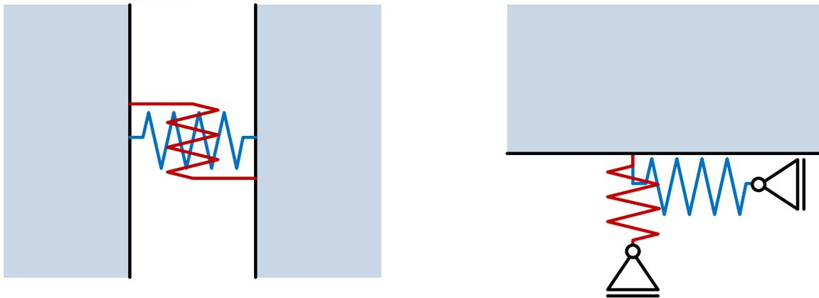
**Fig. 9.6:** Connection of joint and connection to foundation in the FE- model
