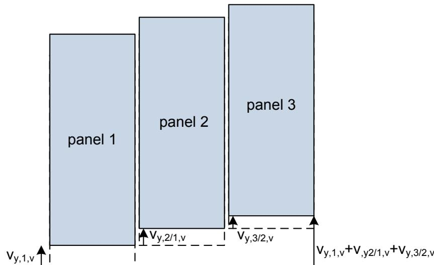
Fig. 9.14: Displacements of panels resulting from forces acting in longitudinal direction
