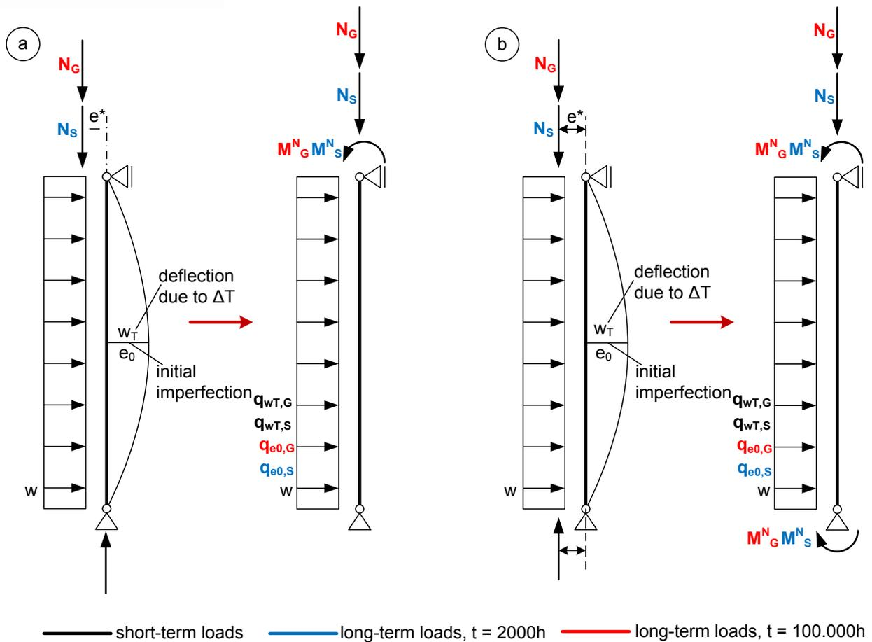
**Fig. 7.4:** Loads on wall panels
