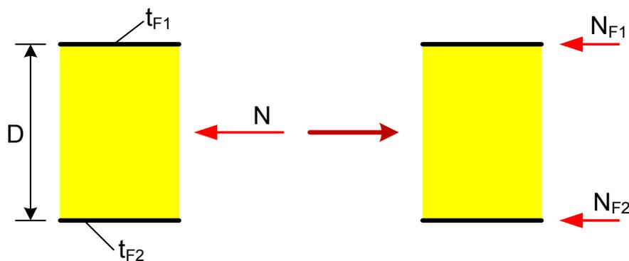
**Fig. 3.1:** Load bearing behaviour of panels subjected to an axial force
