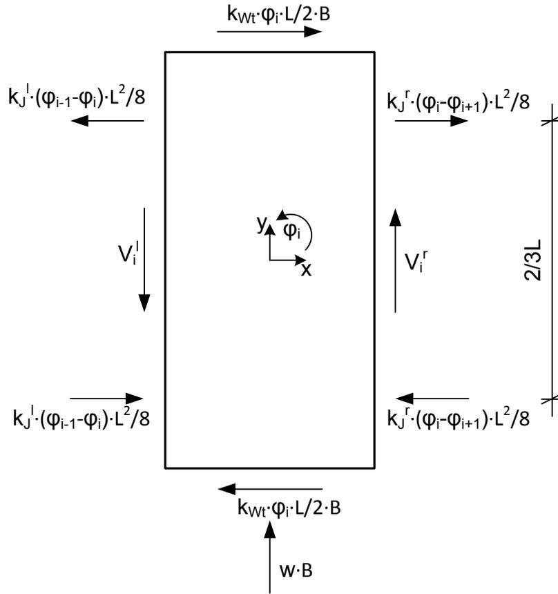
Fig. 9.13: Resulting forces of panel i
