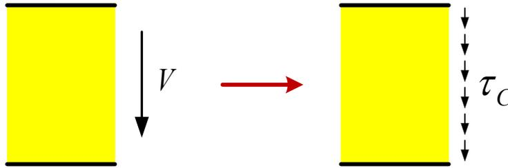
**Fig. 3.4:** Load bearing behaviour of panels subjected to a transverse force
