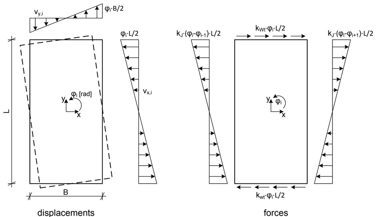
**Fig. 9.12: Displacements and transverse forces caused by rotation  $\varphi_i$**
