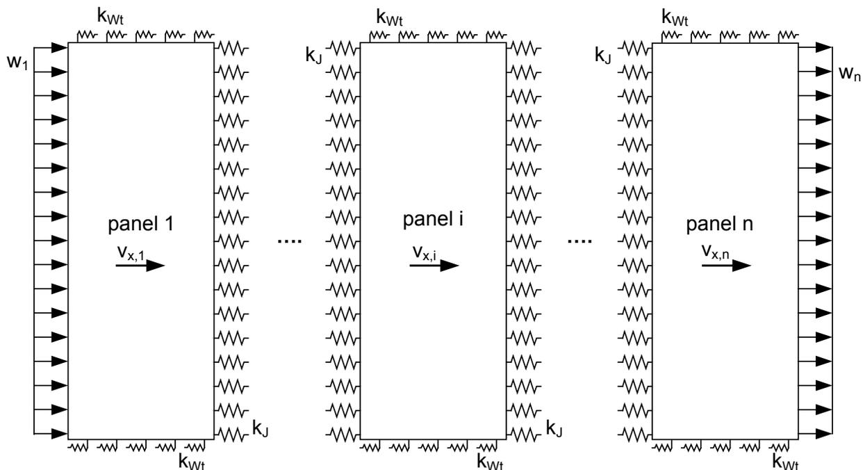
Fig. 9.9: Model of a roof for analytical calculation
