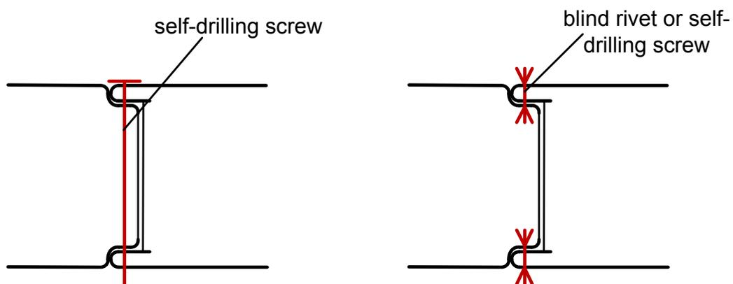
**Fig. 2.4: Connections of longitudinal joints**
