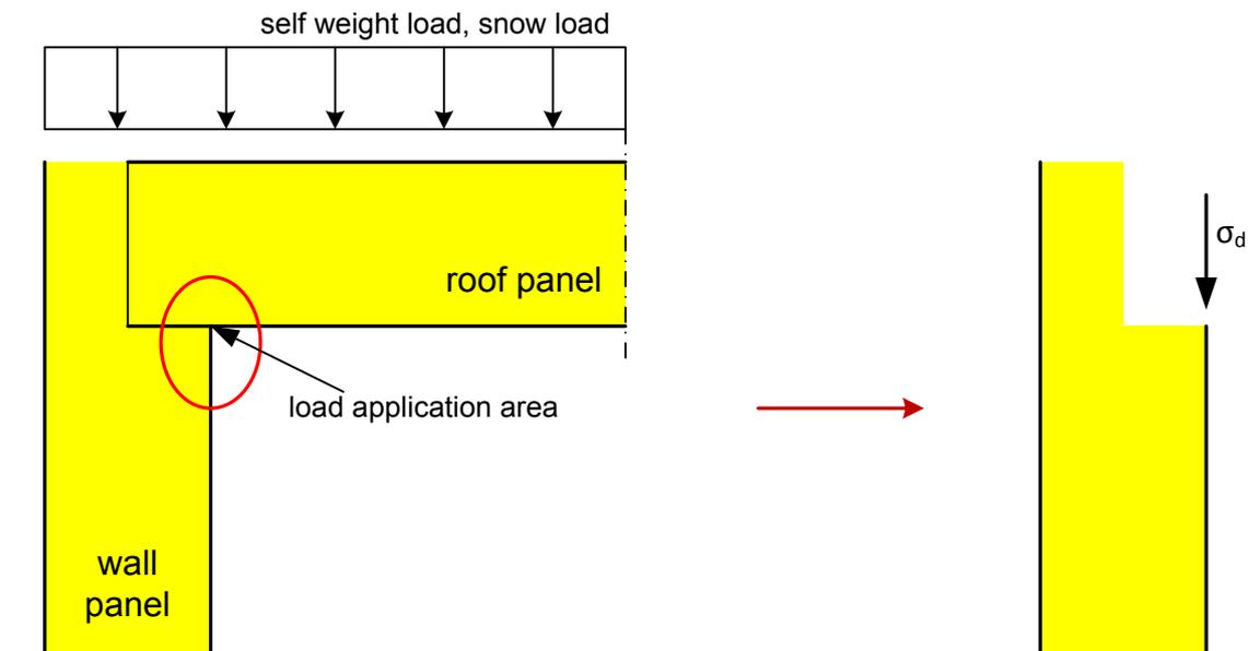
**Fig. 8.2: Normal stress introduced into the wall panel**
