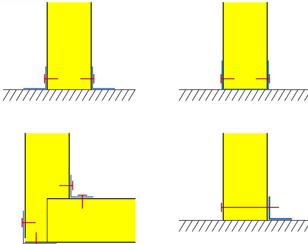
**Fig. 2.3: Possible versions of connections between wall and foundation**
