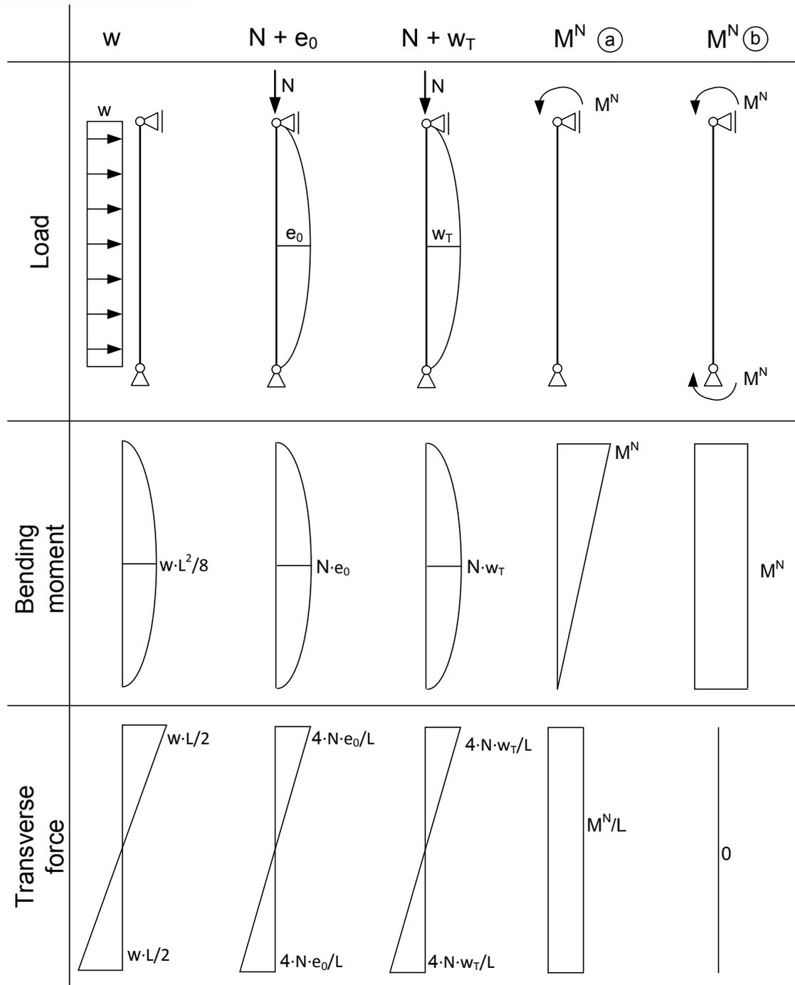
Fig. 7.5: Distribution of moment and transverse force (1<sup>st</sup> order theory, without creeping)
