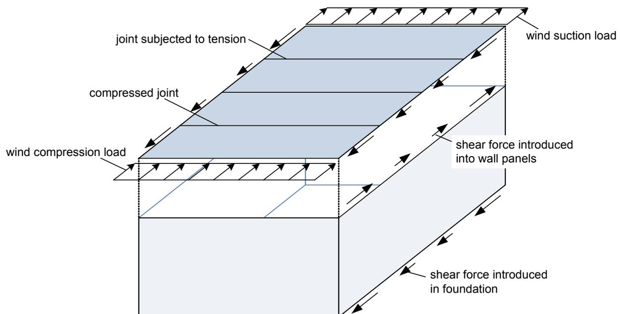
**Fig. 9.2: Transfer of loads through the roof**
