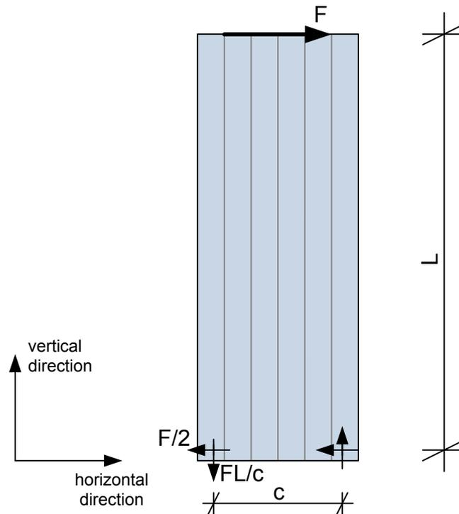
**Fig. 9.16: Forces at an in-plane shear loaded wall panel**
