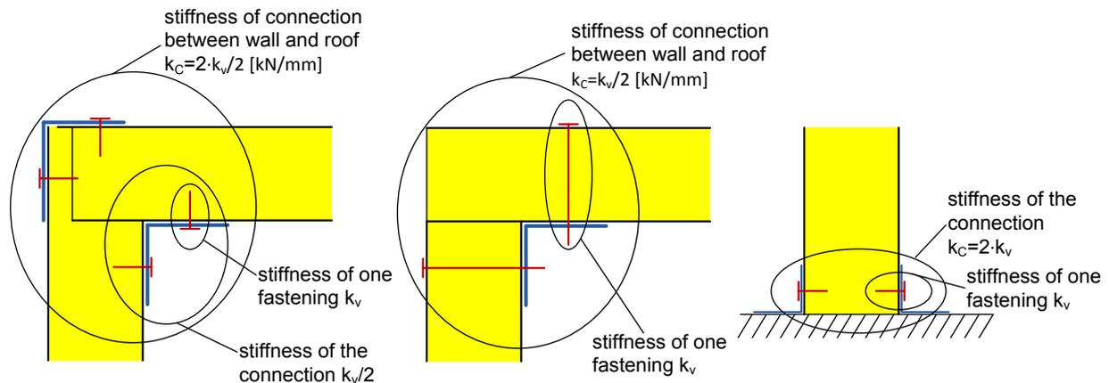
**Fig. 9.5: Determination of stiffness of connections**
