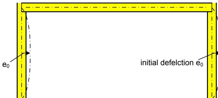
**Fig. 4.4:** Initial deflection of wall panels
