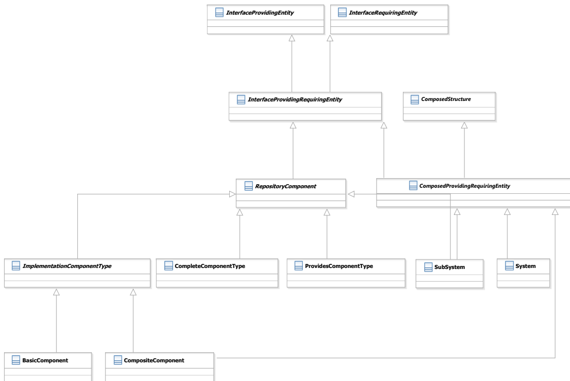
Figure A.4.: PCM Core Entity Overview
