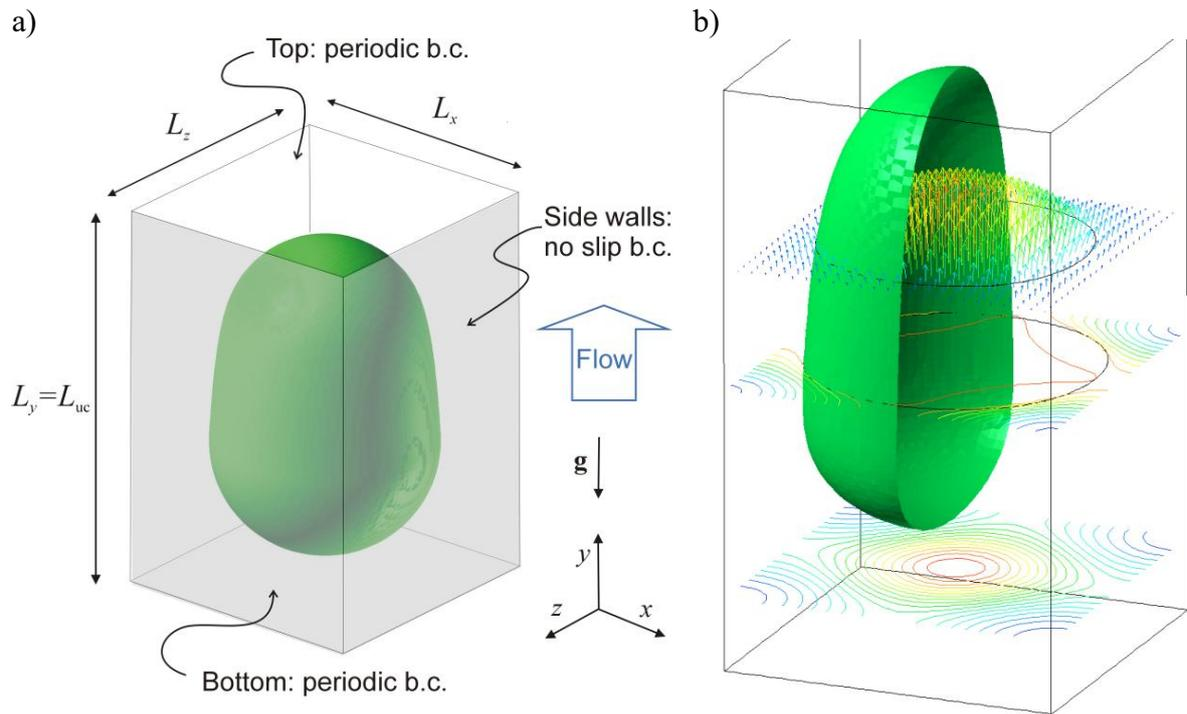
Fig. 1: a) Sketch of computational domain and coordinate system. b) Visualization of computed bubble shape (only half of the bubble is displayed). Also shown are the local velocity field (vectors) and the concentration field (contour lines) of a chemical species (which is transferred from the gas into the liquid phase) in different axial cross-sections
