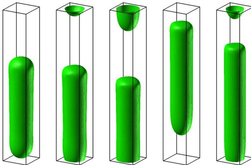
Fig. 2: Perspective view of computed steady bubble shape for  $L_{uc} = 6$  mm for five different values of the capillary number. From left to right, the values of  $(Ca; Re)$  are  $(0.045; 1.22)$ ,  $(0.117; 3.19)$ ,  $(0.17; 4.64)$ ,  $(0.25; 6.81)$ ,  $(0.491; 13.4)$ . The solid lines indicate the size of the computational domain. For further details about the simulations we refer to [4,7]
