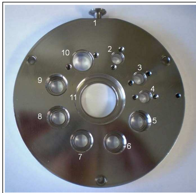
Figure 7: Reactor lid of Minifors bioreactor with numbered connections (see also table 7).
