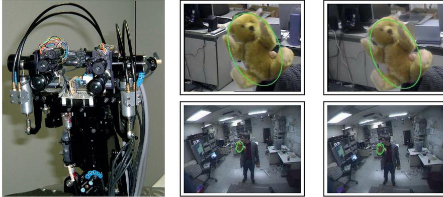
**Fig. 3.4.** Left: The humanoid platform DB offers an active head with foveated vision implemented using two cameras per eye. Right: The active visual search approach proposed in [Ude et al., 2003] actively tracks the target object in the peripheral image to perform recognition in the detailed foveal view. Reprinted from [Ude et al., 2003] ©2003 IEEE.
