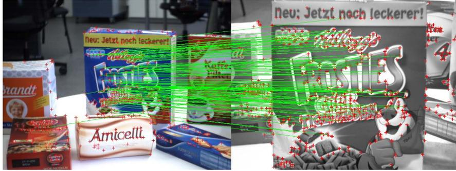
**Fig. 5.15.** Purged correspondences after applying the Hough transform to the matches. The illustrated matches correspond to the bin in Hough space with maximum vote.
