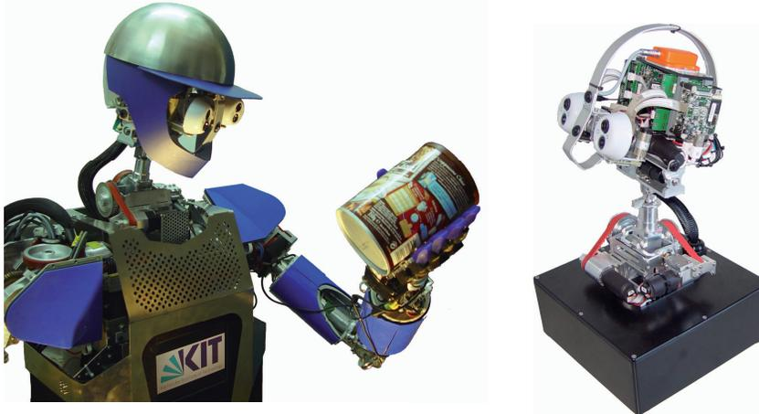
**Fig. 4.1.** Left: The target platform for this thesis is the humanoid robot platform ARMAR-III. Right: The active head of ARMAR-III is available as stand-alone version under the name Karlsruhe Humanoid Head. The head is equipped with a active foveated vision system actuated by 7 DoF.
