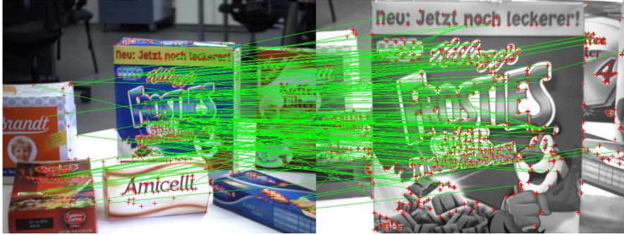
**Fig. 5.14.** Correspondences between object and scene resulting from matches of Harris-SIFT features using the Euclidean distance. The matching procedure generates several outliers.
