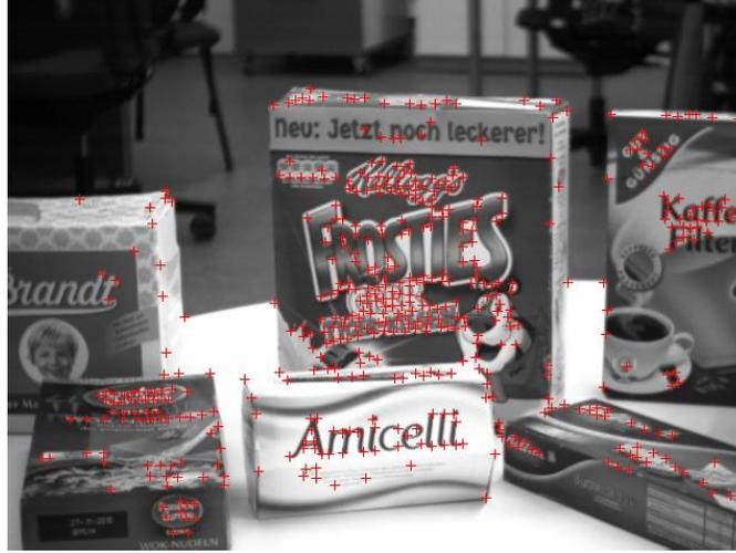
**Fig. 5.12.** Harris corner points extracted in the foveal camera image with a minimum cornerness of  $C_{min} = 0.001$ .
