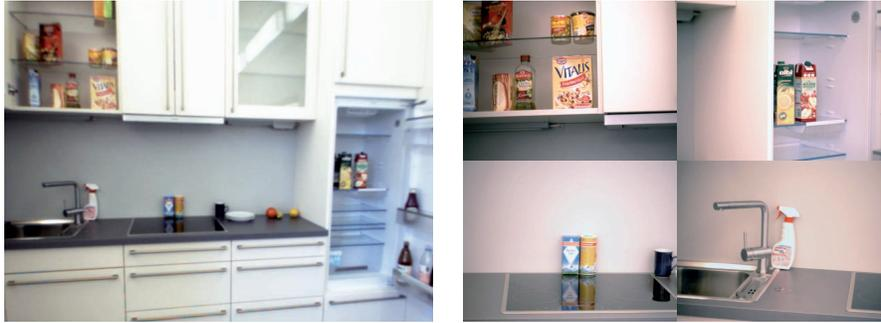
**Fig. 1.2.** The humanoid robot ARMAR-III is equipped with a peripheral-foveal camera system which mimics the high resolution fovea of the human eye. Left: The peripheral views provide an overview of the scene. Right: Using foveal vision the detailed views of the scene are perceived within several glances by actively moving the eyes. The inner model of the scene is derived by considering a sequence of such foveal views at different gaze directions.
