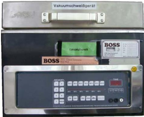
Figure 3.29: Vacuum device, which is used to evacuate the detector package.
