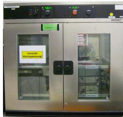
Figure 3.30: Heating cabinet, which is used to maintain a constant temperature while an oscillating high voltage is applied.
