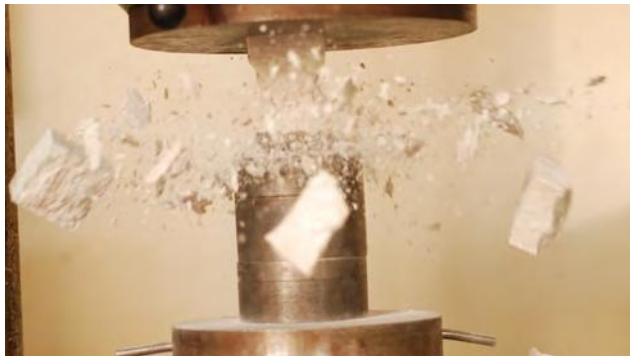
Fig. 8 Failure of high strength concrete (Photo by Salem G. Nehme)
