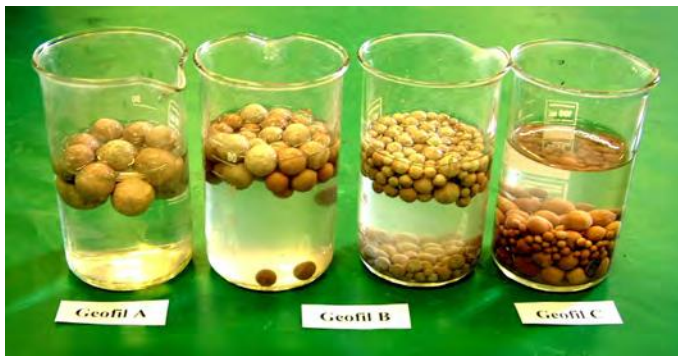
Fig. 6 Lightweight aggregates (Geofil) (photo by Zsuzsanne Józsa)
