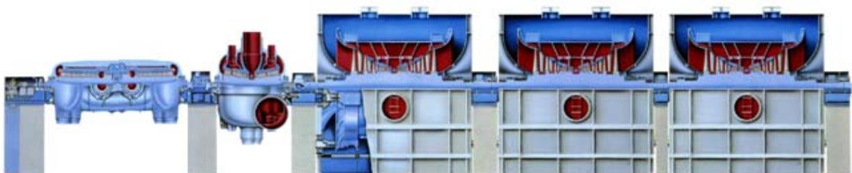
Fig. 5.4: Turbine design concept with double flow HP, IP and 3 LP turbines [12]
