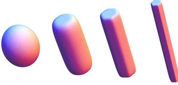
Figure 2.2: Contour of the anisotropic norm \ell^p(\mathbf{x}) = 1 with increasing exponents p = \{2, 5, 10, 20\} and aspect ratios: The angularity of the grain models increases with increasing values for the exponent p . Natural shapes are obtained by high values, e.g., p = 10 \dots 20 and L/B = 3 \dots 10 . The left contour is an ellipse, i.e., a Euclidean norm for p = L/B = 2 .
