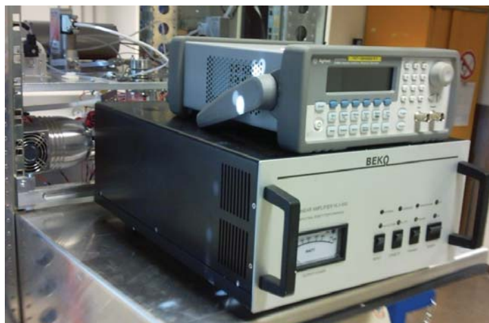
Figure 5.11: View of function generator (Agilent Technologies, USA, model 33220A) and signal amplifier (BEKO Elektronik, Germany).
