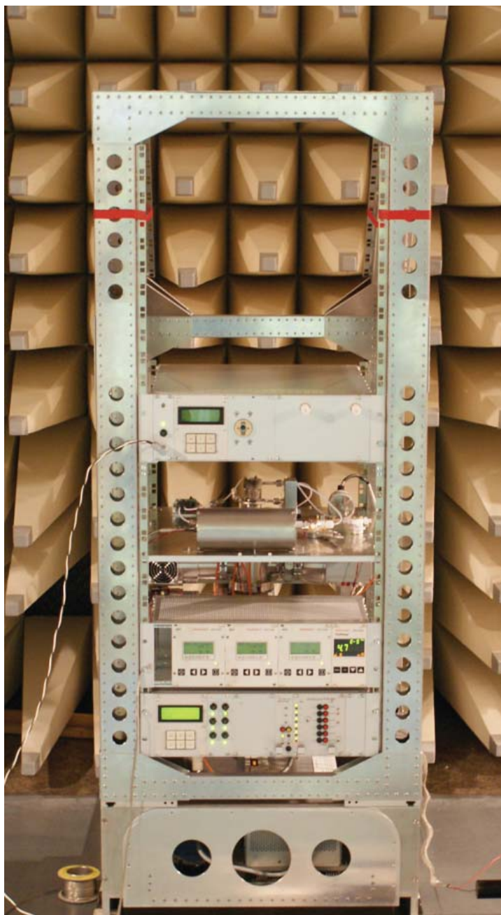
Figure 6.9: HALO rack with the PTR-IF-MS and the O 3 instrument. Picture taken during a electro-magnetic compatibility test.
