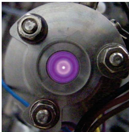
Figure 3.3: View through a quartz glass of the ion production plasma and its regions on a HCD ion source. Picture taken during ion source optimization.
