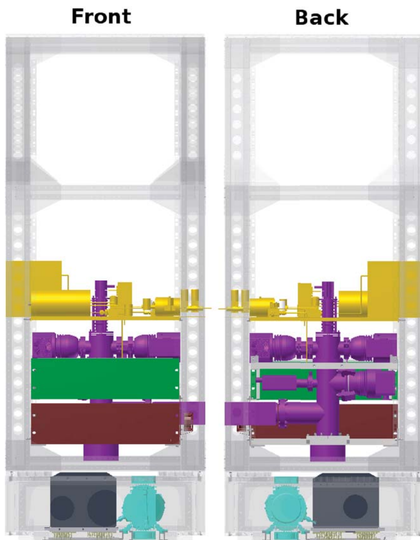
Figure 6.10: Black: radio frequency generator; cyan: diaphragm pump; brown & green: electronic module I & II; violet: MS-Analyser; yellow: flow control plate. For details see text.
