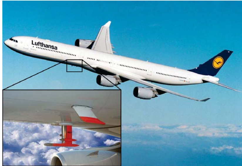
Figure 7.1: Lufthansa Airbus A340-600 and CARIBIC air inlet in closer view.
