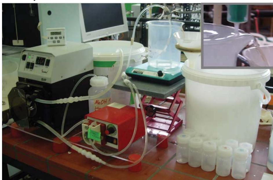
Figure 4.45: Experimental setup of the flow-through cell experiments
