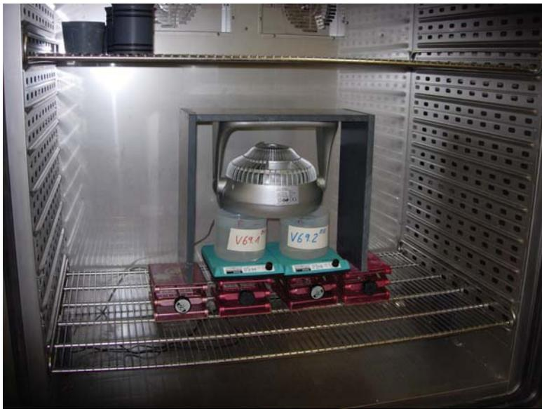
Figure 5.1: Experimental setup of the evaporation experiments in the climate chamber.
