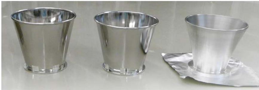
**Figure 5.4: Comparison of three electrode designs.** This photograph shows three different ground electrode designs. The electrode design had a huge impact on the background rate. The electrodes (from left to right) correspond to the measurement I-III described in this section. The corresponding simulation of Penning traps for the three geometries can be found in figure 5.8.
