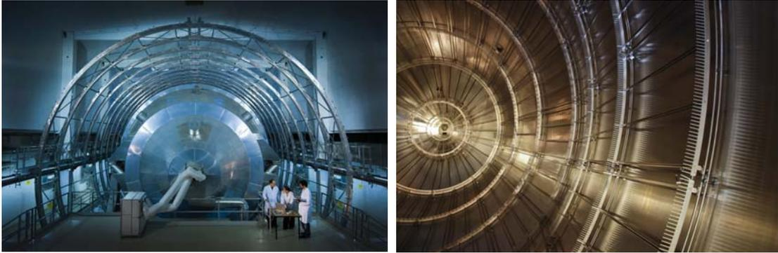
**Figure 2.8: Photograph of air coil system and wire electrode.** Left: The air coil system surrounds the main spectrometer vessel. Its purpose is to compensate the earth magnetic field and to fine tune the magnetic field inside the main spectrometer. Right: View into the main spectrometer. Its inner surface is covered with 24 000 wires of 200-300  $\mu\text{m}$  thickness, providing additional shielding against muon-induced background as well as fine tuning the electrostatic retarding voltage.
