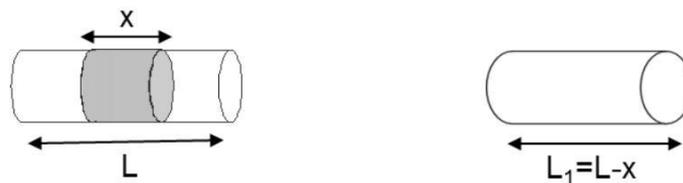
Figure 4-1: Schematic illustration of the experimental set-up for determination of the Bo Number. Left: Reactor tube (length L) with packed bed (length x). Right: Empty reactor tube (length L-x).
