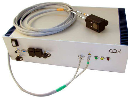
Figure 7.4: Final design of the sensor prototype developed within the BMBF project "CuringOnlineSensor". The sensor head is connected with optical fibres to the processing unit. Laser sources, InGaAs detector and power management are hosted inside this processing unit. The detector head only consists of fixed optical elements, thus suited for rough environments. (Photo courtesy of QIAGEN Lake Constance GmbH, Elmar Feuerbacher.)
