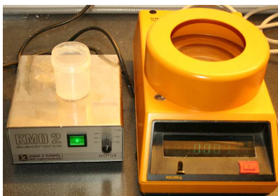
Figure 4.1: Laboratory equipment used for the preparation of the model formulation. Left: Magnetic stirrer; Right: precision scale;
