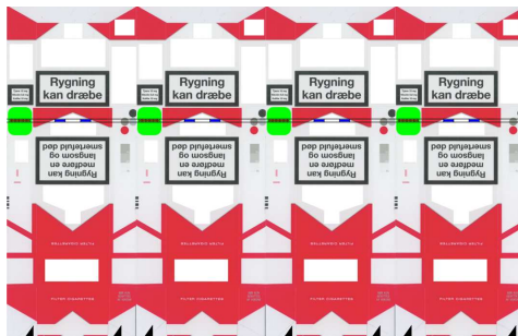
Figure 8.3: Example of the test measurement on the paper web. The laser line of the sensor is marked from left to right. The conversion measurement is performed on the green coloured test patterns. The blue areas are used for calibrating the sensor before each conversion measurement. The trigger marks of the printing machine, which are used for correct positioning of the sensor, are visible as black triangles at the bottom. A detailed view of the test pattern and the reference spots are shown in Figure 8.4.
