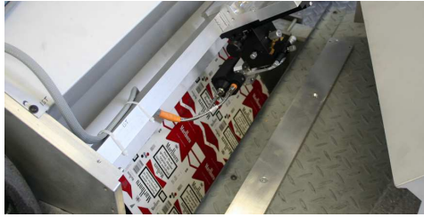
Figure 8.2: Integrated sensor head on the printing machine with a metal cover (right side) and installed optical fibre connection.
