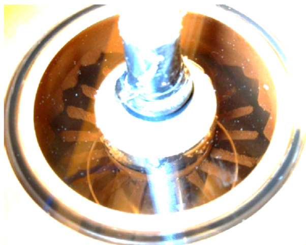
Figure 2: Deposit during the process in MEC in the first prototype; photo taken using a stroboscope; the rough surface of the particles on the wire is well visible;
